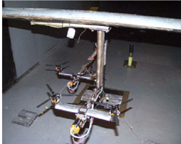
Figure 1. Tiltrotor models in the Army 7- by 10-Foot Wind Tunnel at NASA Ames Research Center.
