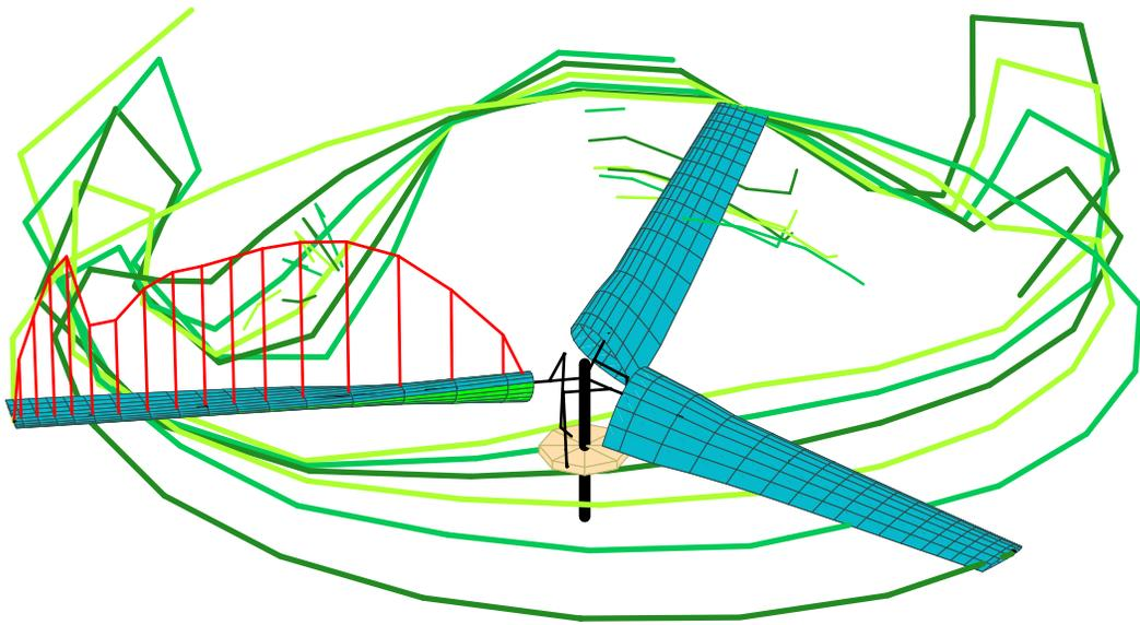
Figure 22a. Calculated TRAM wake geometry and loading for  $\mu = 0.15$ ,  $\alpha_s = -6$ ,  $C_T/\sigma = 0.128$ .
