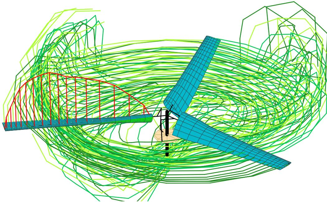
Figure 24a. Calculated TRAM wake geometry and loading for  $\mu = 0.15$ ,  $\alpha_s = -6$ ,  $C_T/\sigma = 0.128$ .
