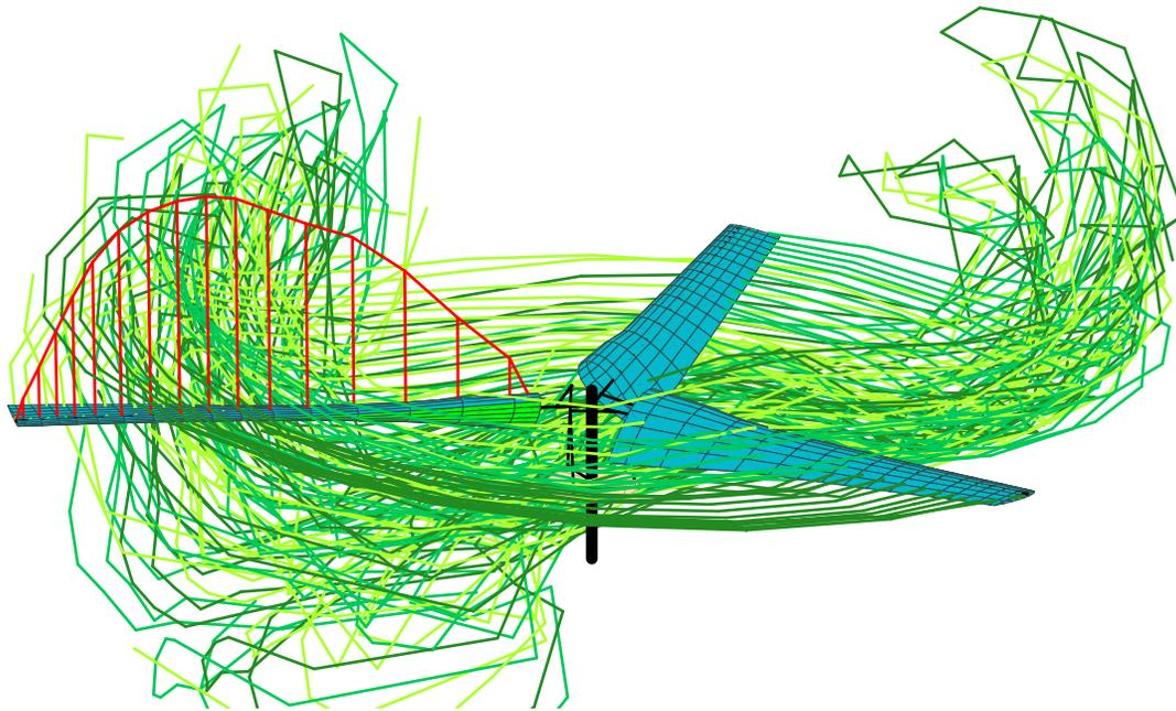
Figure 25a. Calculated TRAM wake geometry and loading for  $\mu = 0.15$ ,  $\alpha_s = 6$ ,  $C_T/\sigma = 0.128$ .
