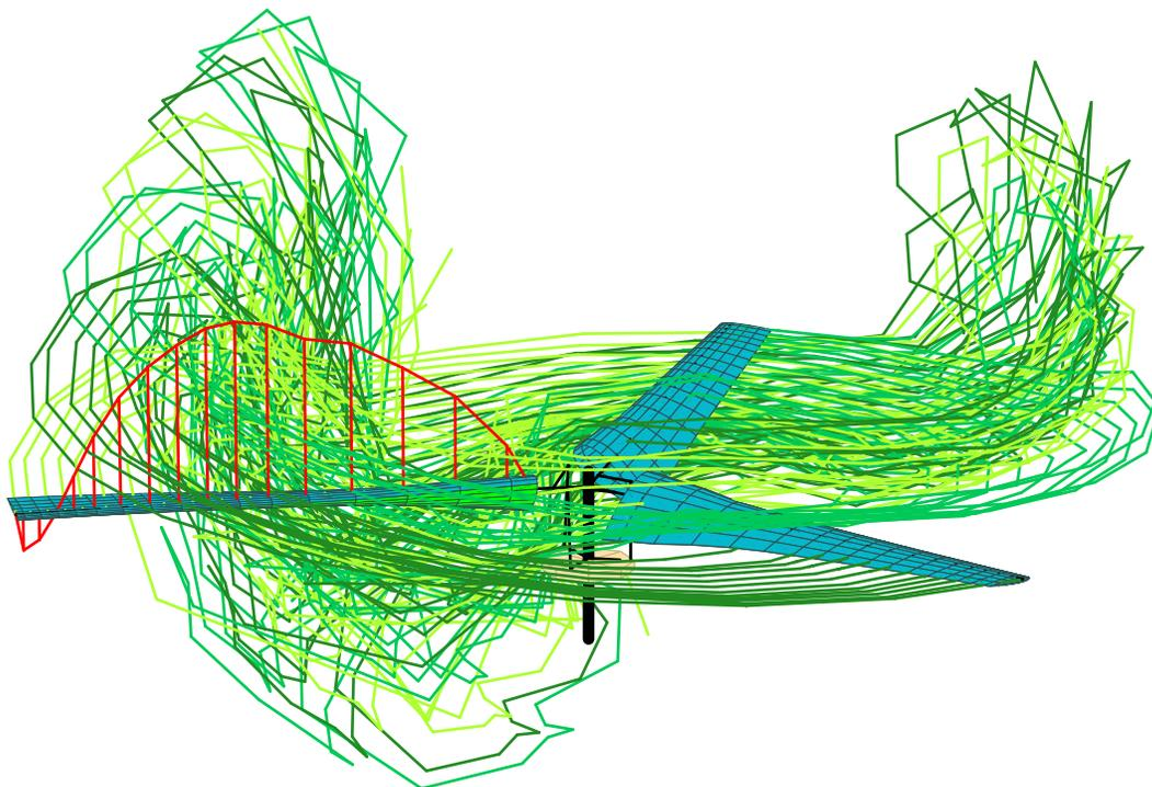
Figure 25b. Calculated TRAM wake geometry and loading for  $\mu = 0.15$ ,  $\alpha_s = 6$ ,  $C_T/\sigma = 0.089$ .
