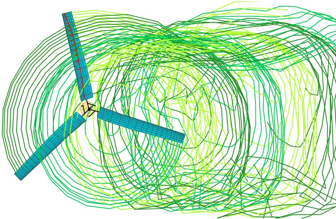
Figure 27a. Calculated TRAM wake geometry and loading for  $\mu = 0.15$ ,  $\alpha_s = 6$ ,  $C_T/\sigma = 0.128$ .
