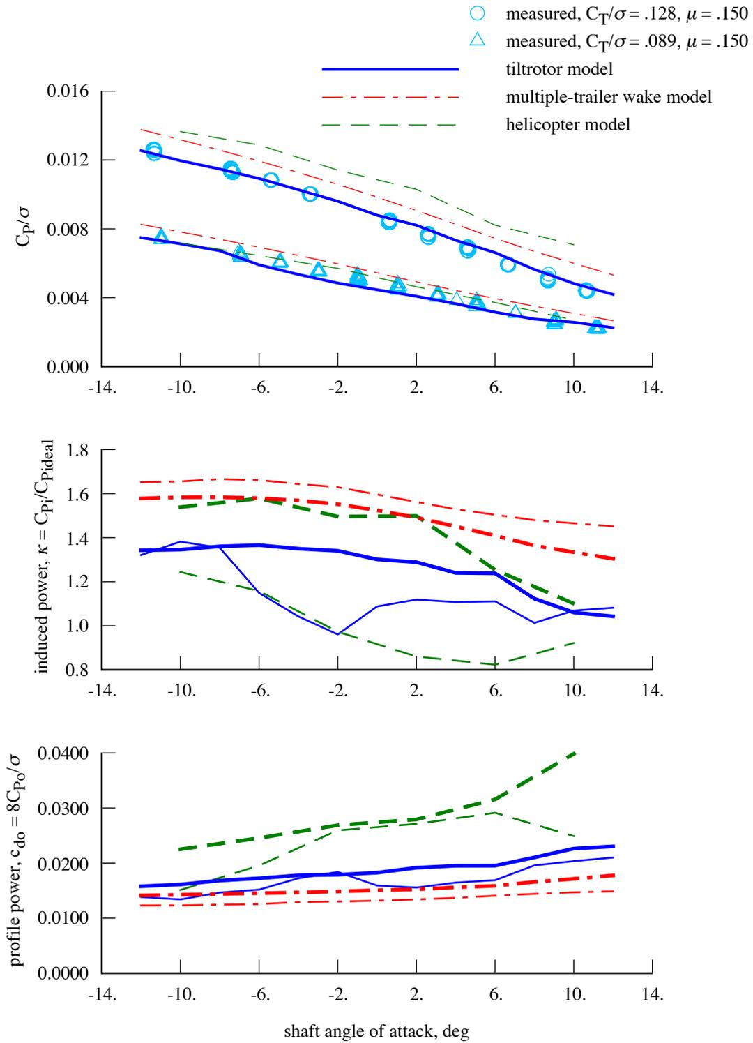
Figure 8. TRAM helicopter mode performance calculated using tiltrotor and helicopter aerodynamic and wake models ( $\mu = 0.15$ ; in lower two figures, heavy line  $C_T/\sigma = 0.128$ , thin line  $C_T/\sigma = 0.089$ ).
