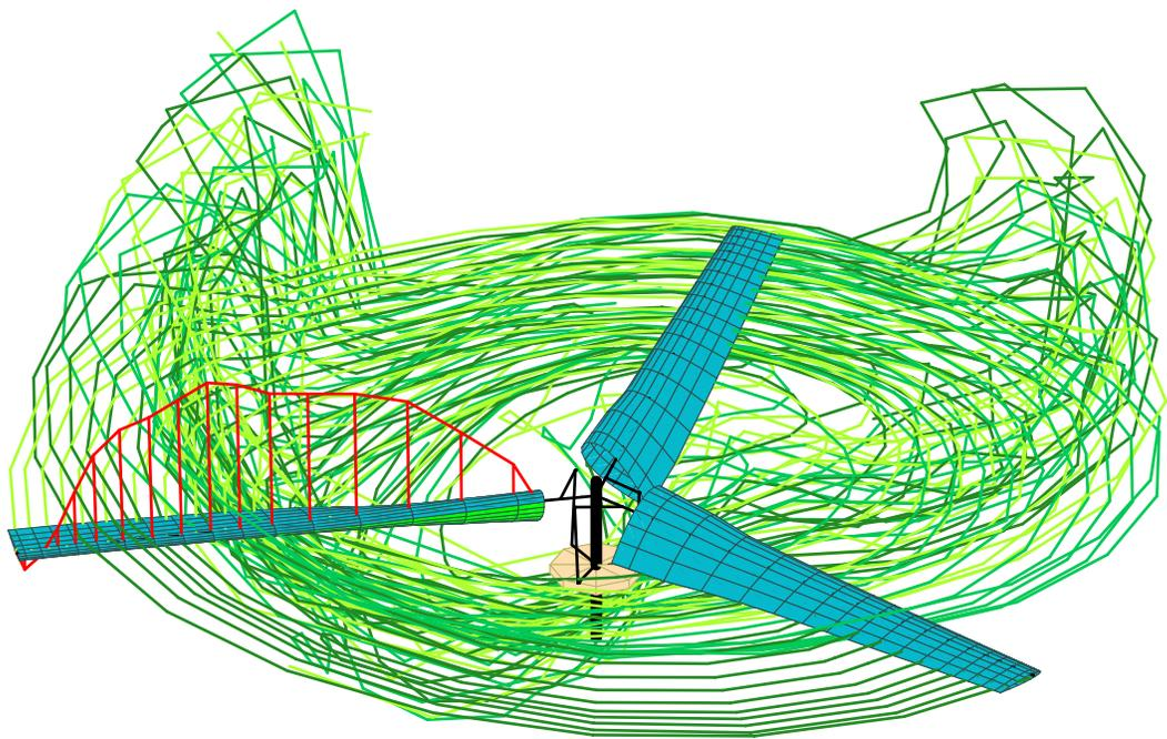
Figure 24b. Calculated TRAM wake geometry and loading for  $\mu = 0.15$ ,  $\alpha_s = -6$ ,  $C_T/\sigma = 0.089$ .
