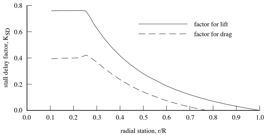
Figure 4. Stall delay factor for TRAM blade.
