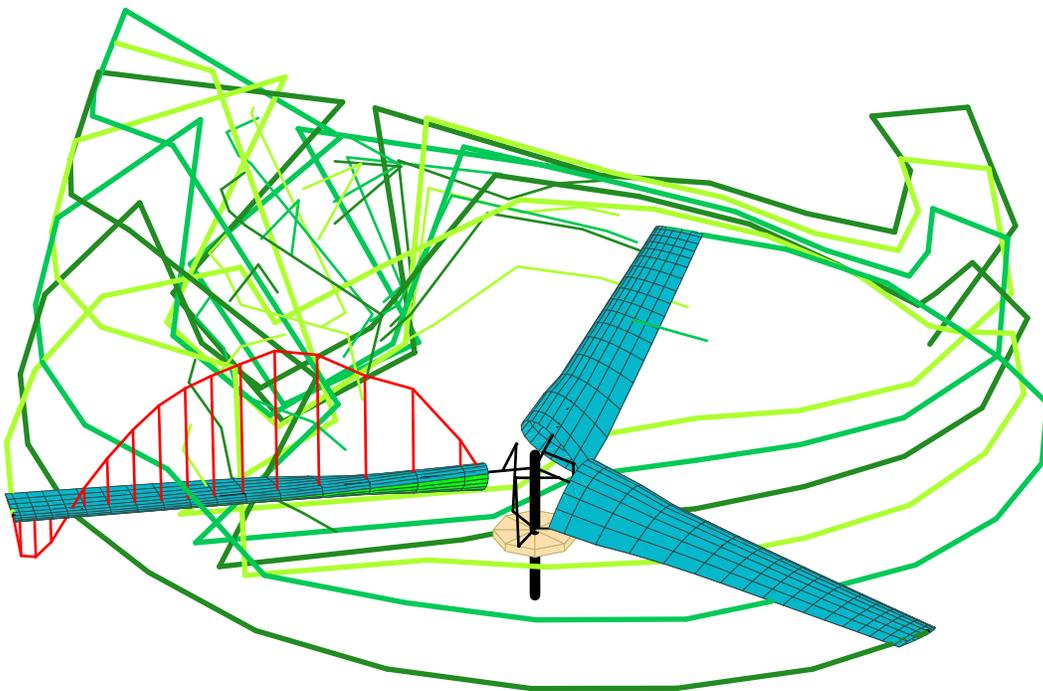
Figure 22b. Calculated TRAM wake geometry and loading for  $\mu = 0.15$ ,  $\alpha_s = -6$ ,  $C_T/\sigma = 0.089$ .
