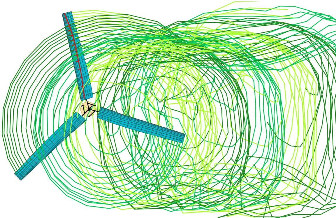
Figure 27b. Calculated TRAM wake geometry and loading for  $\mu = 0.15$ ,  $\alpha_s = 6$ ,  $C_T/\sigma = 0.089$ .
