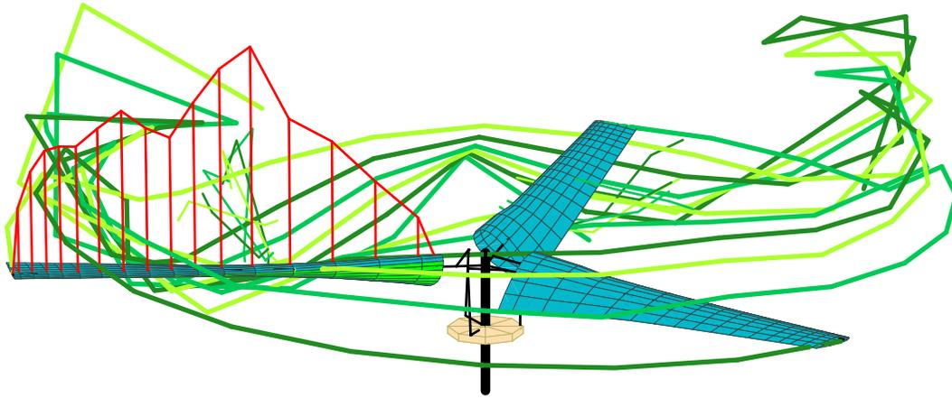
Figure 23a. Calculated TRAM wake geometry and loading for  $\mu = 0.15$ ,  $\alpha_s = 6$ ,  $C_T/\sigma = 0.128$ .
