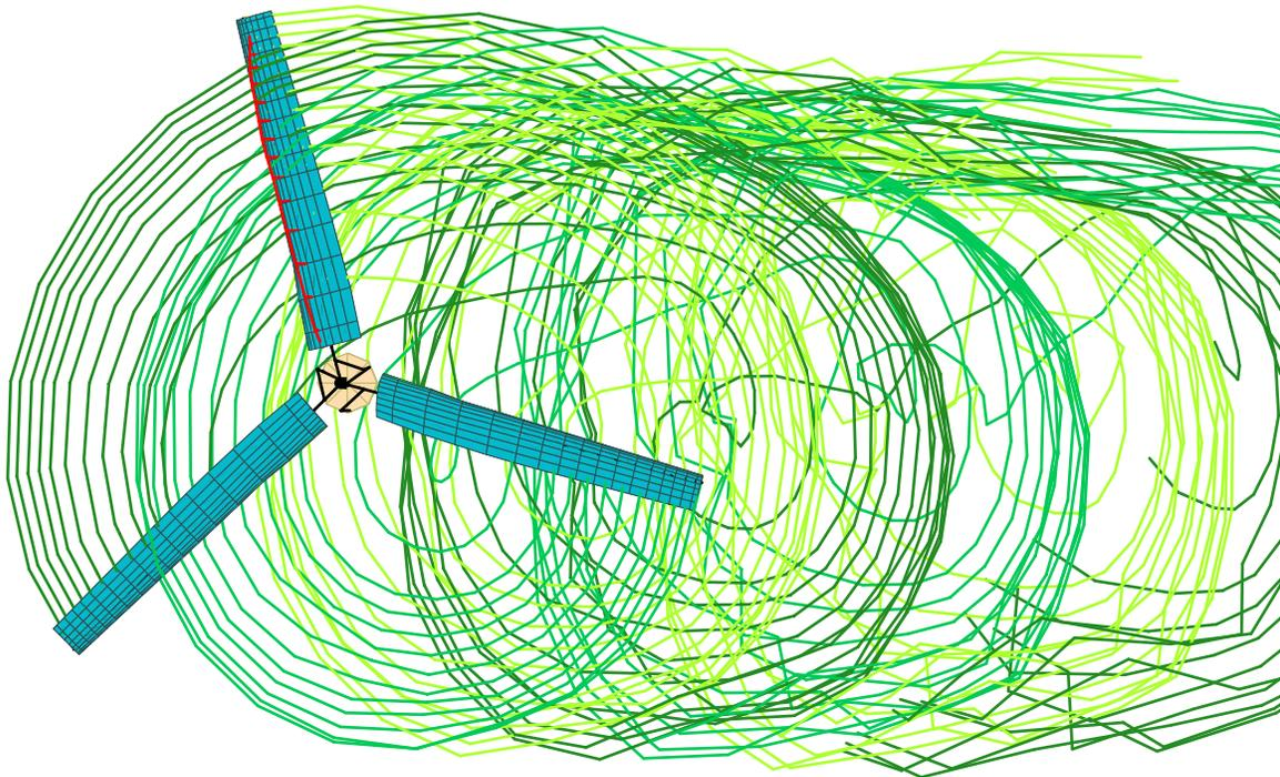
Figure 26b. Calculated TRAM wake geometry and loading for  $\mu = 0.15$ ,  $\alpha_s = -6$ ,  $C_T/\sigma = 0.089$ .
