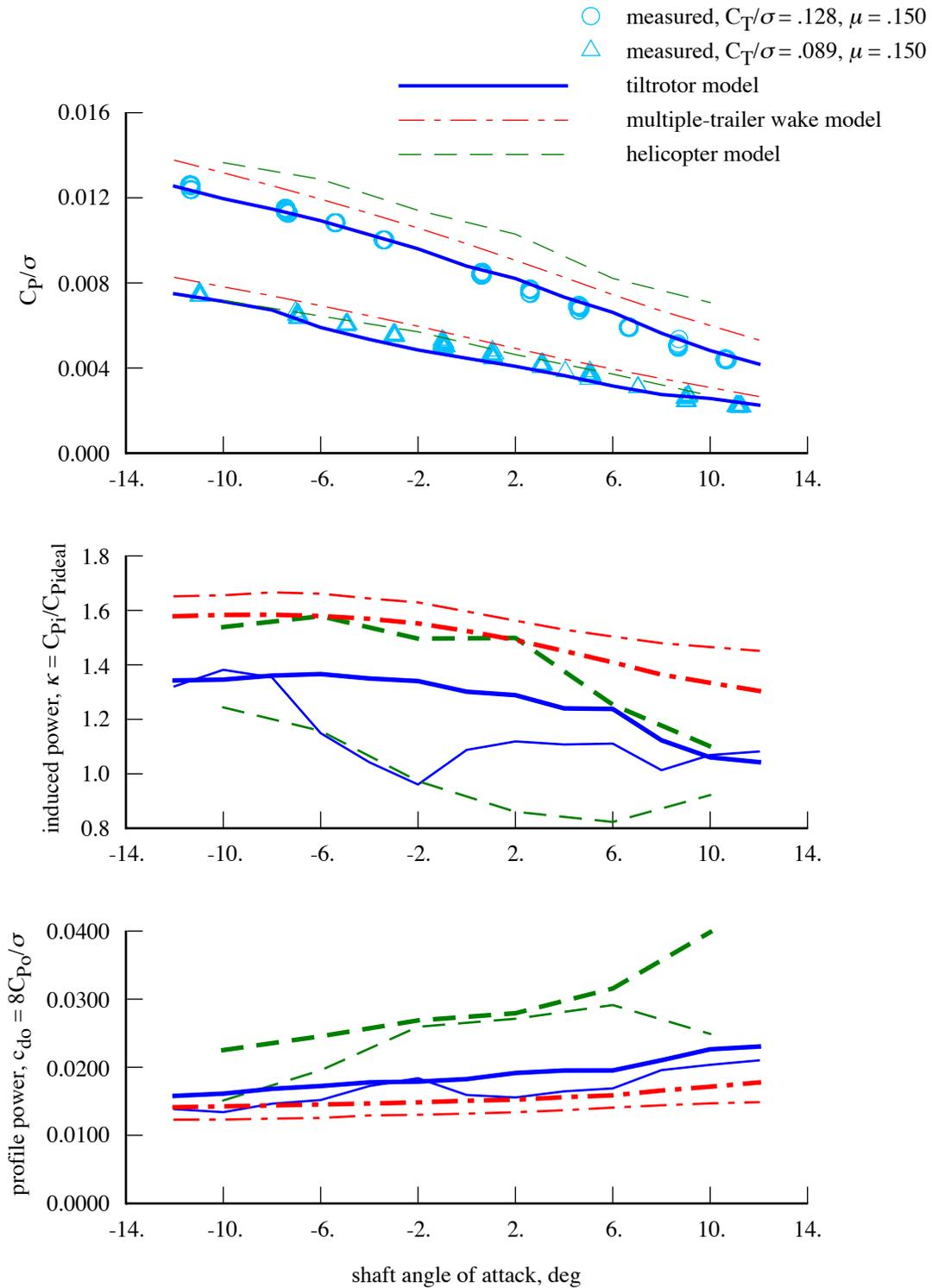
Figure 8. TRAM helicopter mode performance calculated using tiltrotor and helicopter aerodynamic and wake models ( $\mu = 0.15$ ; in lower two figures, heavy line  $C_T/\sigma = 0.128$ , thin line  $C_T/\sigma = 0.089$ ).
