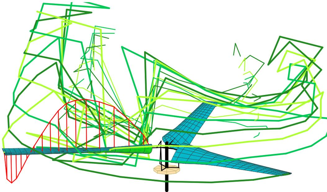
Figure 23b. Calculated TRAM wake geometry and loading for  $\mu = 0.15$ ,  $\alpha_s = 6$ ,  $C_T/\sigma = 0.089$ .
