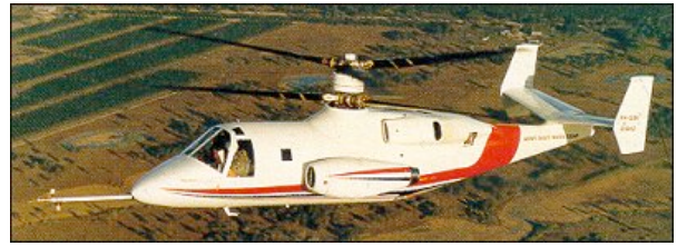
XH-59A coaxial lift-offset helicopter
