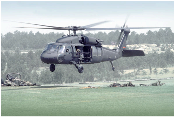
UH-60A single-main rotor and tail-rotor helicopter
