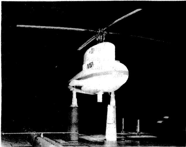
Figure 1. Installation of the RTA and BO 105 rotor in the NASA Ames 40- by 80-Foot Wind Tunnel.
