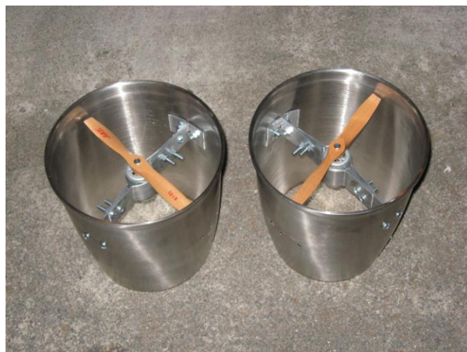
Fig. 5 – Fan & Electric Motor Installation in the Ducts
