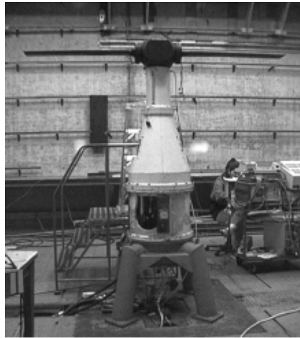
Fig. 1(b). Photograph of test stand installed in hover chamber.
