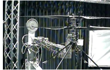
Figure 6: Ingenuity prototype, engineering development model, and flight model system identification testing on swinging arm and gimbal system [32].
