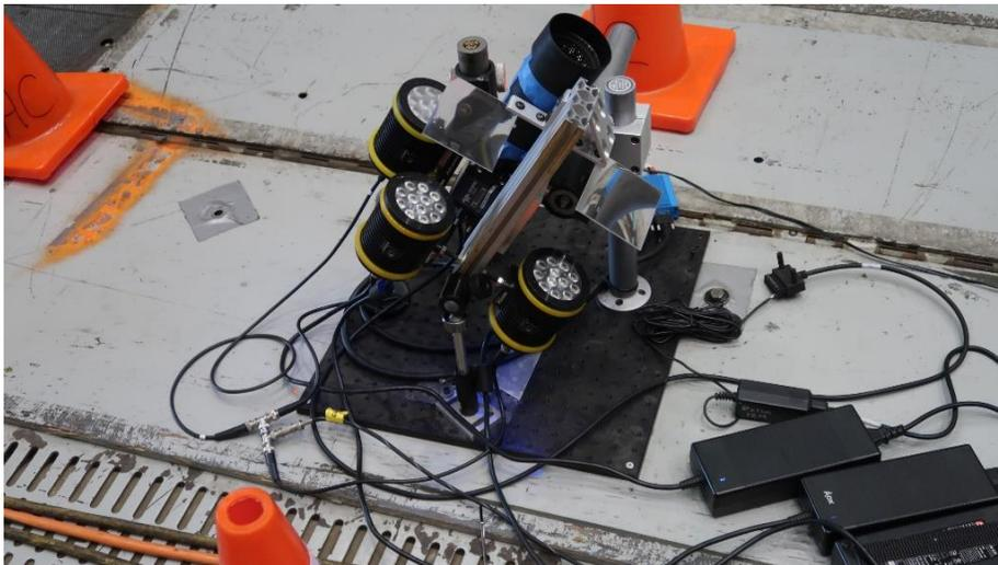
Figure 8. North camera and lamps mounted on the floor of the test section.
