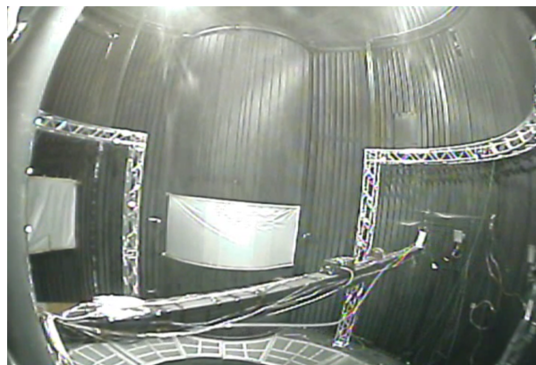
Fig. 14 The helicopter in the swinging-arm configuration. The 3-m long arm was swung back and forth to generate airflow over the rotor.
