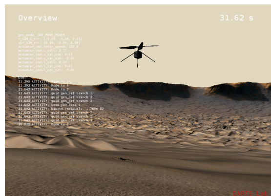
Fig. 11 HeliCAT visualization of the helicopter flying on Mars, with flight software in the loop.
