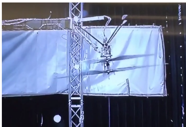
Fig. 15 The helicopter in the gimbal configuration. The helicopter was placed upside-down due to improved air recirculation properties within the chamber and to make it easier to restrain during spinup and spindown.
