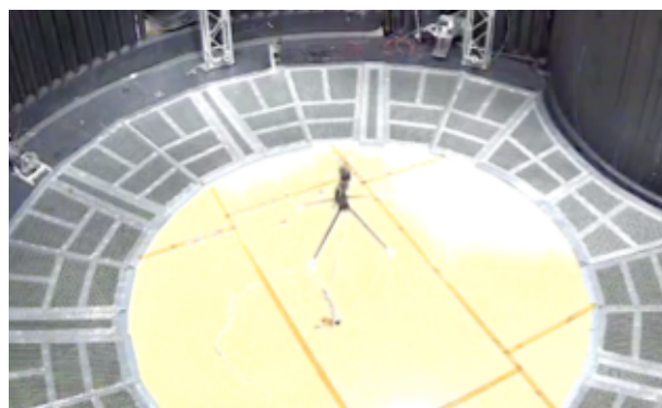
Fig. 2 In this image, the Mars Helicopter demonstration vehicle is taking off for the first controlled flight in Martian atmospheric conditions, inside JPL's 25-ft Space Simulator.
