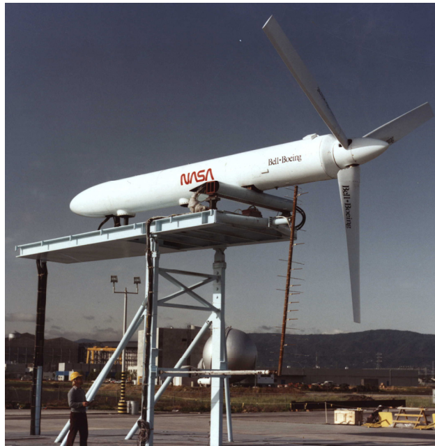
Figure 1. The JVX rotor mounted on the PTR for hover tests at the OARF.
