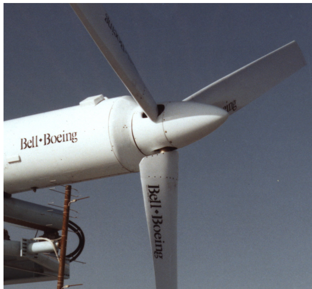
Figure 30. Close-up of the JVX rotor on the PTR in the OARF test configuration.
