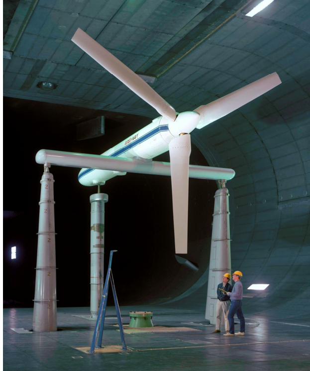
Figure 2. The JVX rotor mounted on the PTR for airplane-mode tests in the NFAC.
