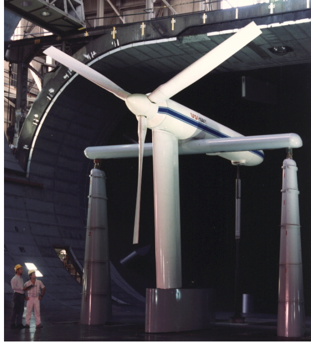
Figure 31. The JVX rotor on the PTR with the wing in airplane mode.
