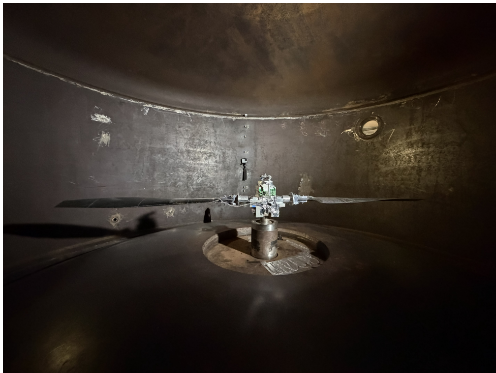
Figure 8. The University of Maryland's 10-foot diameter vacuum chamber.
