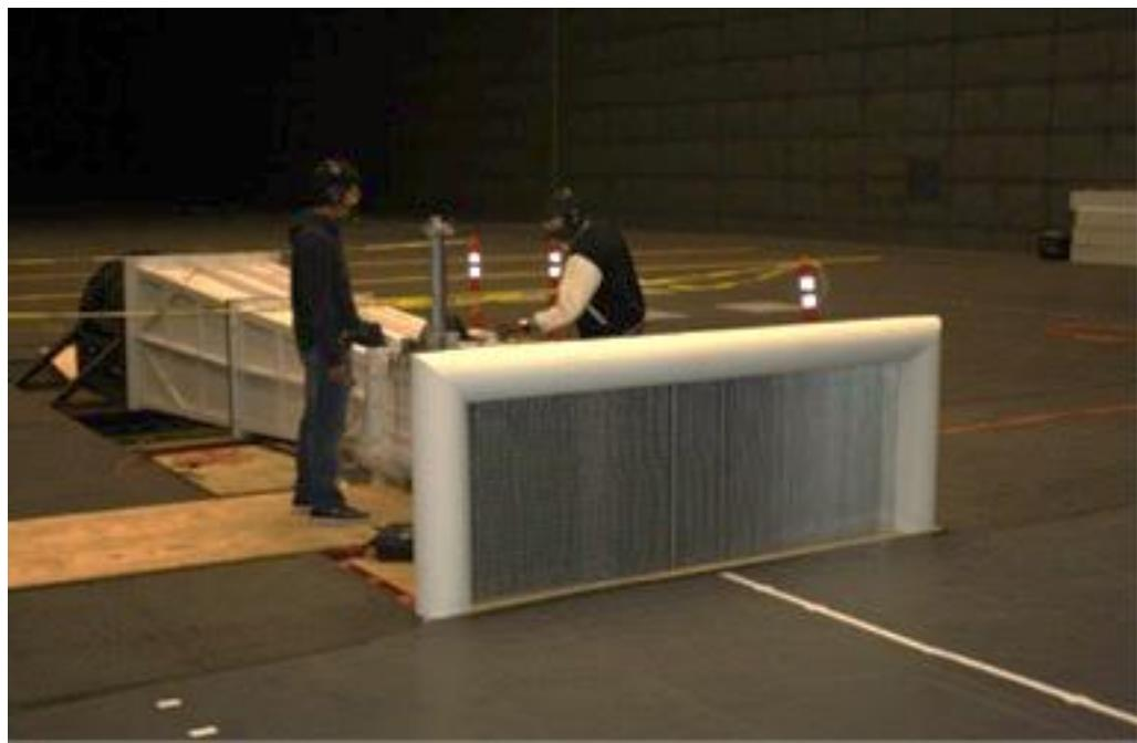
Figure 6. Guide vanes installed in model inlet.
