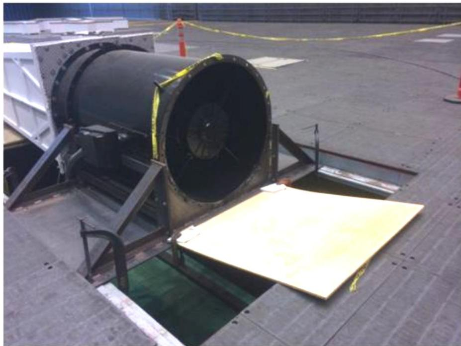
Figure 7. Chicago Blower Co. D/47 vane axial fan attached to rear of 1/50th-scale model.
