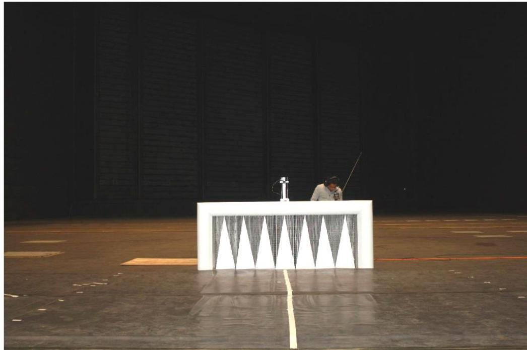
Figure 14. Model inlet with small spires.
