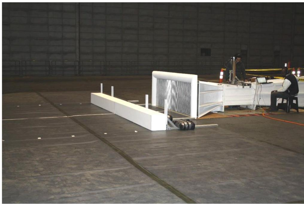
Figure 13. 1/50th-scale model with 1-foot-tall 2D upwind blockage.
