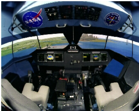
Fig. 5. Simulator cockpit interior. Final approach to notional San Francisco Vertiport shown in visual scene.
