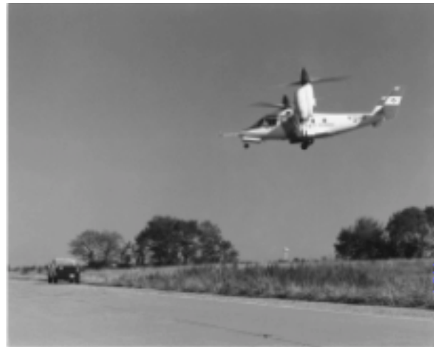
Fig. 1. XV-15 Tiltrotor Research Aircraft shown on final approach during October, 1999 Noise Measurement Flight Test.
