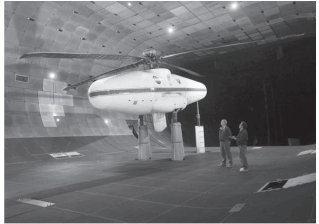
(a) Full-scale UH-60A rotor installation
