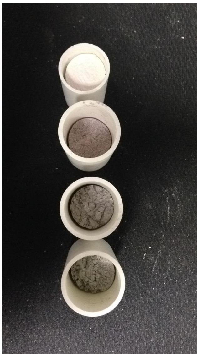
Figure 15. Doped TCP powders in crucibles after calcination.
