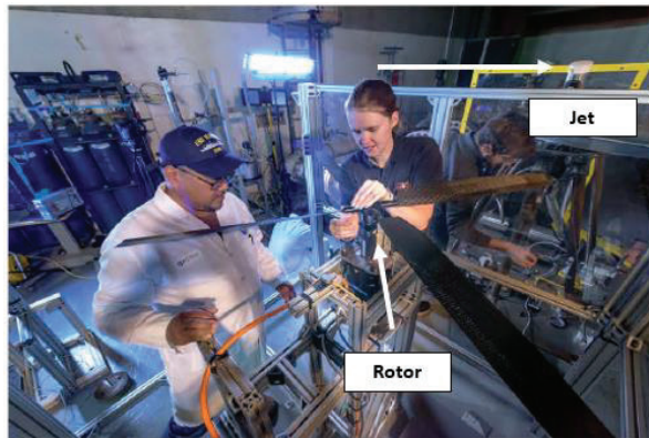
Figure 14. Team members installing rotor next to single jet in Planetary Aeolian Lab.
