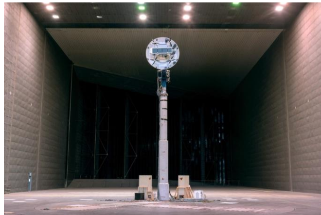
Figure 6. NASA ARC NFAC 80-by 120-ft. Wind Tunnel Test, Dragonfly Scale Model with Entry Backshell.
