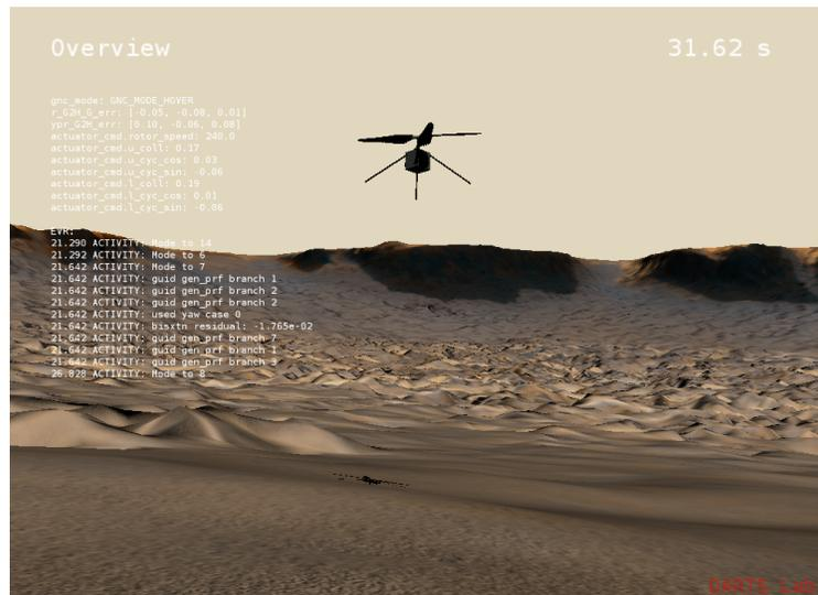
Fig. 4 HeliCAT visualization of the helicopter flying on Mars, with flight software in the loop.
