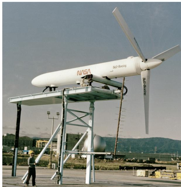
Fig. 1. The JVX rotor mounted on the PTR for hover tests at the OARF.
