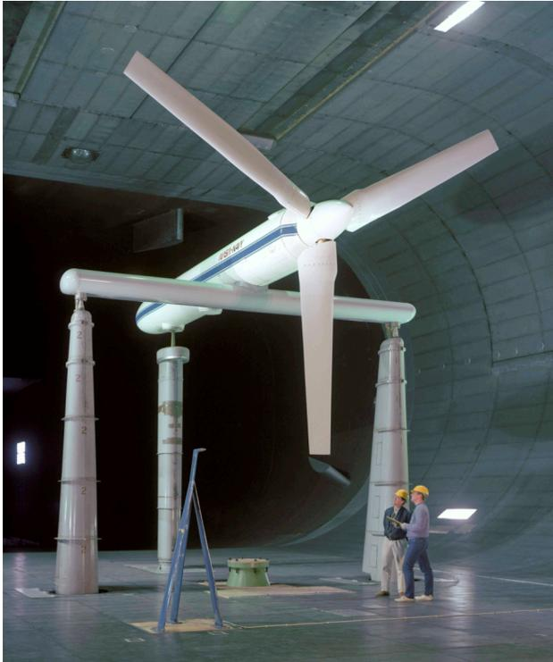
Fig. 2. The JVX rotor mounted on the PTR for airplane-mode tests in the NFAC.
