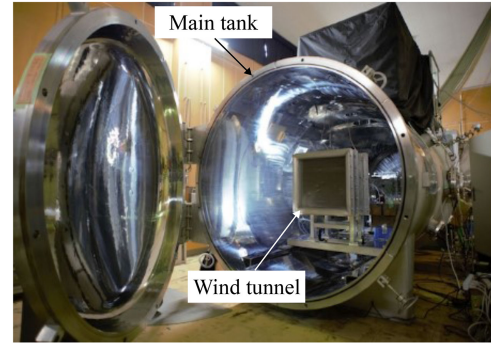
Fig. 5 The MWT at Tohoku University, Japan. The facility is now located at Nagoya University, Japan.
