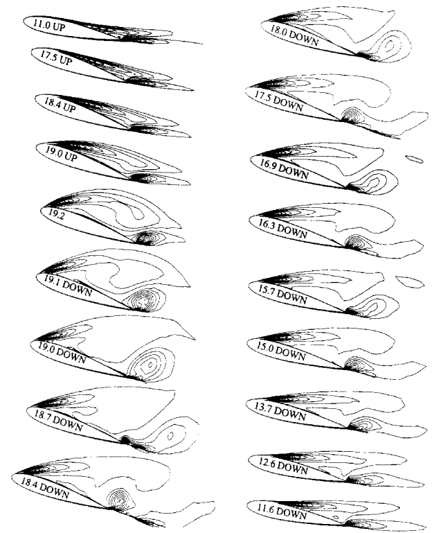
Fig. 4 Vorticity contours for oscillating NACA 0015 airfoil: \alpha (deg) = 15 + 4.2 \sin(2k M_\infty t + 1.57\pi) , M_\infty = 0.29 , Re = 1.95 \times 10^6 , and k = 0.1 .
