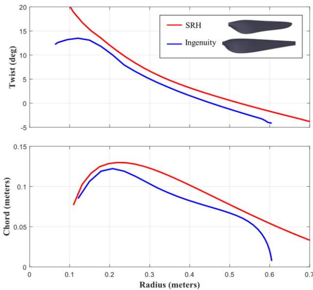
**Figure 7. Twist (deg, top) and chord (m, bottom) for SRH (red) and Ingenuity blade (blue).**
