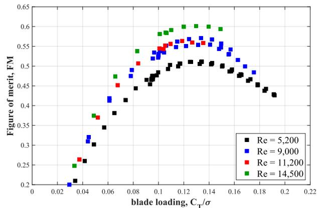
**Figure 8. Figure of merit versus blade loading for EDM-1 in the JPL 25-ft. Space Simulator.**
