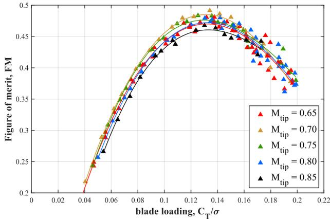
**Figure 9. Figure of merit versus blade loading for TRT in the JPL SS.**
