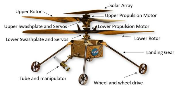
**Figure 3. Labeled SRH diagram. Credit: Mars Sample Return Program.**
