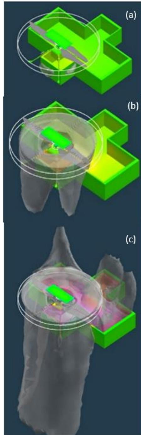
**Figure 5. RotCFD- 15 m/s outwash building with time and interacting with LAIR (accommodation box). Time =8 (a), 12 (b), and 20 (c) seconds from top to bottom.**
