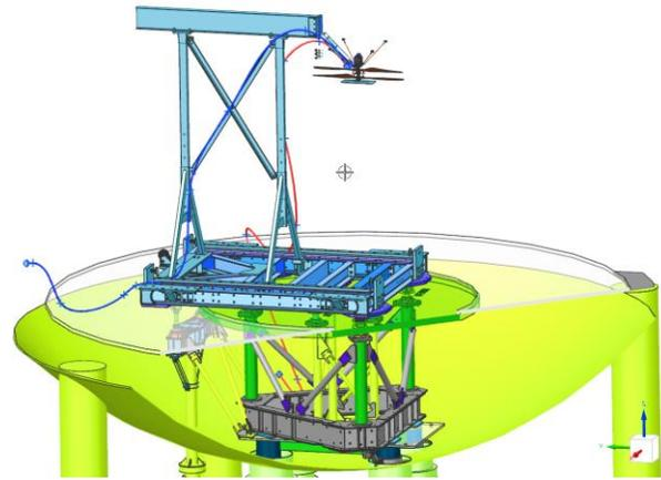
**Figure 6. CAD of Ingenuity EDM-1 Test Set Up. Credit: JPL.**
