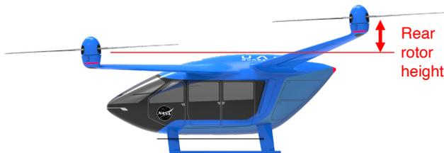
**Figure 5. Quadrotor rear rotor vertical placement**
