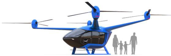
**Figure 4. Rendering of a quadrotor concept aircraft**
