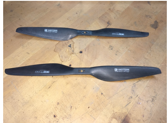
Figure 3. T-Motor Carbon Fiber 15x5 blades.
