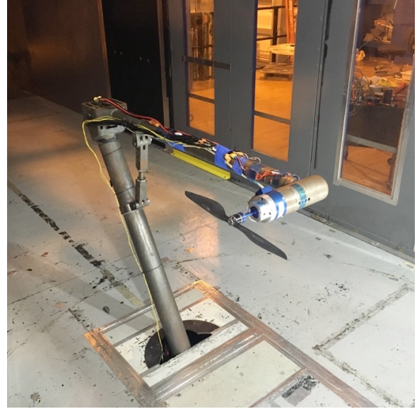
Figure 1. SUI Endurance isolated rotor hover test configuration.
