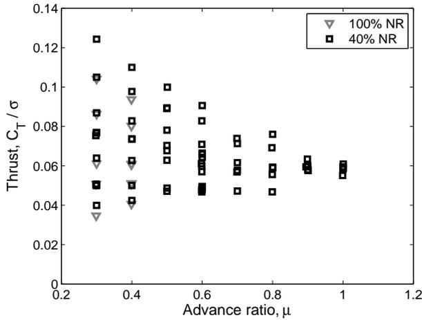
Figure 7: Non-dimensional thrust vs. speed at 4° shaft angle (tilt back).
