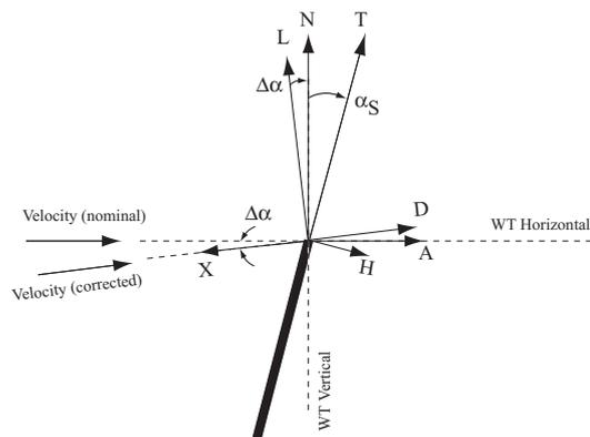
Figure 2: **Model shaft angle  $\alpha_S$ , wall correction  $\Delta\alpha$ , and rotor forces in tunnel axes (N and A), shaft axes (T and H), and corrected wind axes (L and D), and the propulsive force (X = -D).**
