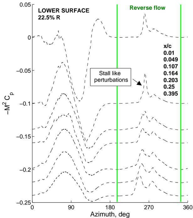
Figure 45: Lower surface pressures at 22.5% R;  $\mu = 0.8$ ;  $C_T/\sigma = 0.045$  ( $\theta_{75} = 8^\circ$ ),  $\alpha_S = 0^\circ$ ; 40% NR; (P9159).
