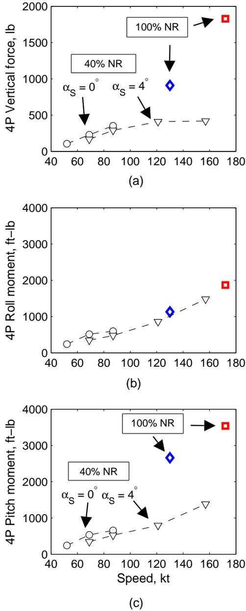
Figure 41: **Vibratory hub loads vs. speed for nominal and 40% NR slowed rotors; nominal:  $\mu = 0.3, C_T/\sigma = 0.082, \alpha_S = 0^\circ$  (P6619) (symbol- $\diamond$ );  $\mu = 0.4, C_T/\sigma = 0.071, \alpha_S = 0^\circ$ , (P6912) (symbol- $\square$ ); slowed: speed sweep at  $C_T/\sigma = 0.06, \alpha_S = 0^\circ$  (symbol- $\circ$ ) and at  $C_T/\sigma = 0.06, \alpha_S = 4^\circ$  (symbol- $\nabla$ ).**
