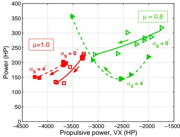
Figure 22: **Total power vs. propulsive power (HP) for advance ratios  $\mu = 0.8$  (green),  $0.9$  (blue) and  $1.0$  (red) at shaft angles  $0^\circ$  (open symbols) and  $4^\circ$  (solid symbols); arrows mark direction of increasing collective.**
