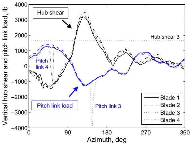
Figure 39: **Vertical hub shear and pitch link loads on four blades;**  $\mu = 0.9$ ,  $C_T/\sigma = 0.063$ ,  $\alpha_S = 4^\circ$ ; 40% NR.
