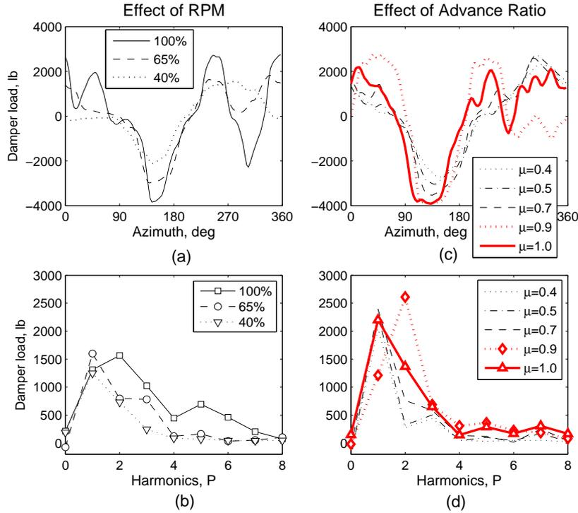
Figure 38: **Effect of RPM and advance ratio variation on damper loads;** (a) and (b):  $\mu = 0.4$ ,  $C_T/\sigma = 0.07$ ,  $\alpha_S = 0^\circ$ ; (c) and (d):  $C_T/\sigma \approx 0.06$ ,  $\alpha_S = 4^\circ$ ; 40% NR.
