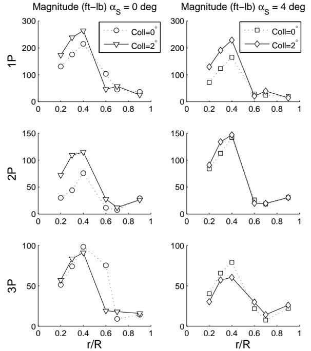
Figure 33: Effect of collective increase on 1-3/rev torsion moments at  $\mu = 1.0$  for two different shaft angles;  $\alpha_S = 0^\circ$  ( $\theta_{75}=0^\circ$  and  $2^\circ$  produces  $C_T/\sigma = 0.019$  and  $0.022$ ) and  $\alpha_S = 4^\circ$  ( $\theta_{75}=0^\circ$  and  $2^\circ$  produces  $C_T/\sigma = 0.061$  and  $0.059$  – reversal); 40% NR.
