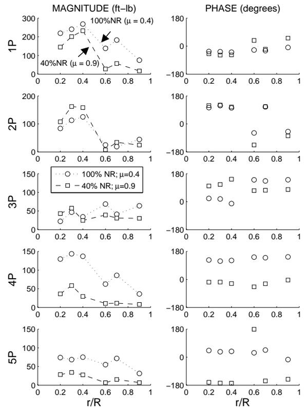
Figure 30: Torsion moment harmonics for nominal and 40% NR slowed rotor; nominal:  $\mu = 0.4$ ,  $C_T/\sigma = 0.07$ ,  $\alpha_S = 0^\circ$ ; slowed:  $\mu = 0.9$ ,  $C_T/\sigma = 0.06$ ,  $\alpha_S = 4^\circ$ .
