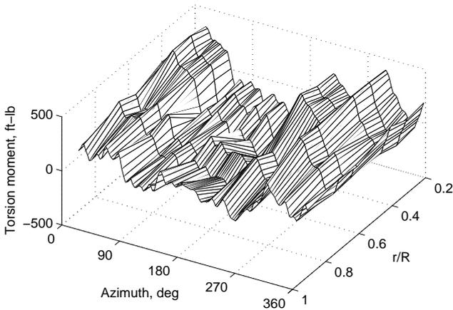
Figure 28: Torsion moment at 100% NR;  $\mu = 0.4$ ,  $C_T/\sigma = 0.07$ ,  $\alpha_S = 0^\circ$ .
