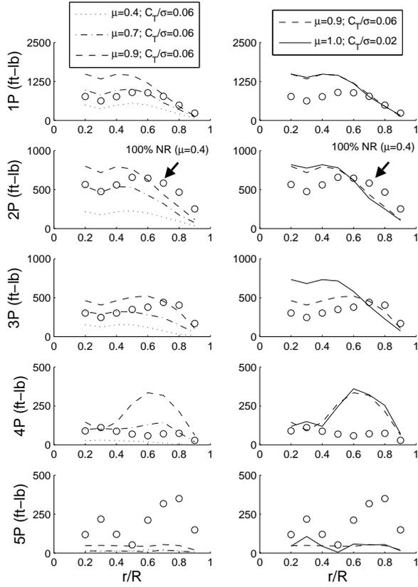
Figure 27: Flap bending moment harmonics for nominal and 40% NR slowed rotor; nominal:  $\mu = 0.4$ ,  $C_T/\sigma = 0.07$ ,  $\alpha_S = 0^\circ$  (shown as symbols- $\circ$ ); slowed:  $\mu = 0.4-0.9$ ,  $C_T/\sigma = 0.06$ ,  $\alpha_S = 4^\circ$  and  $\mu = 1.0$ ,  $C_T/\sigma = 0.02$ ,  $\alpha_S = 0^\circ$  (shown as lines).
