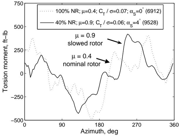
Figure 31: Torsion moment at 30% R for nominal and 40% NR slowed rotor; nominal:  $\mu = 0.4$ ,  $C_T/\sigma = 0.07$ ,  $\alpha_S = 0^\circ$ ; slowed:  $\mu = 0.9$ ,  $C_T/\sigma = 0.06$ ,  $\alpha_S = 4^\circ$ .
