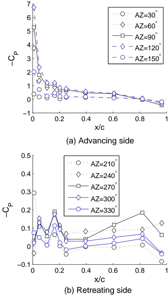
Figure 49: **Chord-wise pressures along 67.5% R lower surface on advancing and retreating sides;**  $\mu = 0.9$ ;  $C_T/\sigma = 0.063$  ( $\theta_{75} = 6.2^\circ$ ),  $\alpha_S = 4^\circ$ ; **40% NR; (P9528).**
