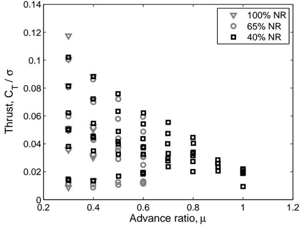
Figure 6: Non-dimensional thrust vs. speed at 0° shaft angle.
