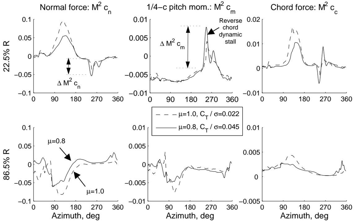
Figure 54: Sectional airloads at 22.5% and 86.5% R for the 40% NR slowed rotor at two high advance ratio points:  $\mu = 1.0, C_T/\sigma = 0.022, \theta = 2^\circ, \alpha_S = 0^\circ$  (P9175); and  $\mu = 0.8, C_T/\sigma = 0.045, \theta = 8^\circ, \alpha_S = 0^\circ$  (P9159).
