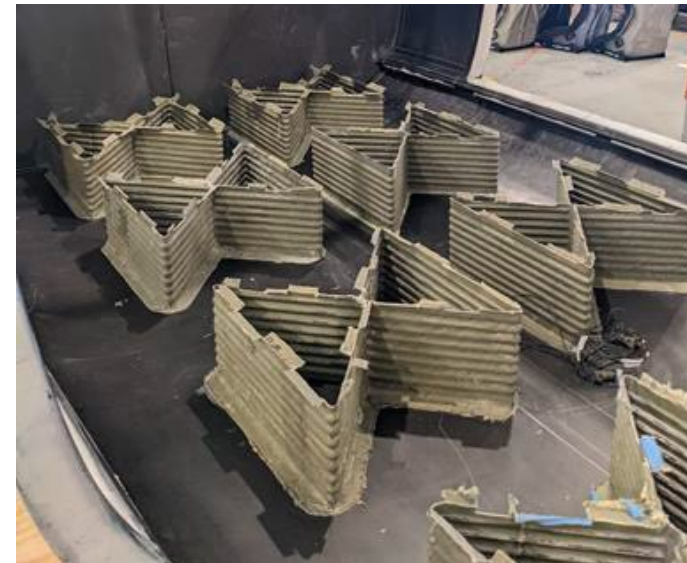
Lift+Cruise cabin crash test article structural components
