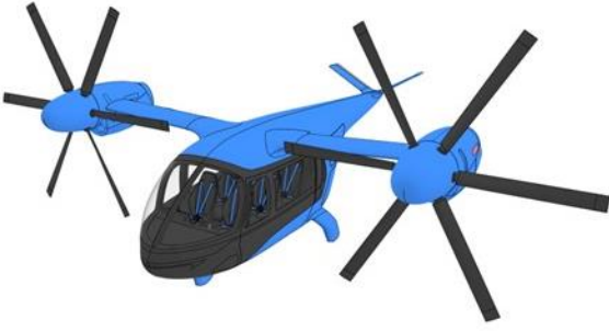
Figure 1. Rendering of the tiltrotor UAM reference vehicle in airplane mode
