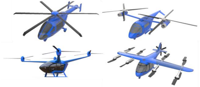
Figure 13. QSMR (top left), side-by-side (top right), quadrotor (bottom left), and lift+cruise (bottom right) reference vehicles
