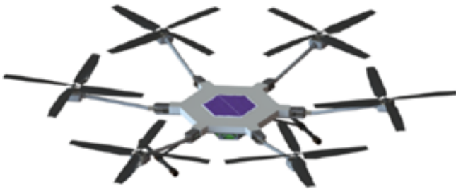
Figure 1. Mars Science Helicopter conceptual design [3].
