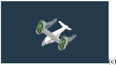
Figure 34. Hover and low-speed first generation (consistent with a UAV or small aircraft) 2DOF tilting/pivoting ducted fan aerial vehicle and rotor wakes: (a) hover, i_N=90 Deg.; (b) in the middle of tilt transition, 150 ft/s, i_N=60 Deg.; (c) near the end of tilt transition, 200 ft/s, i_N=30 Deg.
