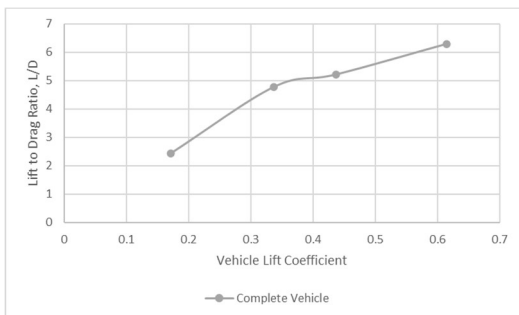
Figure 28. Complete first generation PPT vehicle lift-to-drag ratio, L/D
