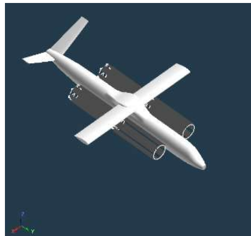
Figure 15. Isometric view of stopped rotor cycloidal vehicle
