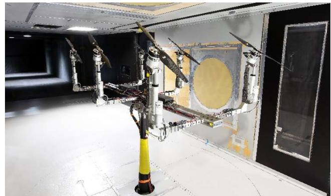
Figure 2. MTB installed in the U.S. Army 7- by 10-ft Wind Tunnel
