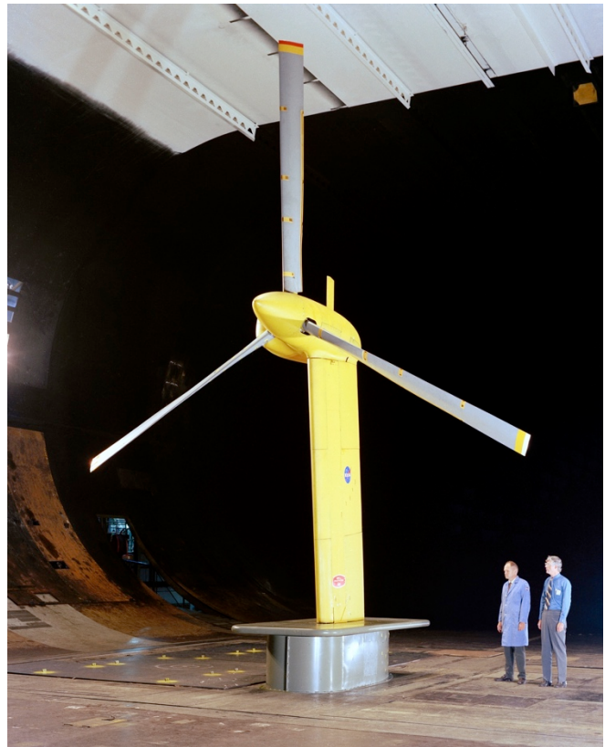
Fig. 6. XV-15 rotor on the Dynamic Test Stand (1970).
