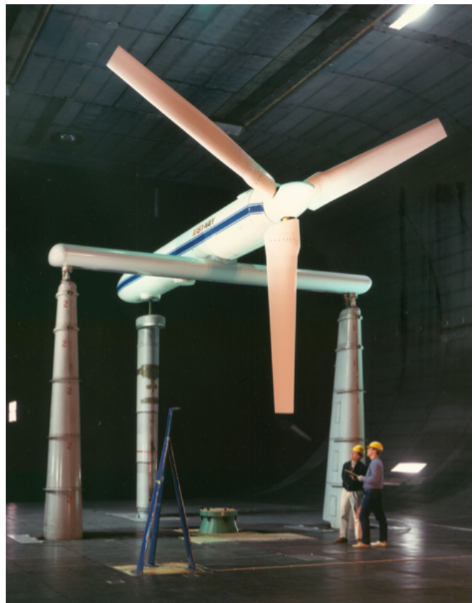
Fig. 4. Scaled JVX rotor on the Prop Test Rig (1991).
