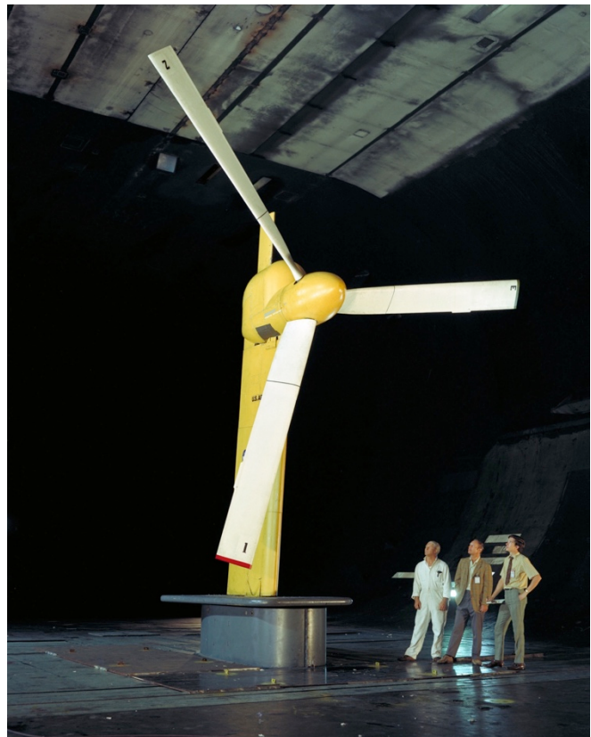
Fig. 7. Boeing 222 semi-span wing and rotor (1972).
