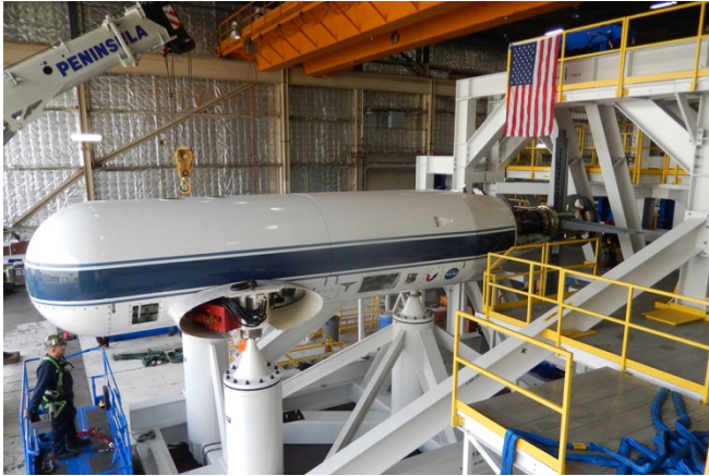
Fig. 16. TTR installed in the Calibration Rig, with metric hardware in place of the rotor.
