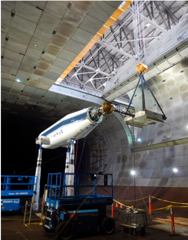
Fig. 19. Shake test with lateral input at the rotor hub.
