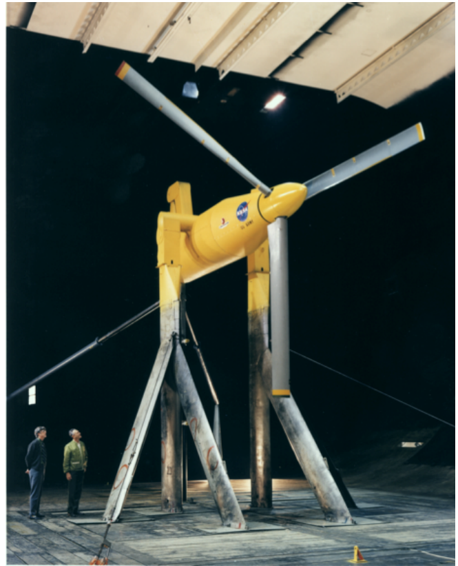
Fig. 3. Bell XV-15 rotor on the Propeller Test Rig (1970).
