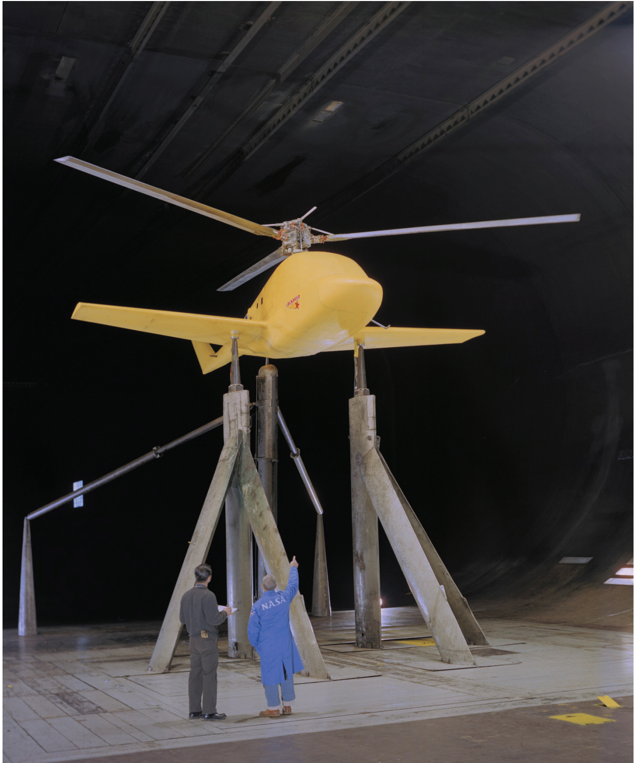
Figure 137. Lockheed stoppable rotor in lifting mode. (NASA A-36028)
