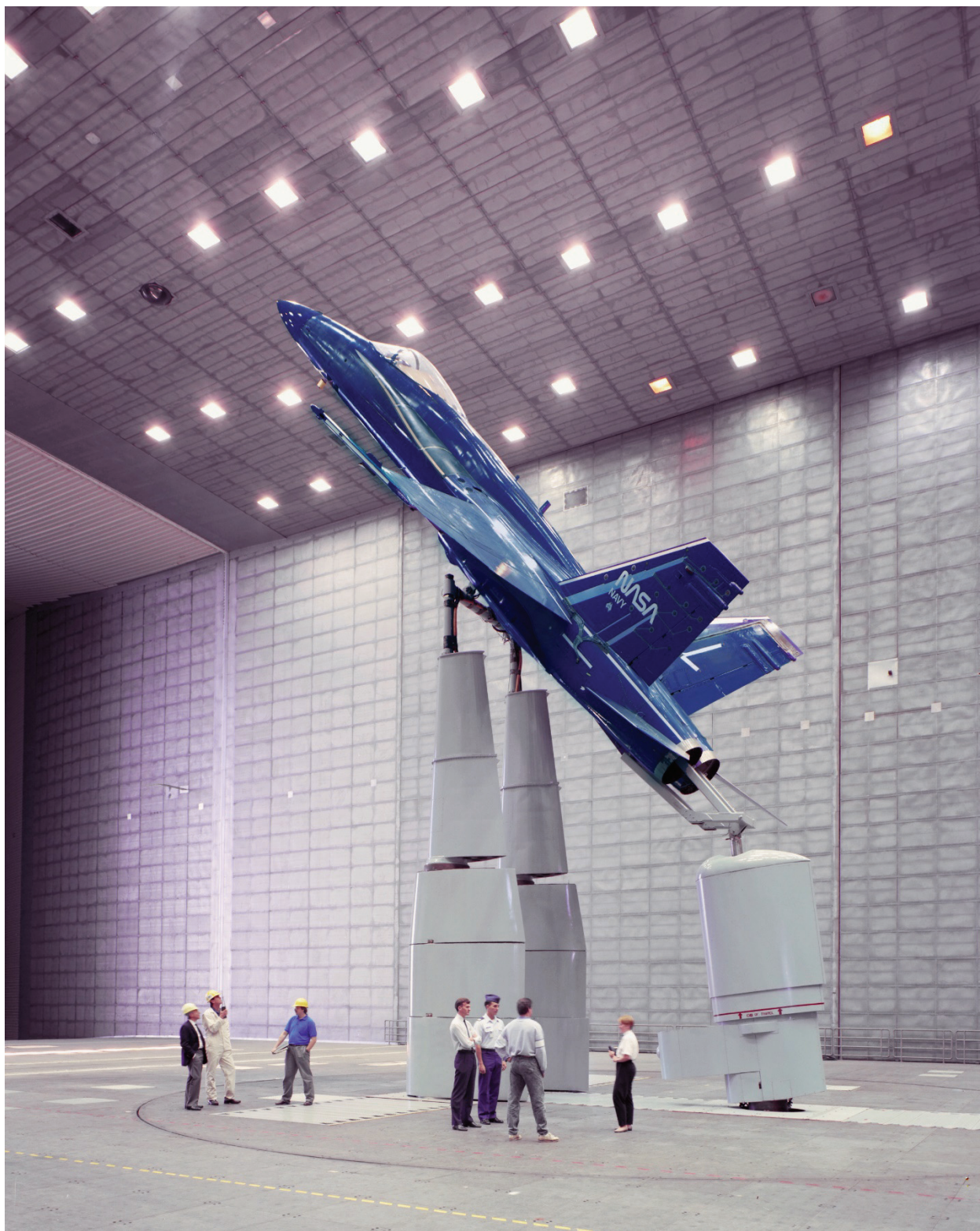
Figure 258. McDonnell Douglas F-18 fighter in the 80- by 120-foot test section at high angle of attack. (NASA AC91-0255-75)
