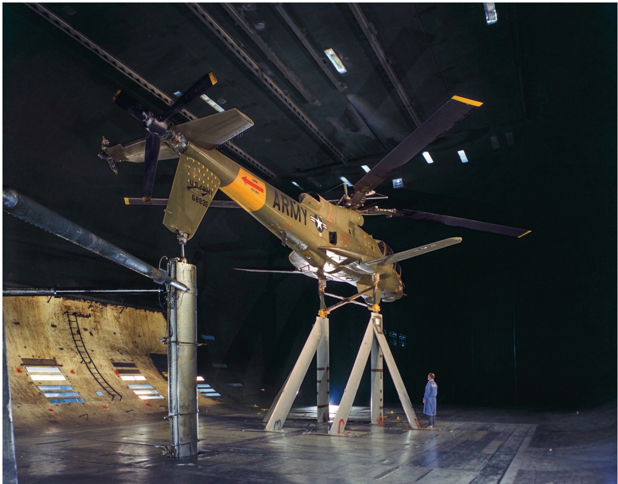
Figure 142. Three-quarter rear view of the Lockheed AH-56 Cheyenne showing the pusher propeller. (NASA AC-42561-2)
