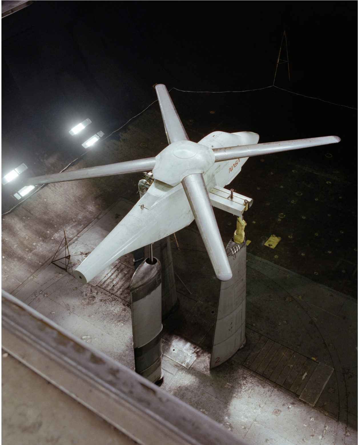
Figure 146. Overhead view of the X-wing helicopter model. (NASA AC79-0367-1)
