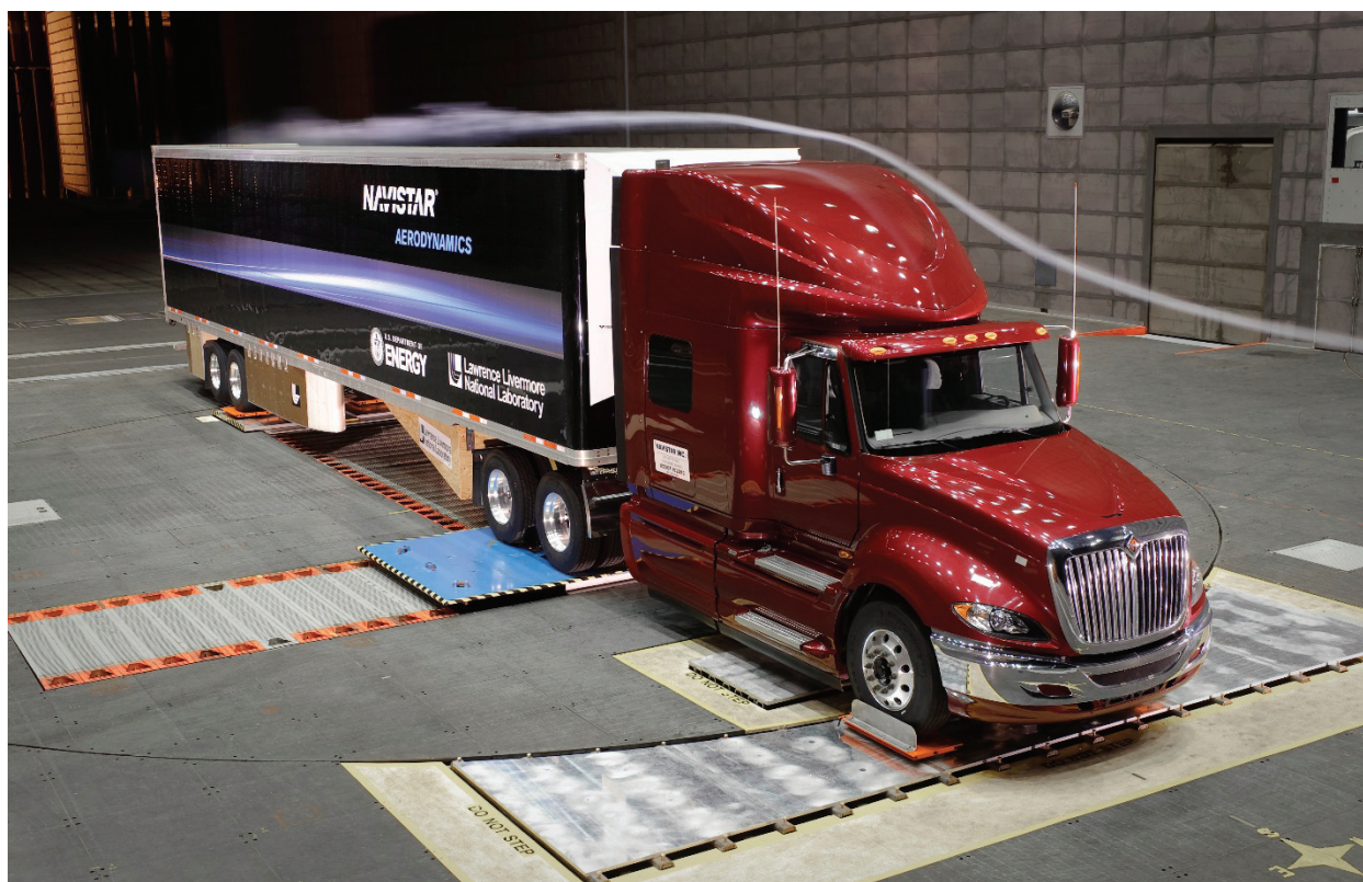
Figure 283. Smoke flow visualization studies of truck with trailer in the 80- by 120-foot test section. (NASA ACD10-0020-065)
