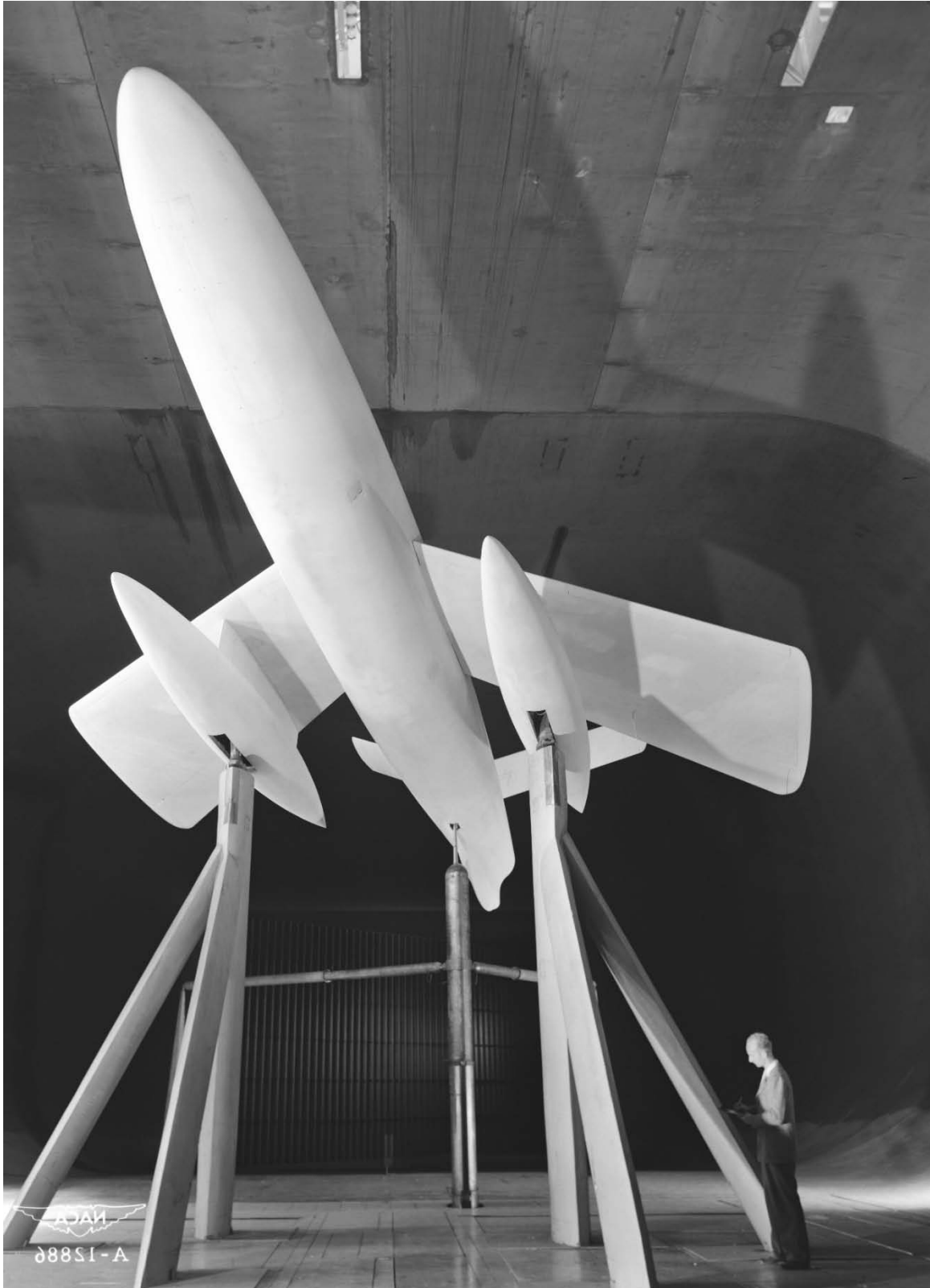
Figure 67. Front view of the Republic XF-91 experimental airplane. The reverse taper is shown (that is, the wingtip chord is greater than the wing root chord). ( NACA A-12886 )
