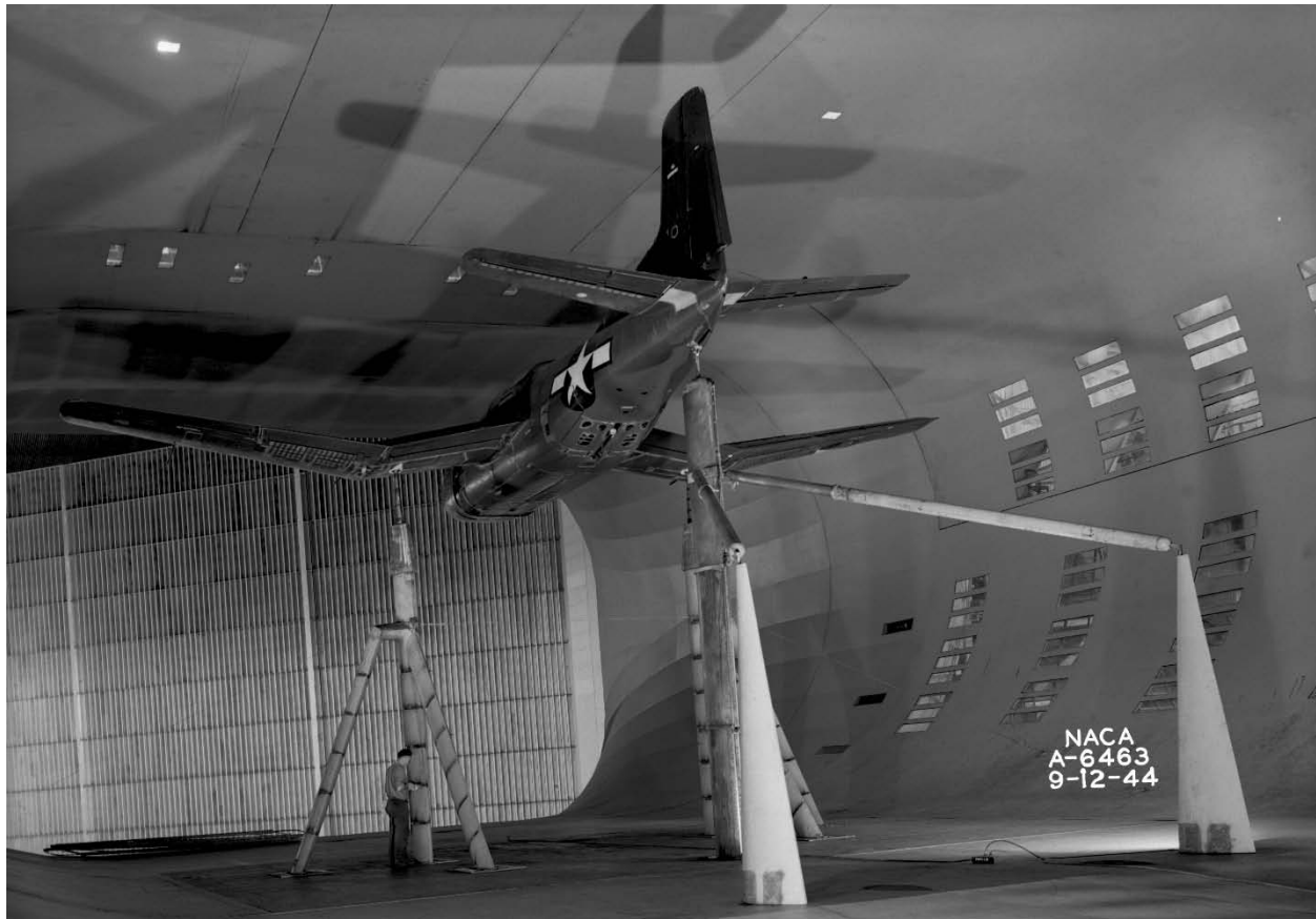
Figure 62. Rear view of the Douglas BTD-1; the two telescoping tail-strut support struts are shown. (NACA A-6463)
