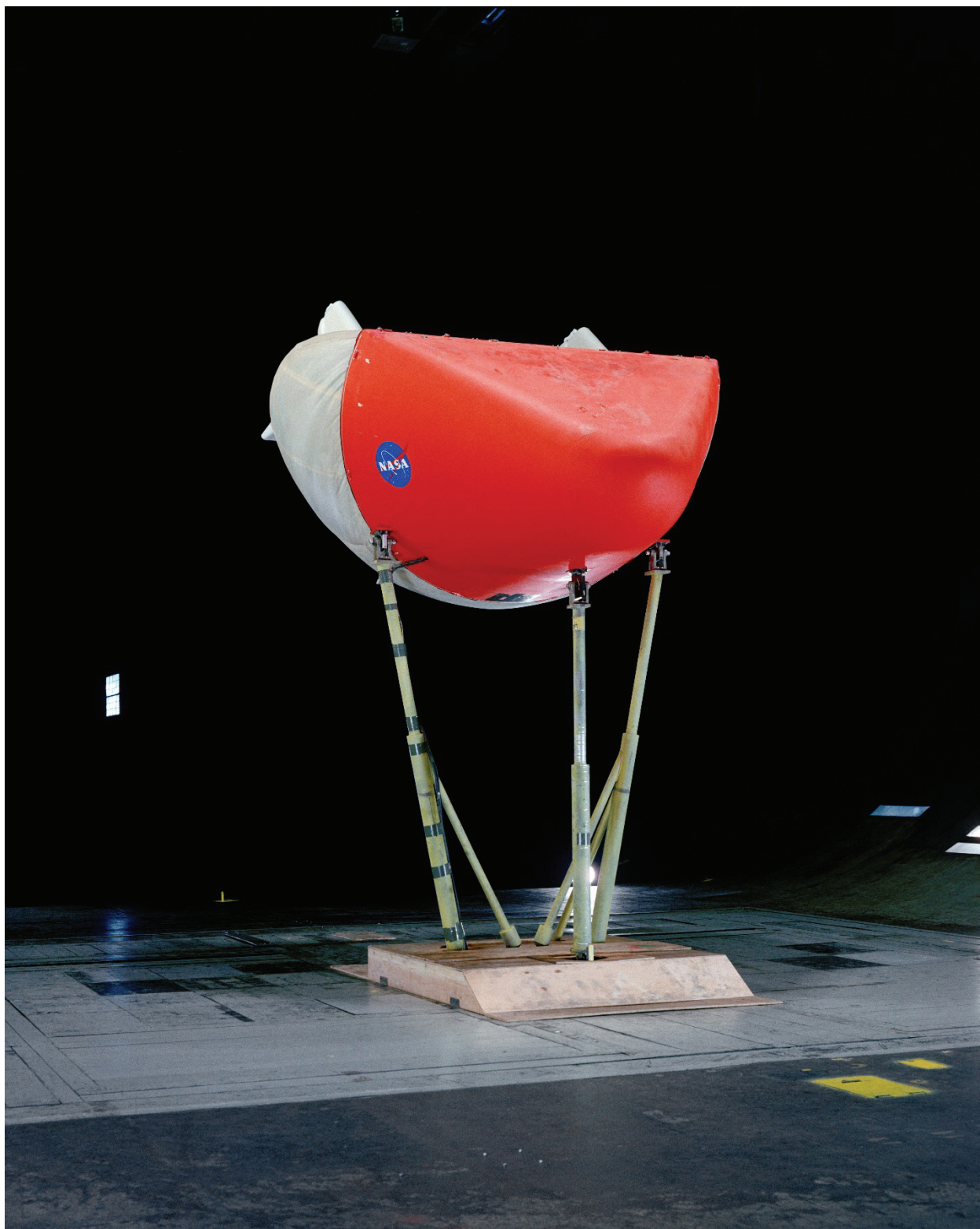
Figure 228. Three-quarter front view of M1-L lifting-body model with inflatable afterbody. (NASA A-35755)
