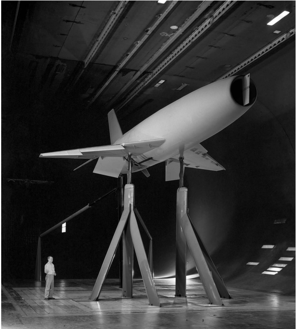
Figure 94. Follow-on experiments of F-4 model wing with flaps and BLC but with a different fuselage. Empennage with drooped horizontal tail; flaps and slats down. Engineer Leo Hall in photo. (NACA A-22148)
