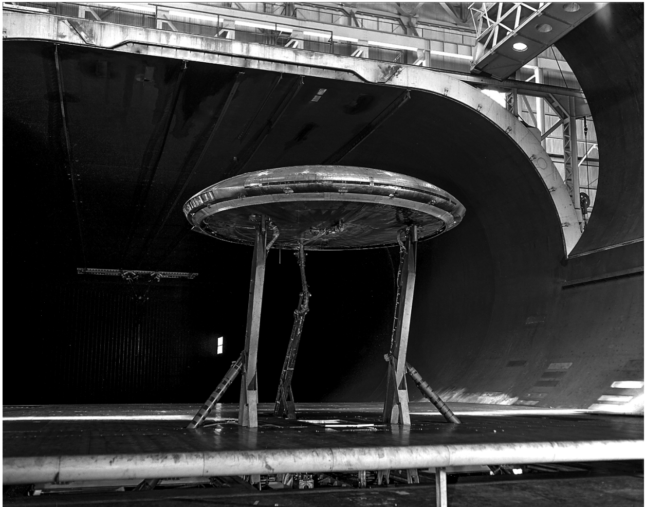
Figure 150. Three-quarter front view of the Avrocar flying saucer on variable-height support struts. (NASA A-27748)
