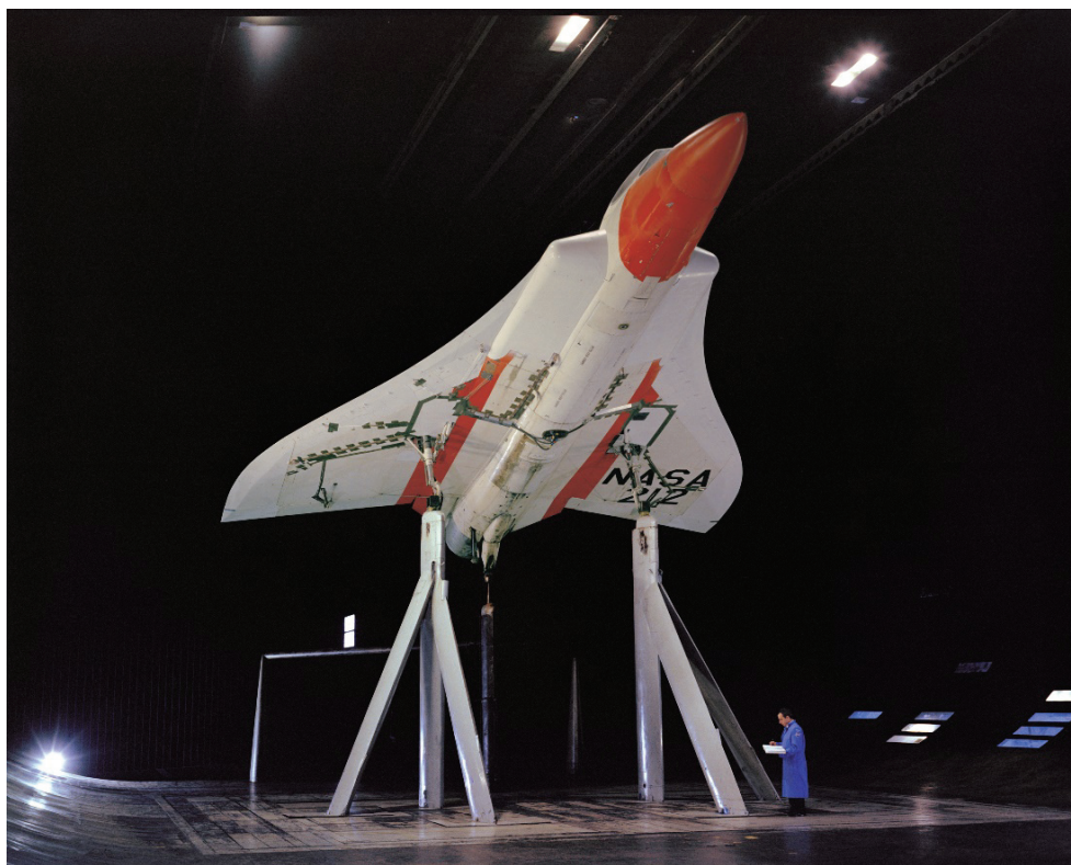
Figure 128. Front lower view of Douglas F5D-1 aircraft with ogee-shaped wing; the wing was modified to simulate a Concorde SST wing. (NASA AC-31304)
