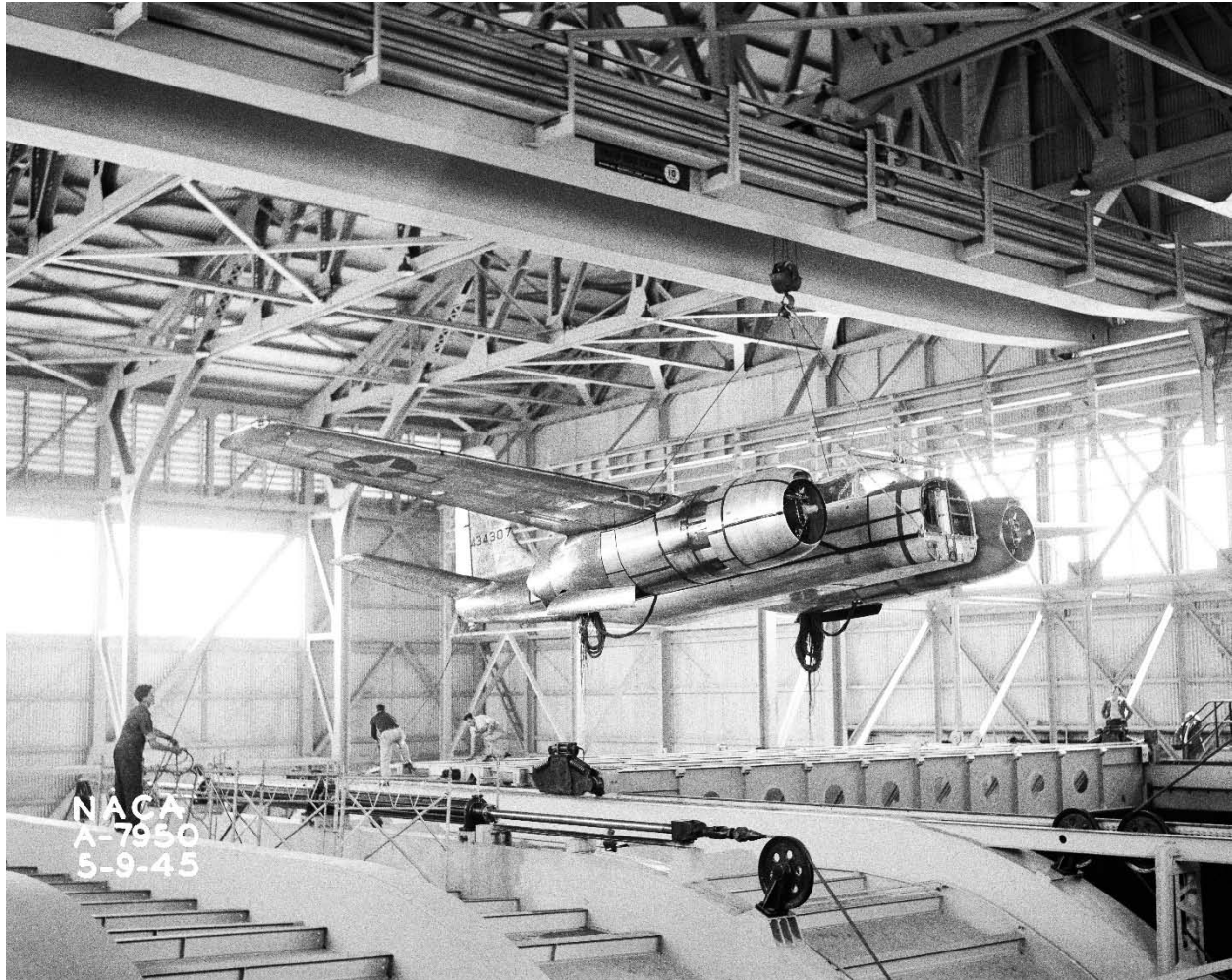
Figure 65. Douglas A-26 attack bomber being lifted into the tunnel without its fuselage nose and propellers. The aircraft is above the test section in this view. ( NACA A-7950 )
