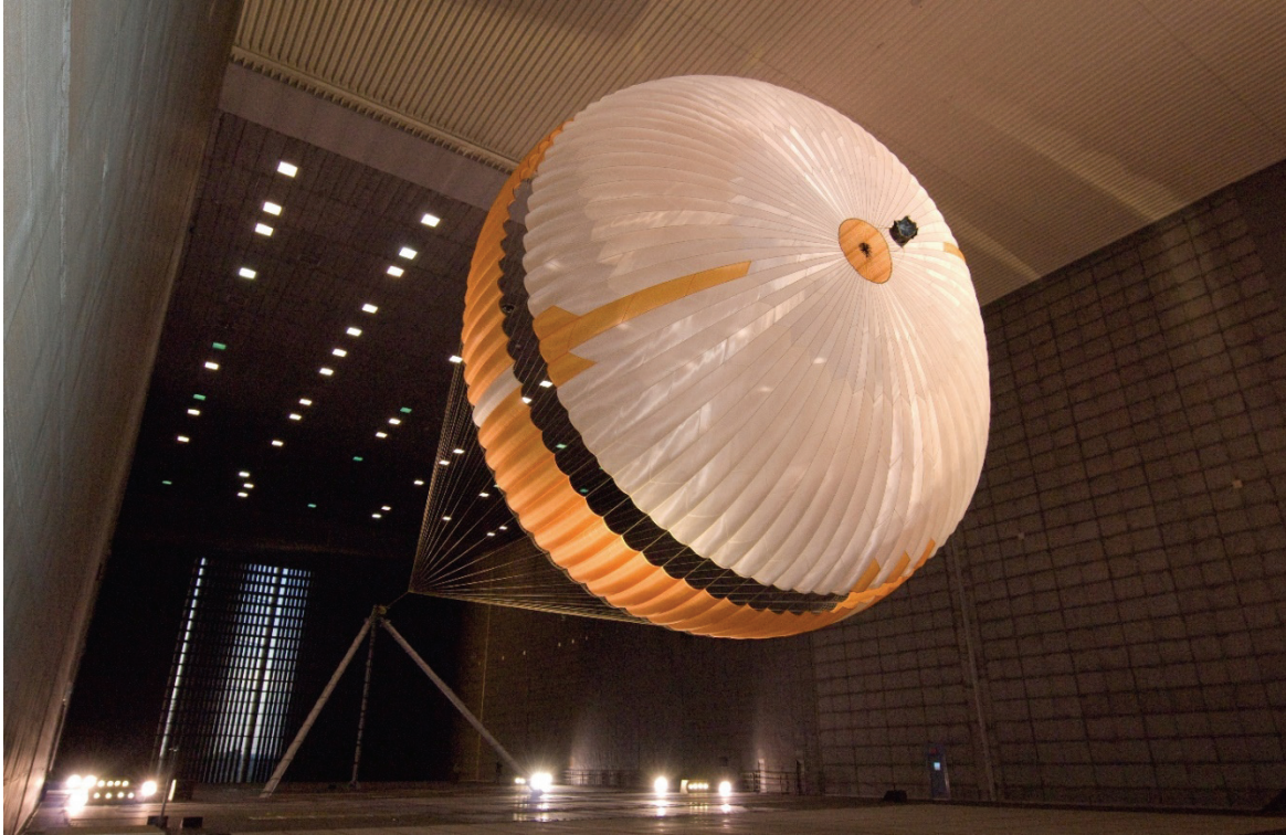
Figure 269. MSL parachute attached to a custom support in the 80- by 120-foot test section. (MSL_D2009_0331_TO164)
