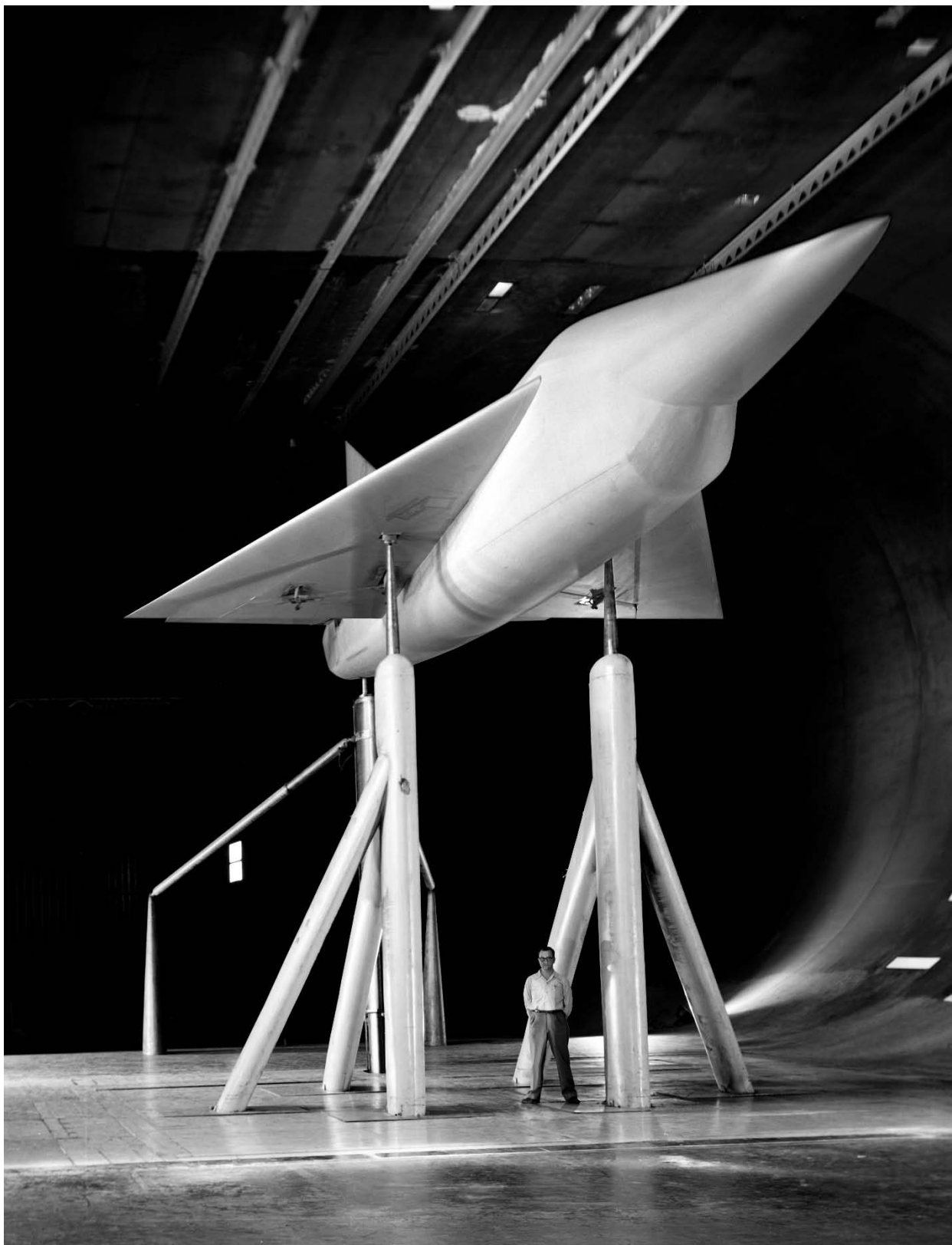
Figure 91. Three-quarter front view of model with an aspect-ratio-2 variable-incidence triangular wing on the fuselage with a vertical tail. Engineer William T. Evans in photo. ( NACA A-17102 )
