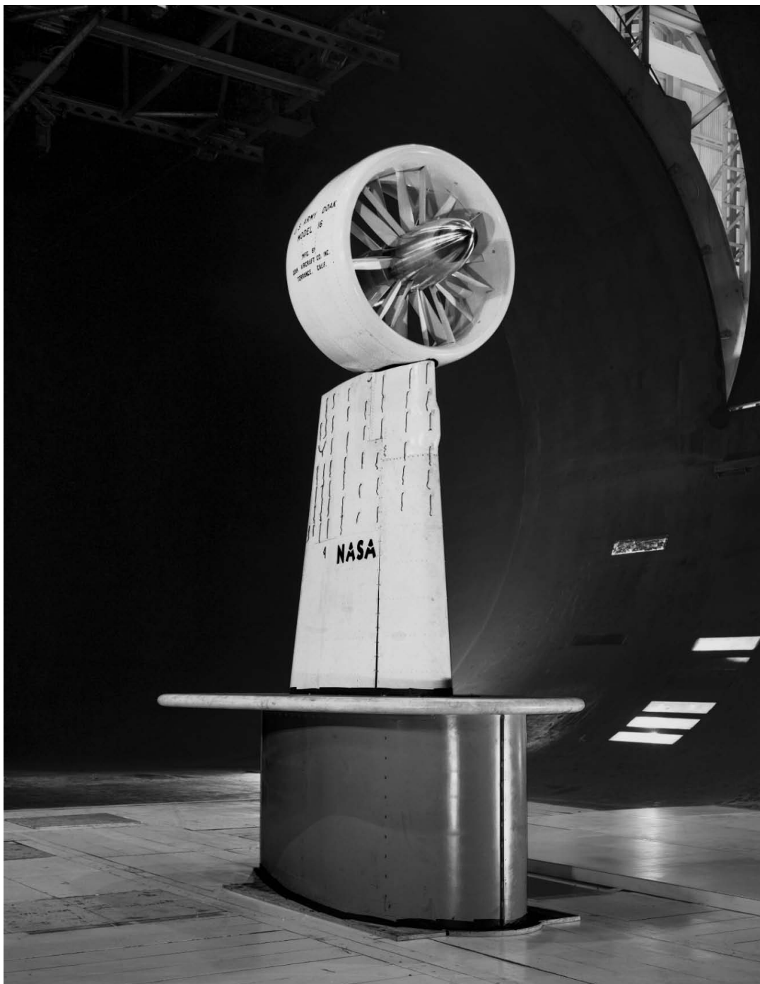
Figure 178. Doak VZ-4DA 4-foot-diameter ducted-fan semispan model. (NASA A-25140)
