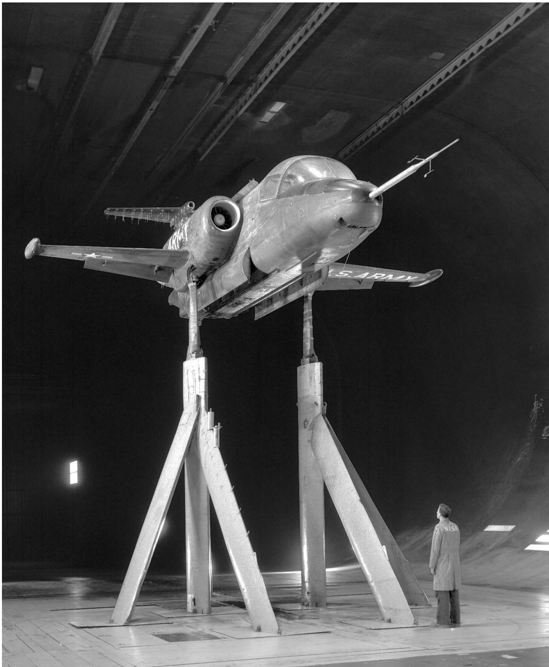
Figure 208. Three-quarter front view of the Lockheed XV-4A Hummingbird experimental jet-ejector augmentor VTOL aircraft. The augmentors were in the fuselage; open augmentor exhaust doors are shown. (NASA A-33194)
