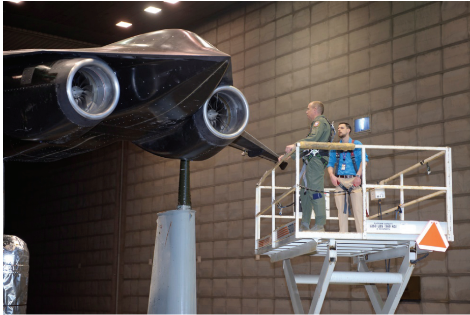
Figure 252. SACD 23-percent-scale model in the 80- by 120-foot test section. (110715-F-UU070-014)
