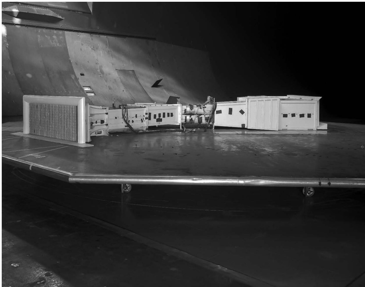
Figure 30. Side view of NFAC wind tunnel model in the 40- by 80-foot test section mounted on a ground board. Inlet for the 80- by 120-foot test section on the left and drive in the center. (NASA A76-0634)
