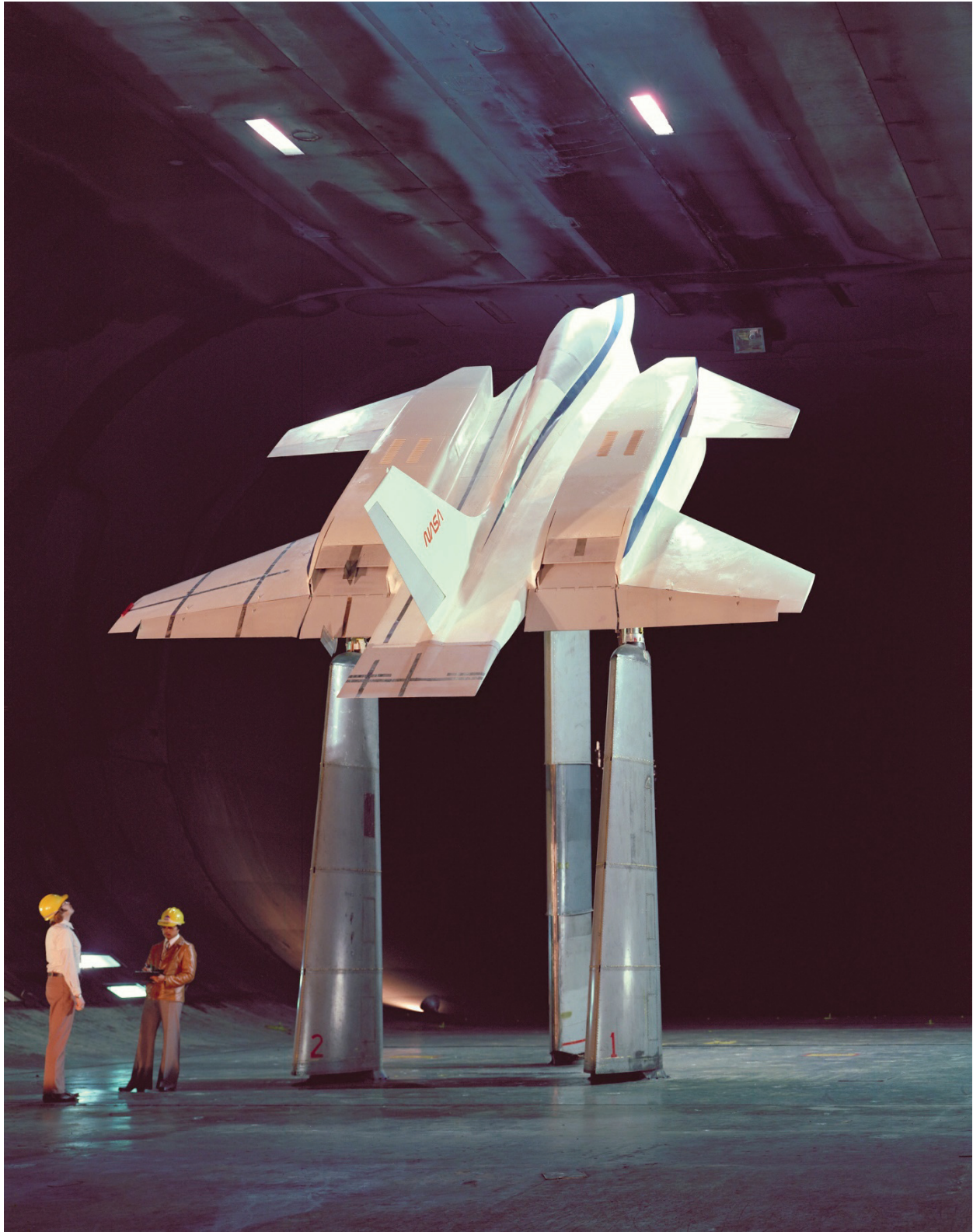
Figure 175. Three-quarter rear view of a highly maneuverable, supersonic V/STOL fighter model. (NASA AC79-0110-2)
