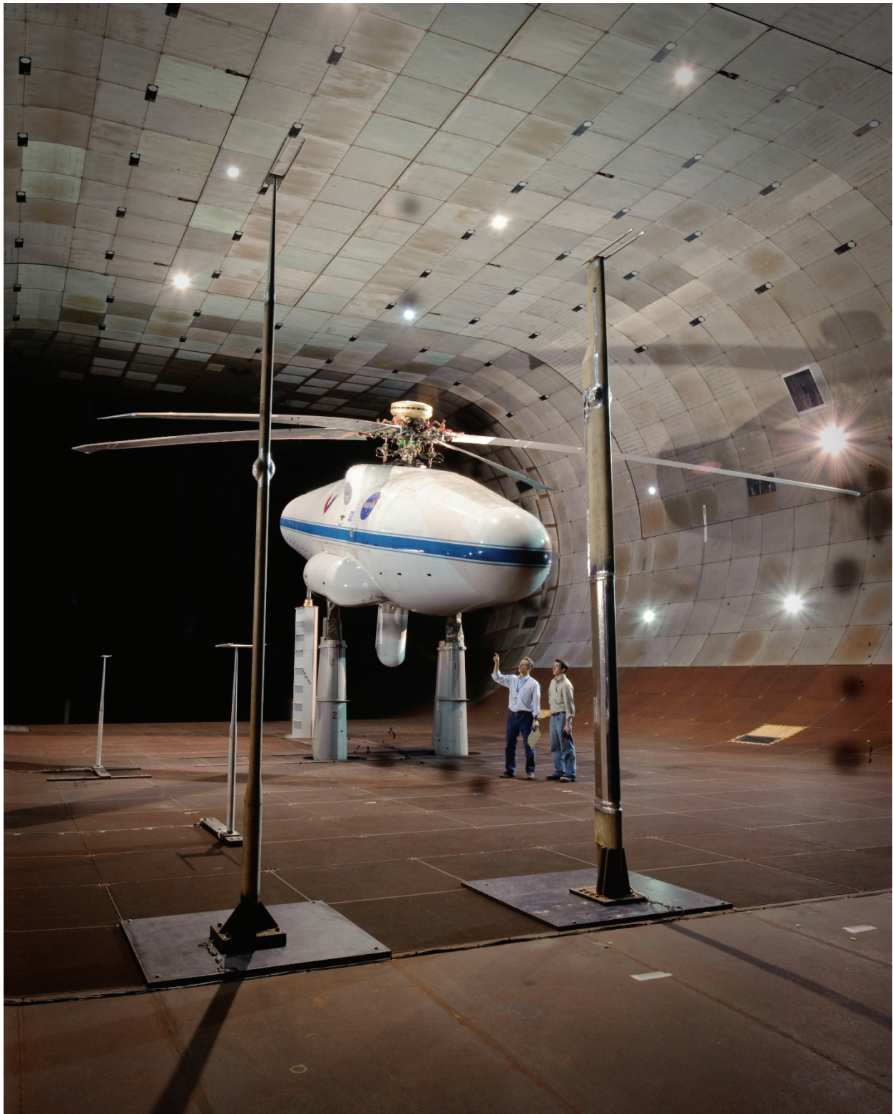
Figure 247. Sikorsky UH-60 helicopter rotor in the 40- by 80-foot test section for high-speed testing. (NASA ACD09-0020-006)
