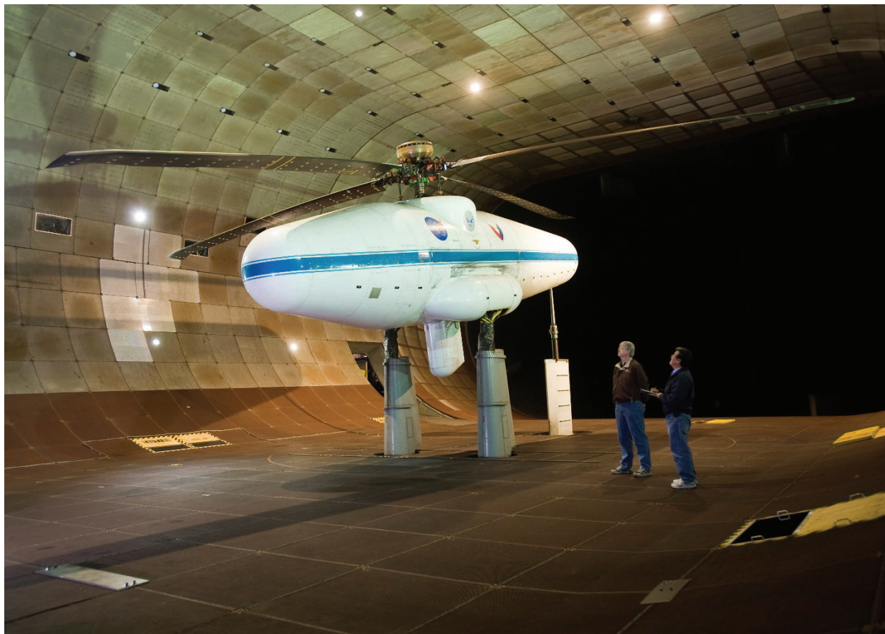
Figure 248. UH-60A main rotor on the LRTA in the 40- by 80-Foot Wind Tunnel for airloads test. (NASA ACD10-0087-004)
