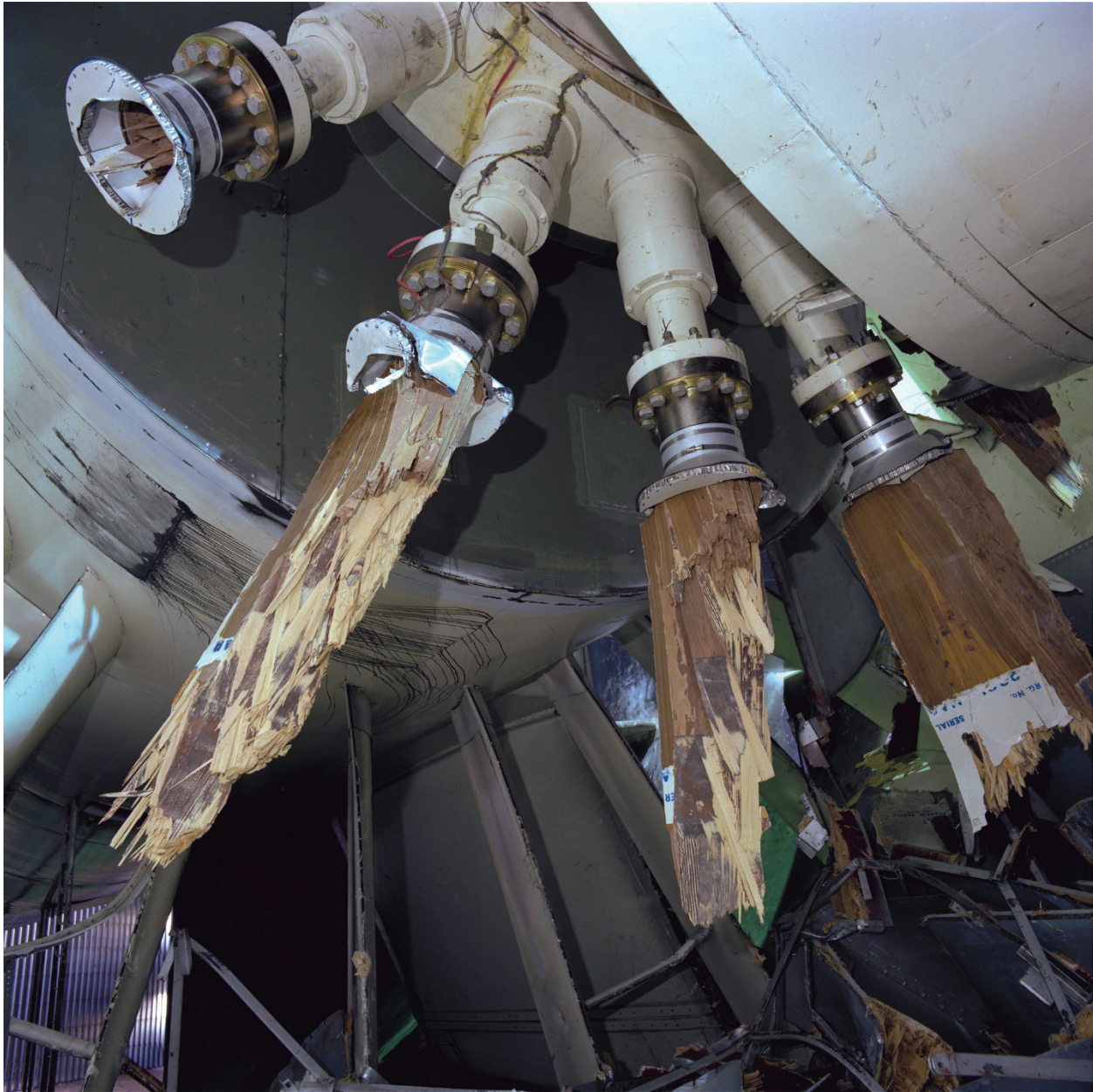
Figure 54. Results of the 1982 accident showing fan blade destruction. (NASA AC82-0875-155)
