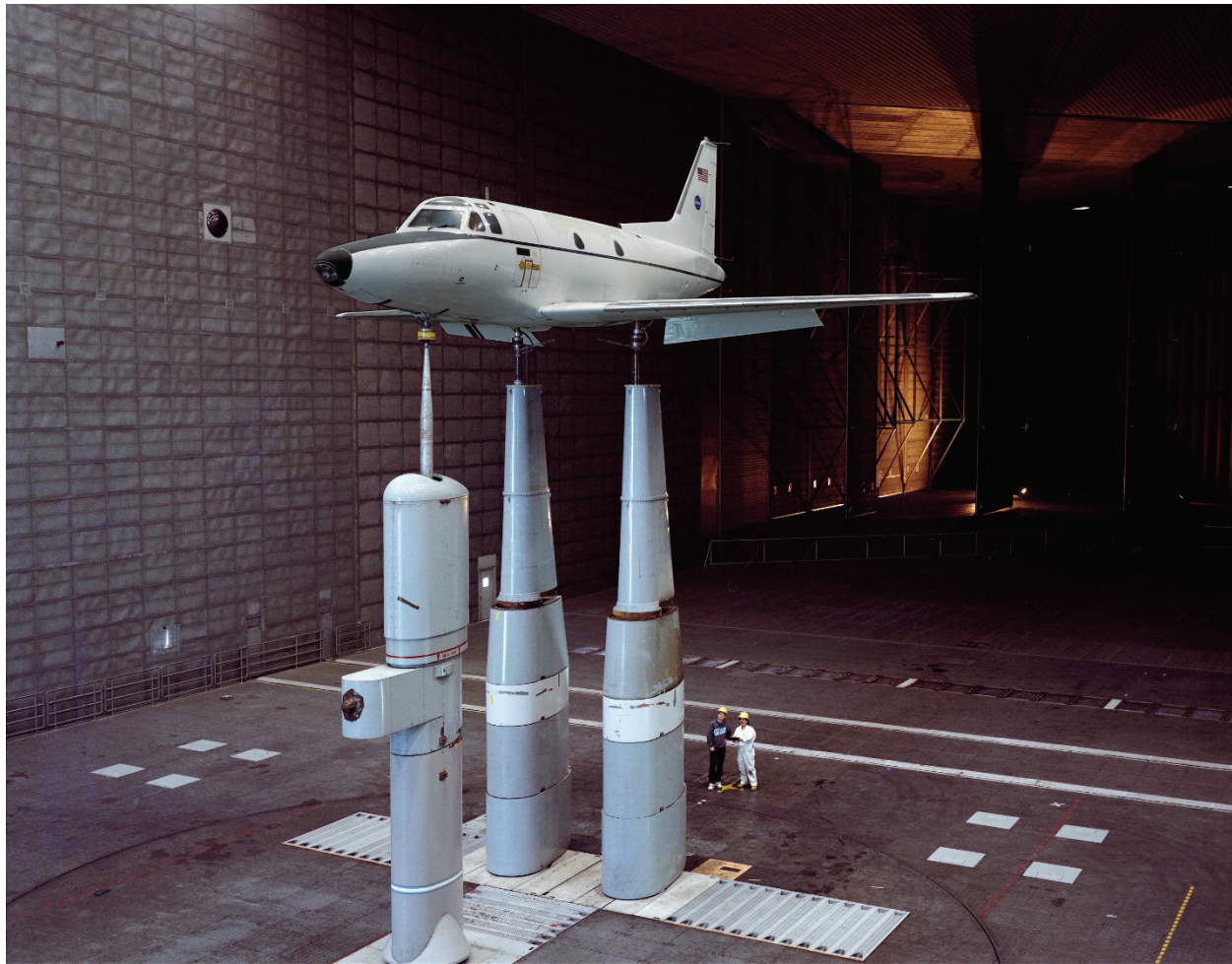
Figure 264. Three-quarter front view of the North American T-39 Sabreliner in 80- by 120-foot test section for high-lift research. (NASA AC93-0233-2)
