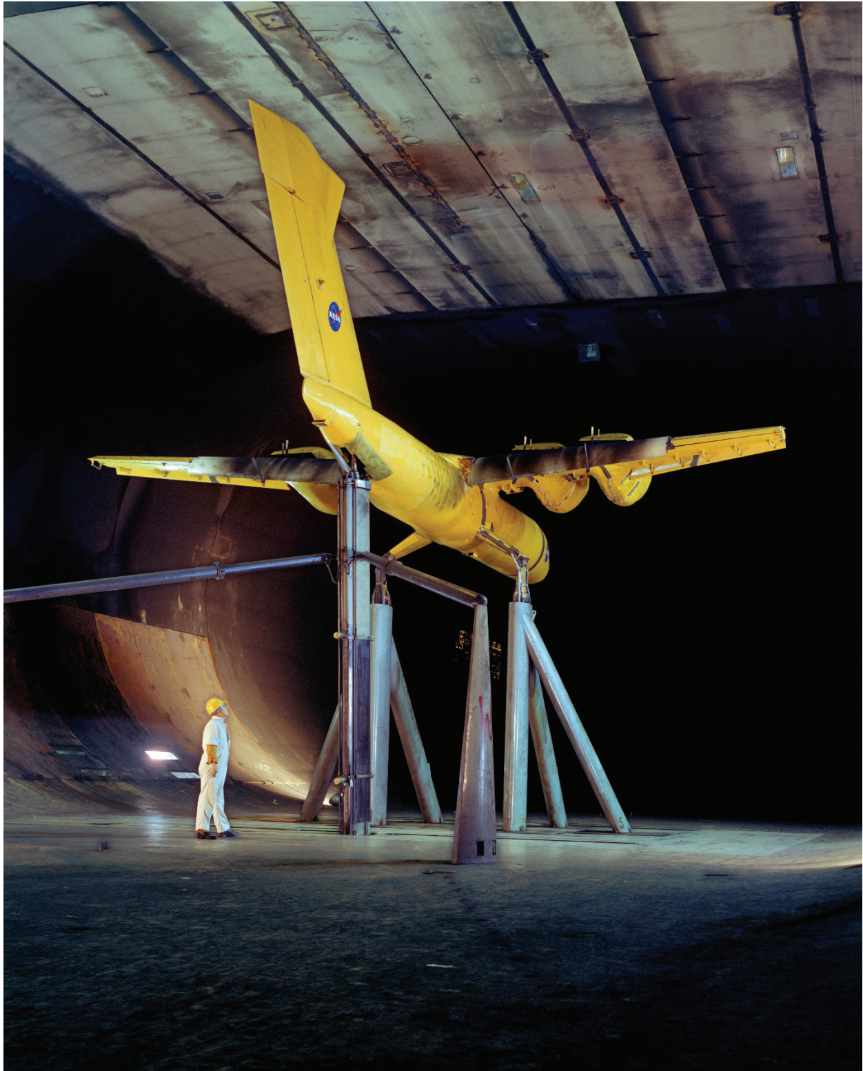
Figure 219. Rear view of USB model with four jet engines. ( NASA AC74-0958 )
