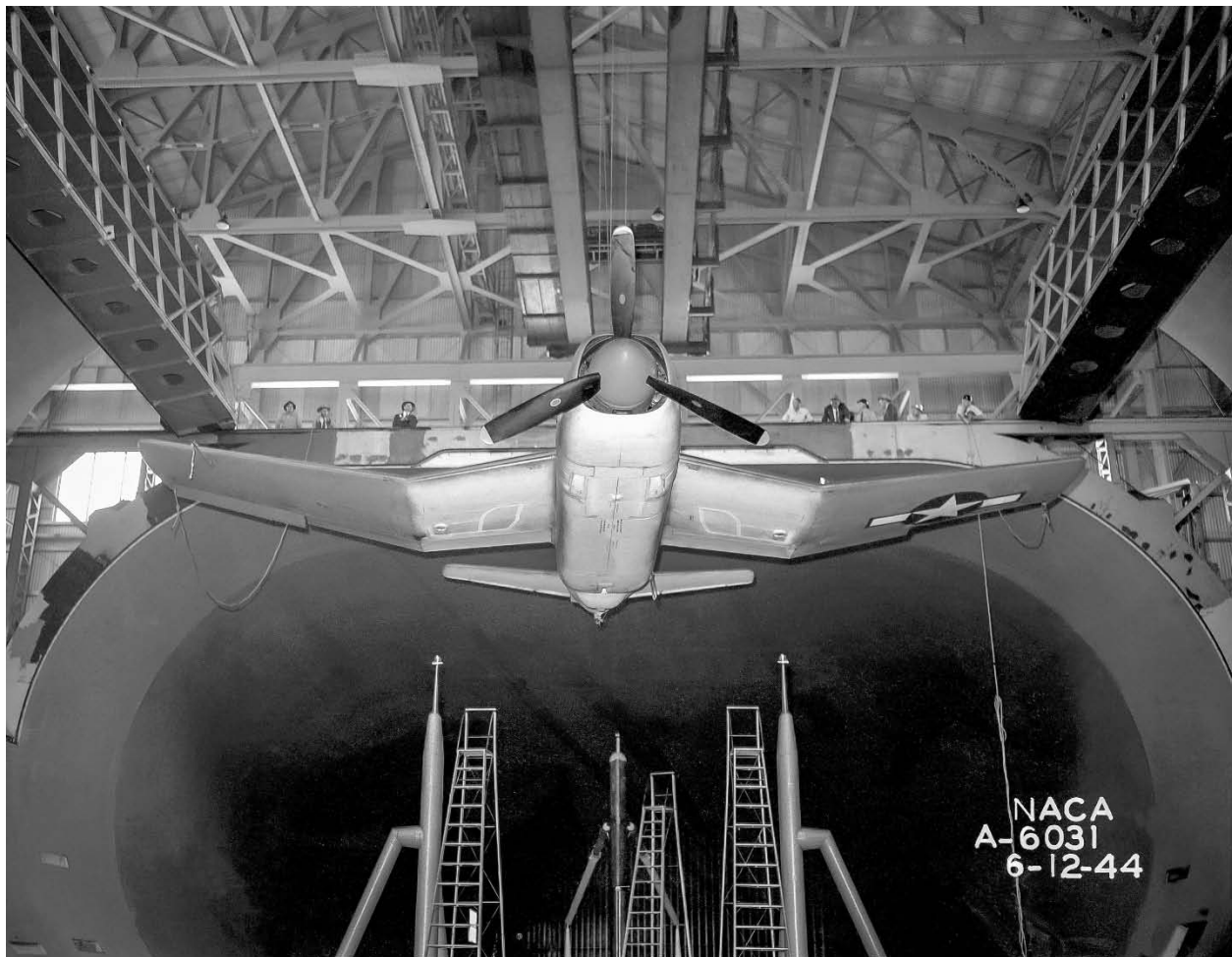
Figure 59. The first airplane tested in the 40- by 80-Foot Wind Tunnel was a Douglas XSB2D-1; it is shown being lowered into the test section on June 12, 1944. The edge of the overhead doors can be seen. This was a so-called gull-wing aircraft. ( NACA A-6031 )
