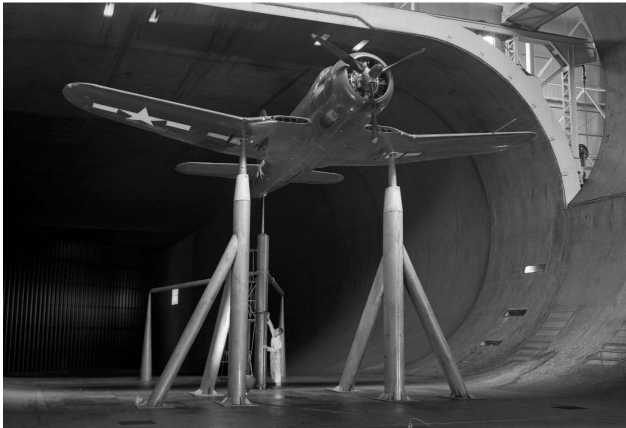
Figure 78. Ryan FR-1 Fireball experimental aircraft intended for carrier operations using both propeller and jet-engine thrust. The jet-engine inlets are at the wing roots next to the fuselage. The overhead doors are still open. (NACA A-7309)
