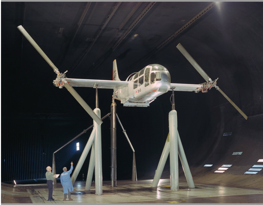
Figure 133. Bell XV-3 tilt-rotor aircraft with two-bladed proprotors in forward-flight mode. (NASA A-37006-5)
