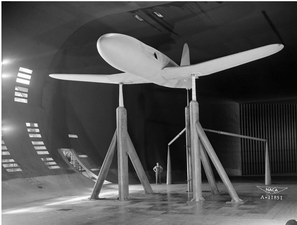
Figure 80. Submerged jet-engine inlet model in tunnel. The inlet is shown in the fuselage above the leading edge of the wing. (NACA A-11851)
