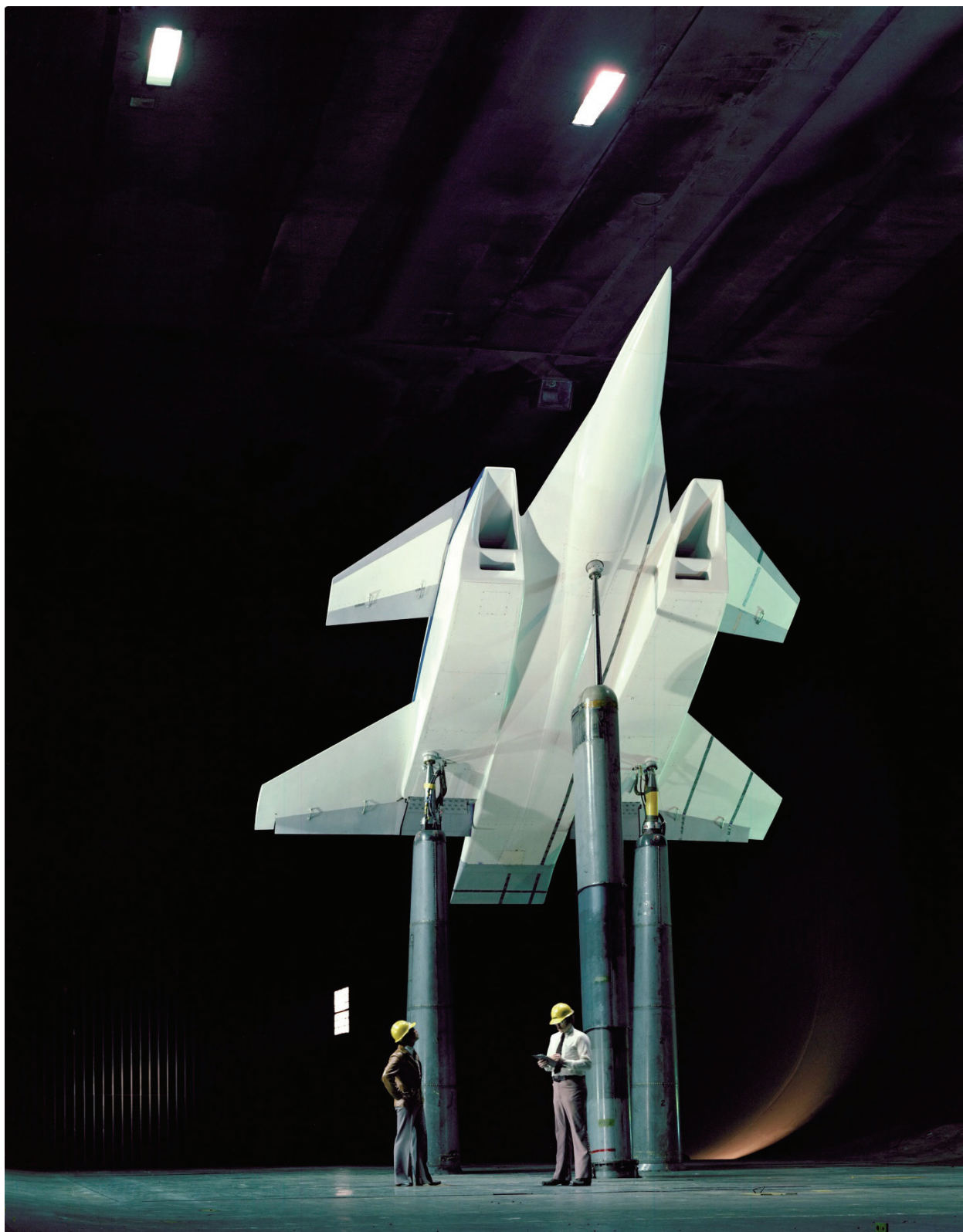
Figure 174. Three-quarter front view of a highly maneuverable, supersonic V/STOL fighter model. (NASA AC79-0110-1)
