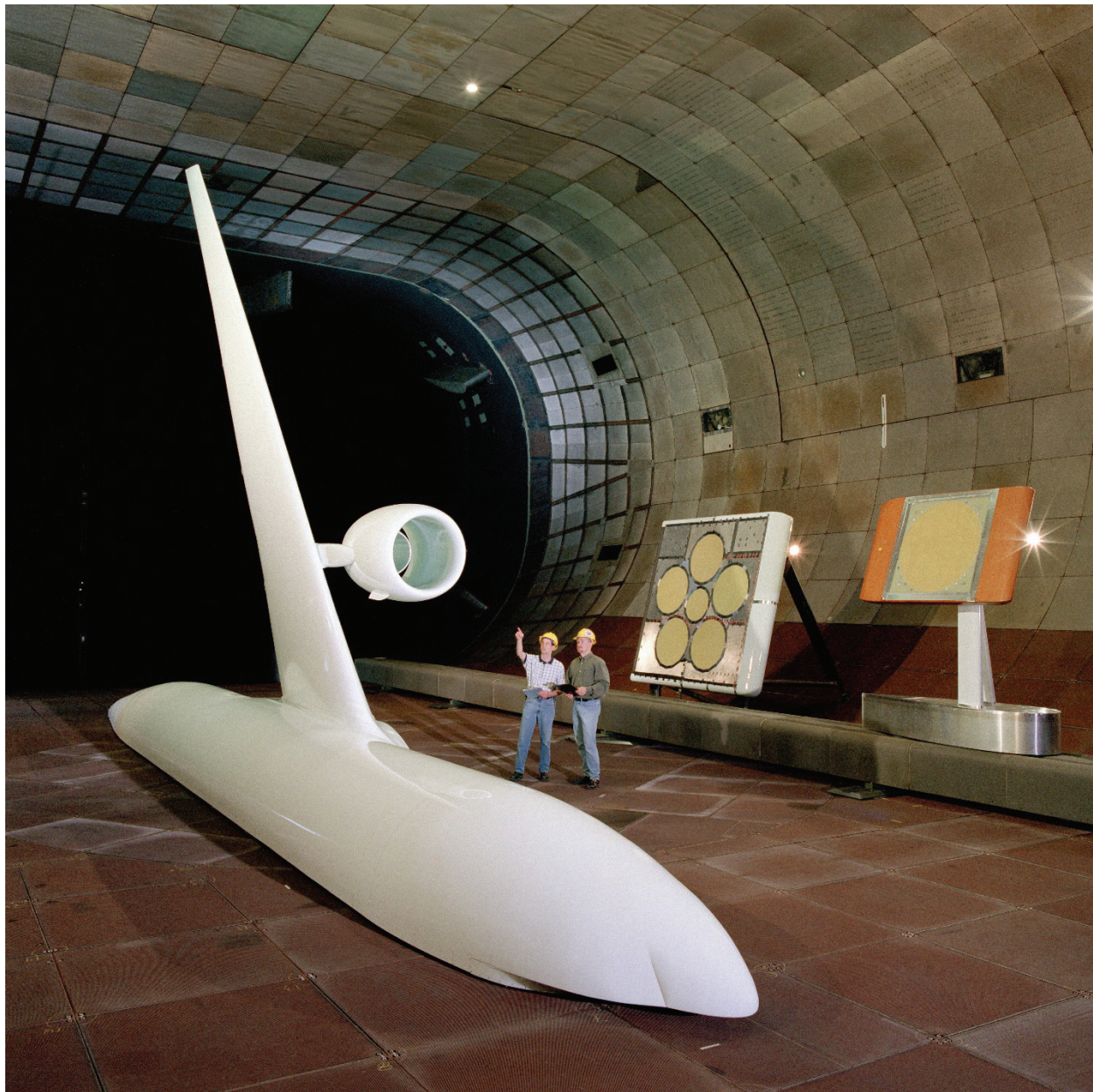
Figure 275. A 26-percent-scale semispan model of a Boeing 777. ( NASA AC01-0114-116 )
