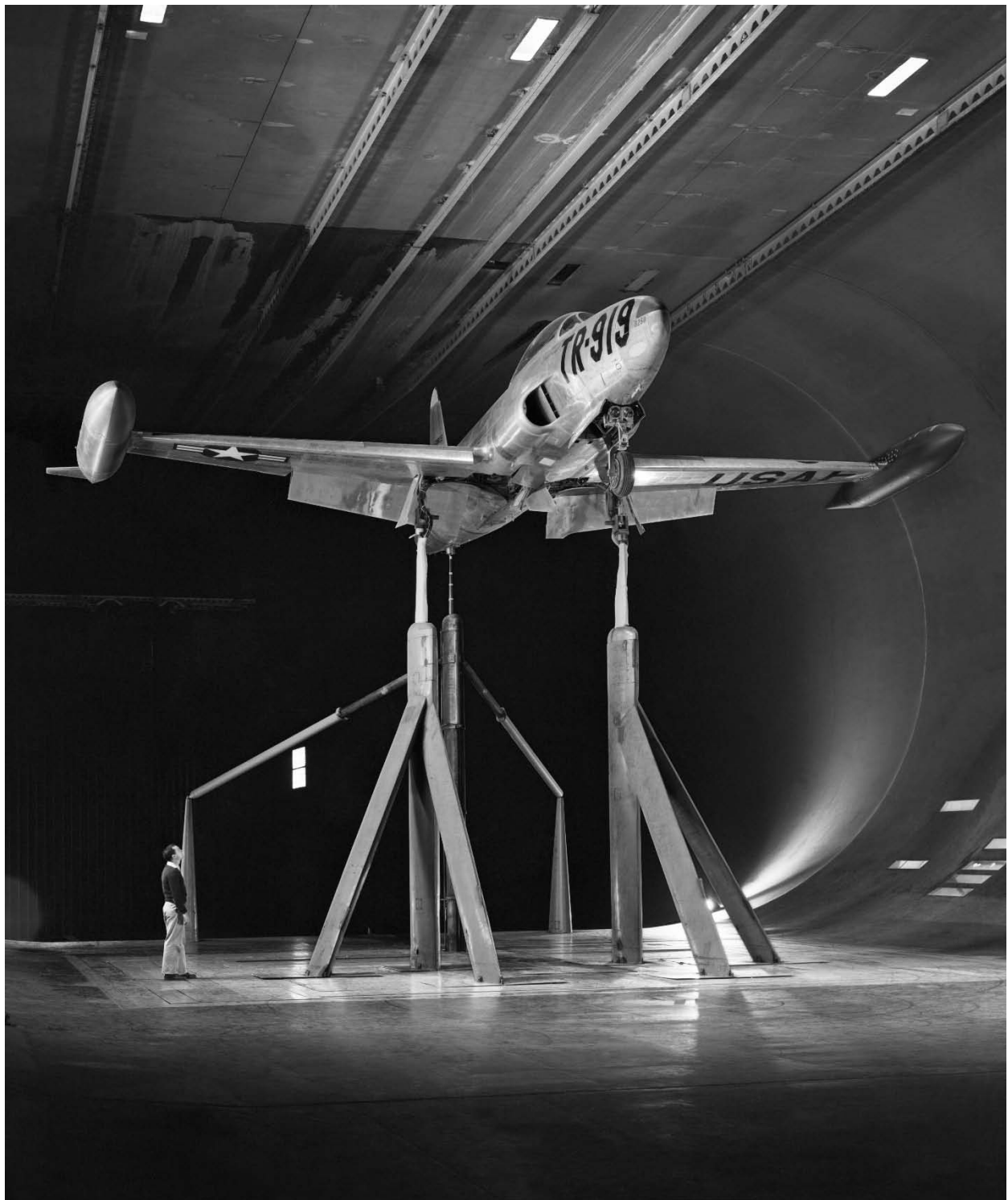
Figure 95. Three-quarter front view of a Lockheed T-33 airplane in the tunnel with BLC on wing. (NACA A-19841)
