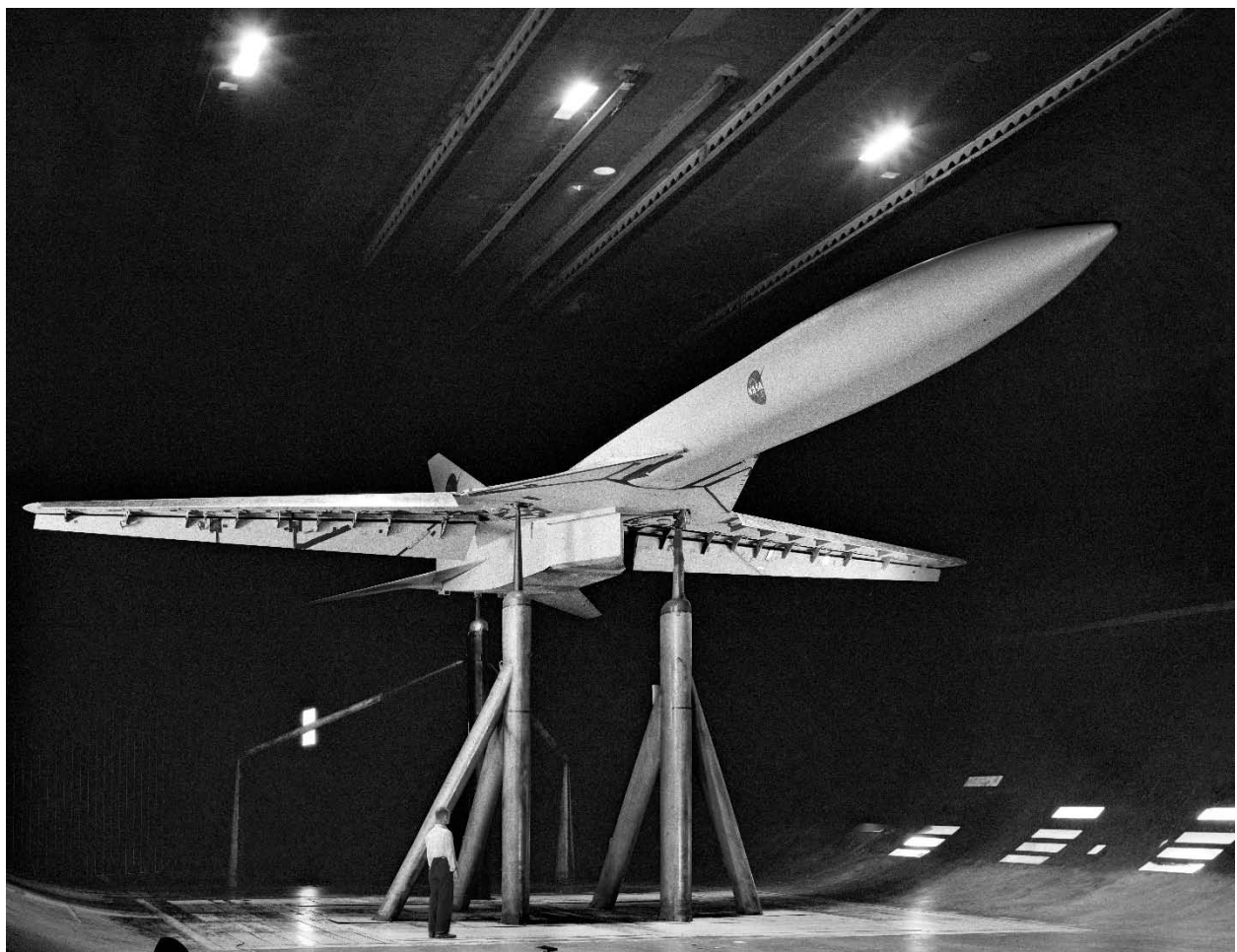
Figure 125. SST model with variable-sweep wings in forward position and engine pod in center underneath. (NASA A-30876)
