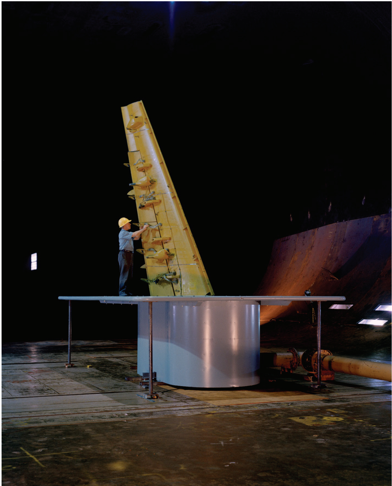
Figure 206. Three-quarter front view of semispan augmentor wing model with Edwin Verrette making model changes. (NASA AC74-1799)
