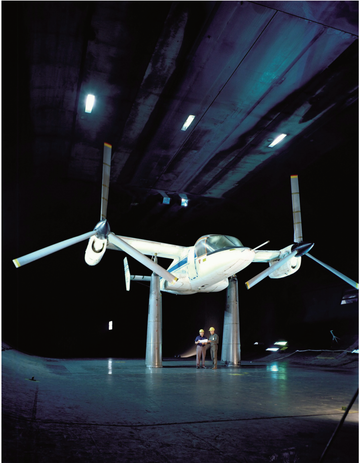
Figure 135. XV-15 tilt-rotor research aircraft in forward flight or cruising mode. (NASA AC78-0579-3)
