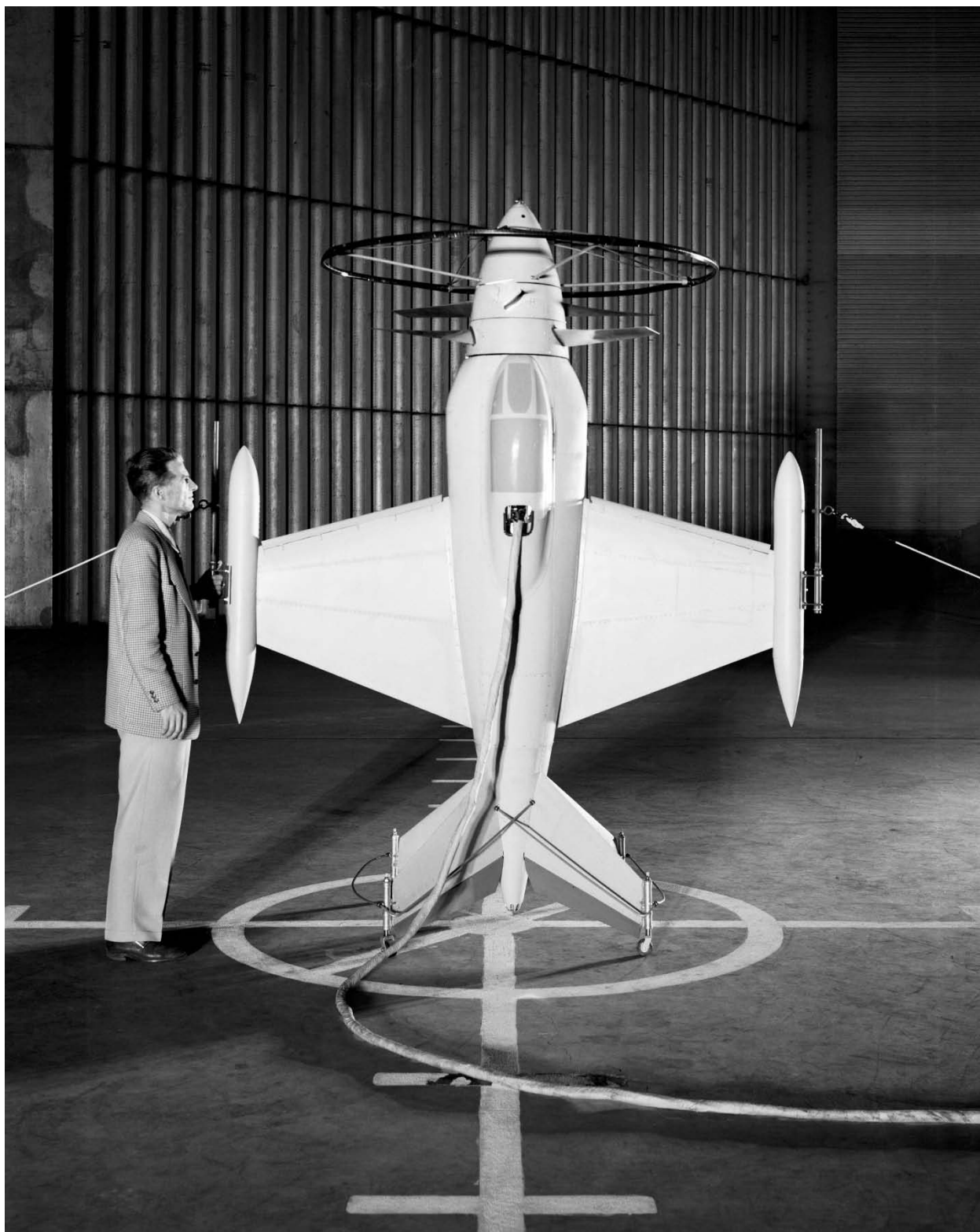
Figure 75. A 1/4-scale Lockheed XFV-1 tail-sitter VTOL airplane model in the settling chamber, which is the largest area of the wind tunnel. ( NACA A-17167 )
