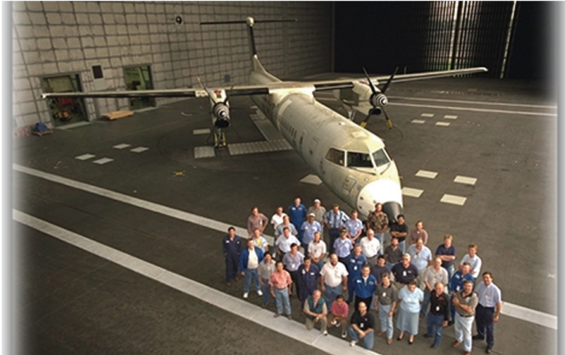
Figure 268. Bombardier Dash 8 Q400 aircraft in the 80- by 120-foot test section with test crew. (J. Sacco collection, DASH 8)
