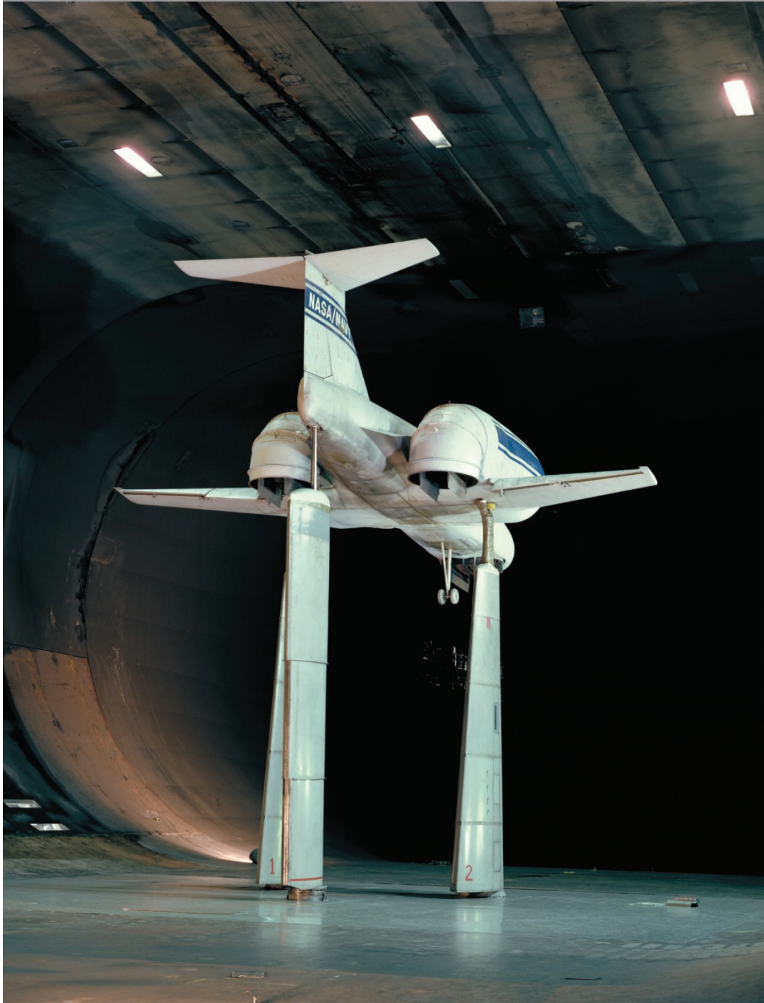
Figure 164. Three-quarter rear view of lift/cruise-fan fighter showing fan nozzle deflected downward. (NASA AC76-1061)
