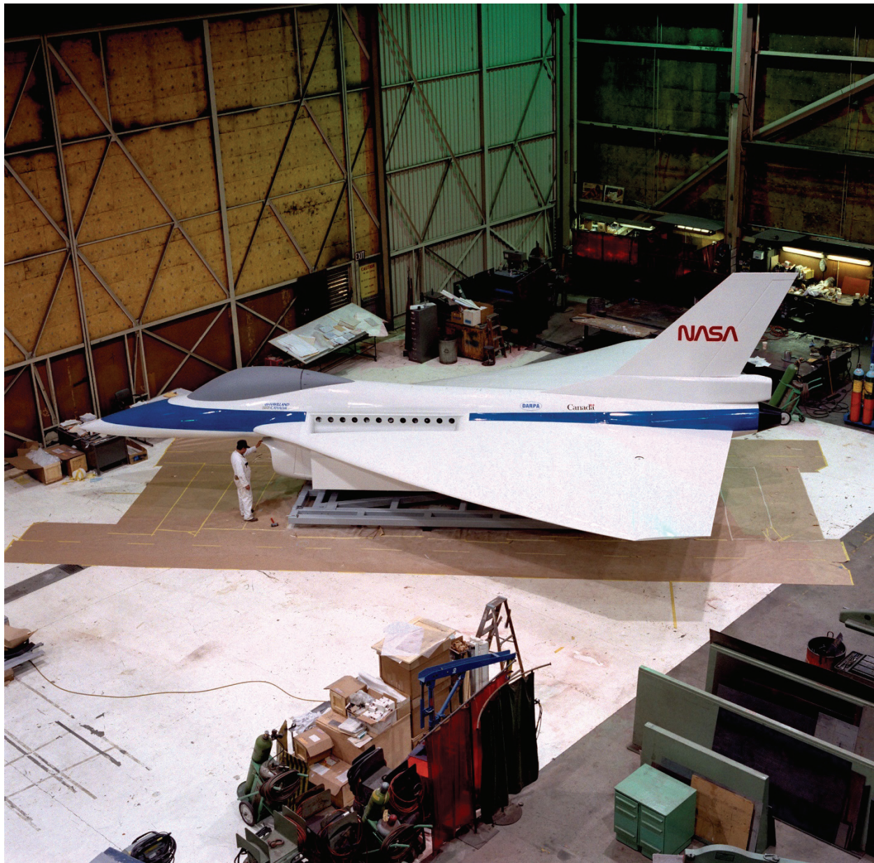
Figure 253. General Dynamics E-7 ejector-lift/vectored-thrust full-scale model in the Ames shop. (NASA AC87-0372-143)
