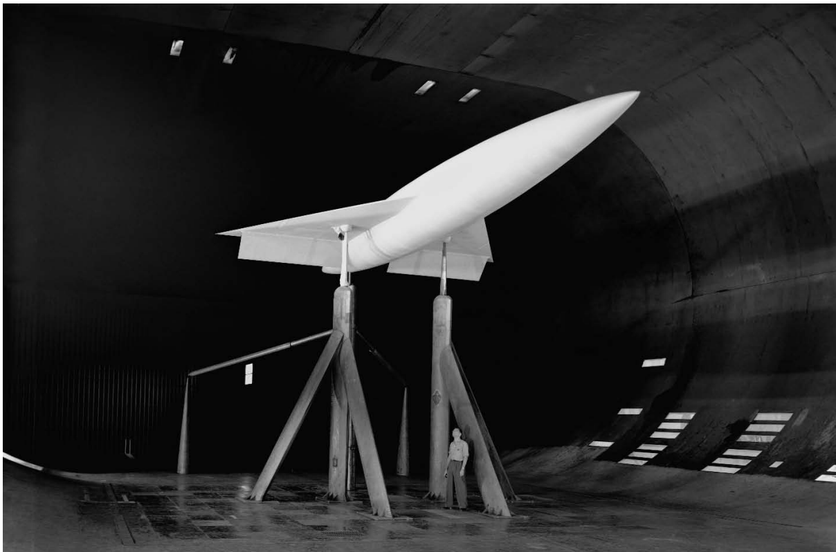
Figure 88. Three-quarter front view of delta-wing model with body and vertical tail; aspect-ratio-2 wing shown with flaps down. (NACA A-11948)
