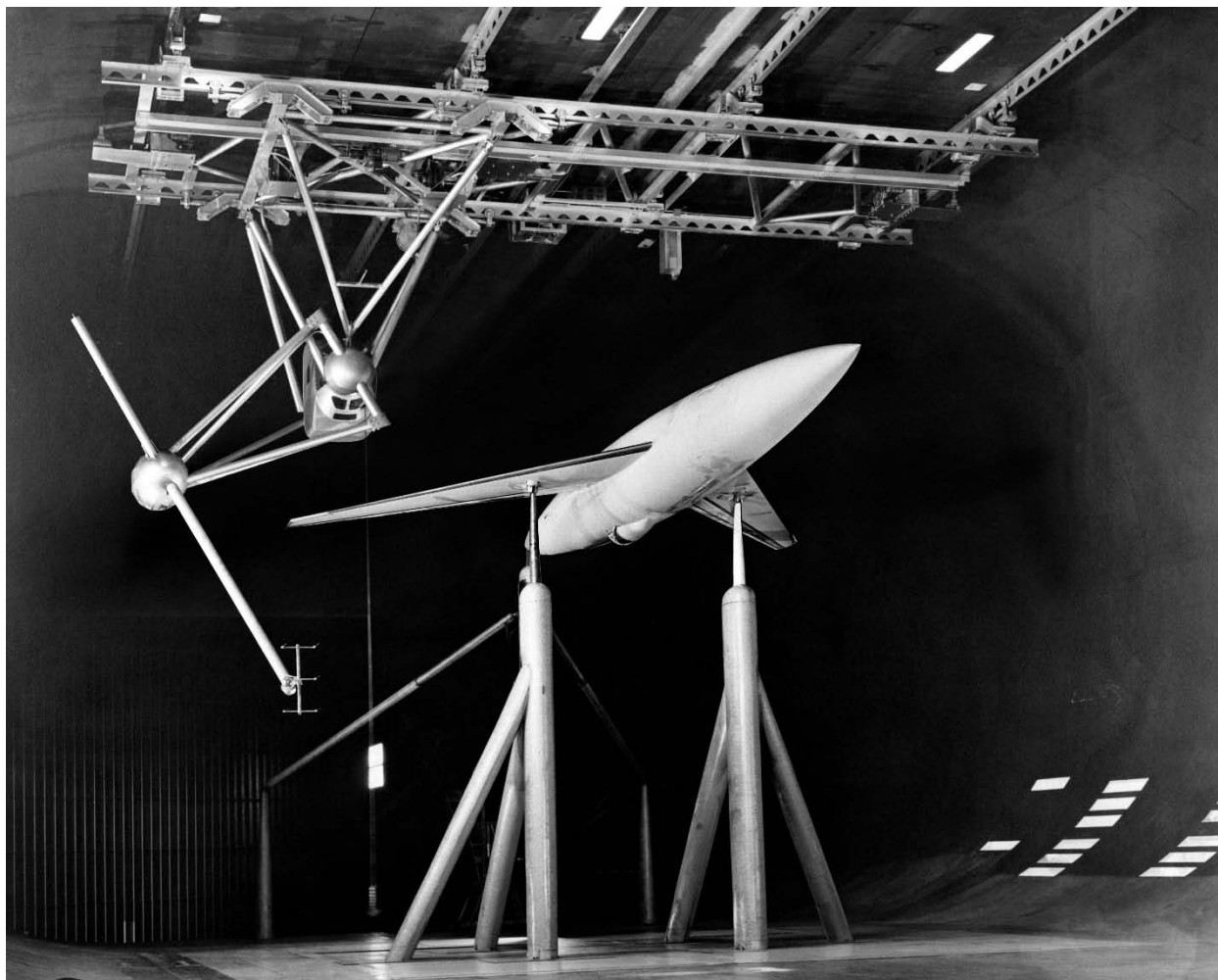
Figure 23. View of 63-degree swept wing with survey rig in the background to the left. ( NACA A-16650 )
