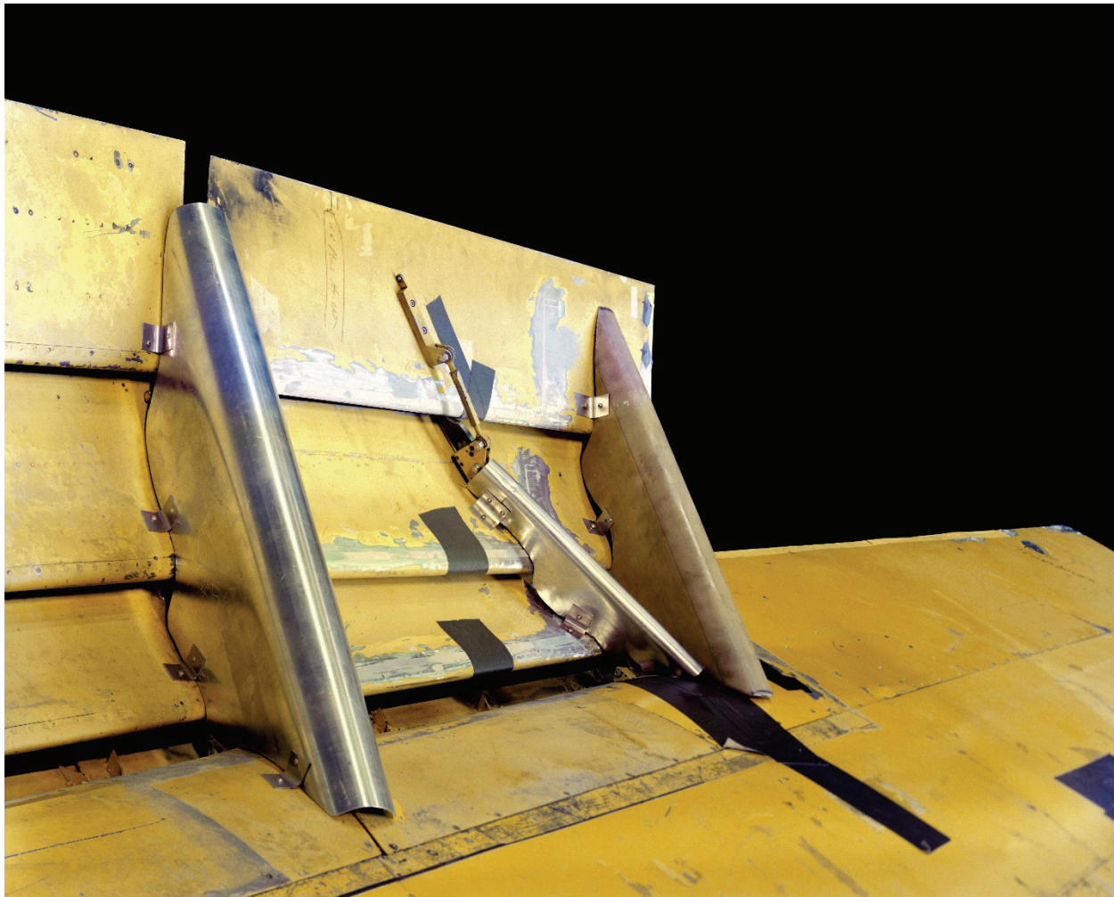
Figure 238. Airframe noise semispan model with close-up of triple-slotted flaps. (NASA78-1062-2)
