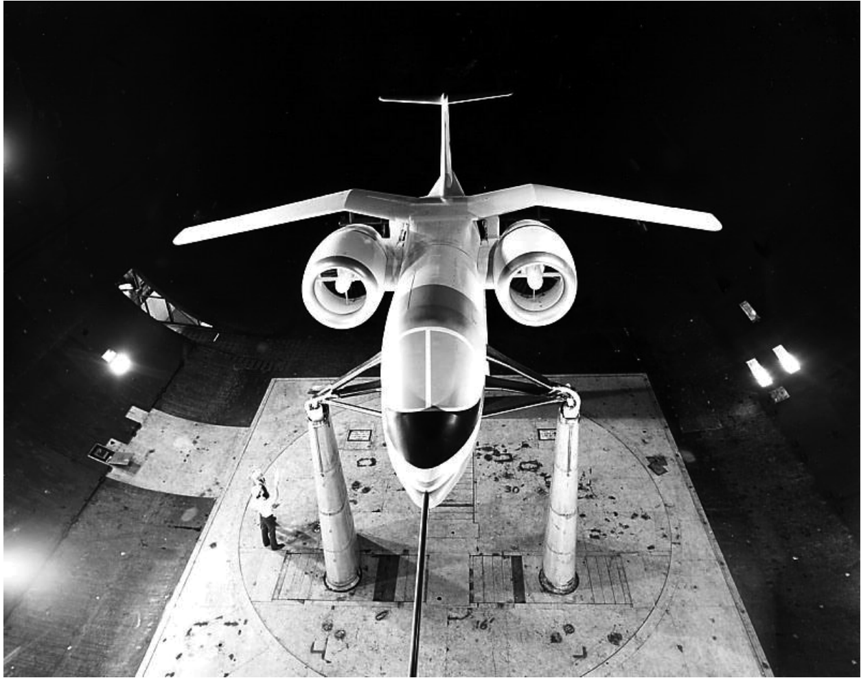
Figure 186. Overhead front view of Grumman 698 tilt-nacelle V/STOL model in the wind tunnel. (J. Sacco collection, gru698_4X80)
