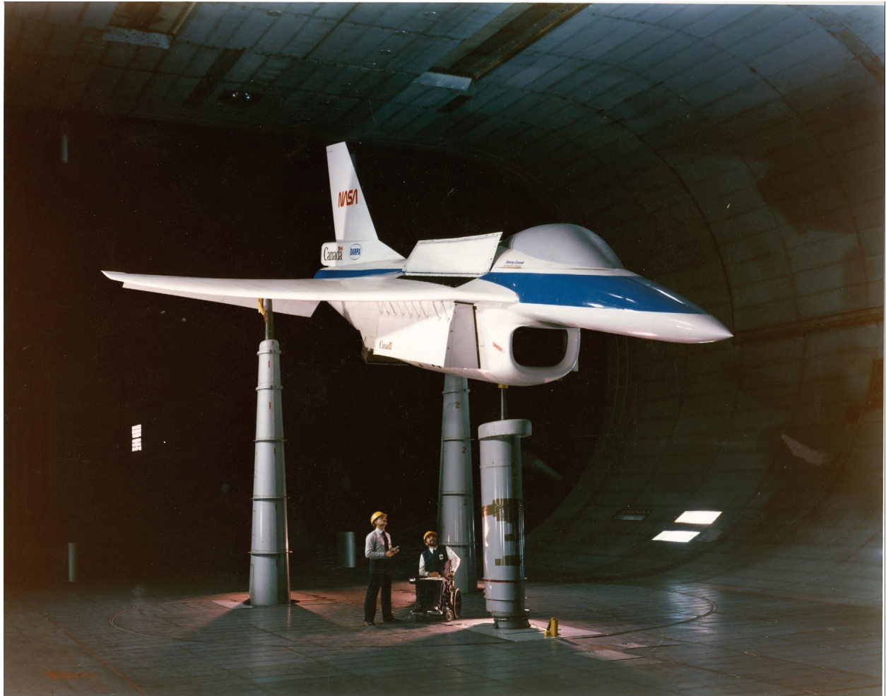
Figure 254. Three-quarter front view of General Dynamics E-7 ejector-lift/vectored-thrust full-scale model. As shown, the ejectors are along the sides of the fuselage and the inlet doors are open. (NASA AC88-0530-28)
