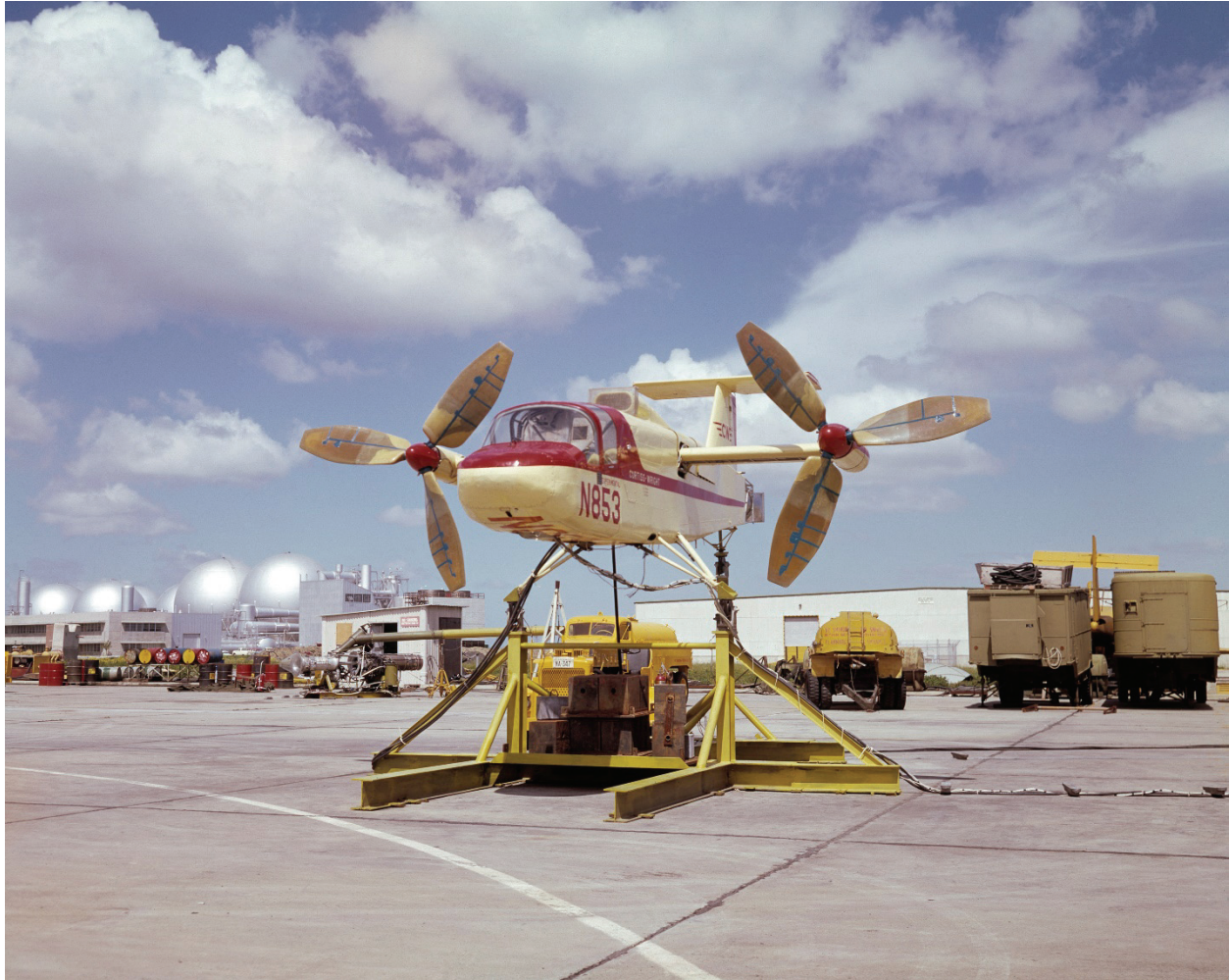
Figure 198. Curtiss-Wright X-100 V/TOL experimental aircraft on flight line for checkout prior to wind tunnel tests. (NASA A-30770)
