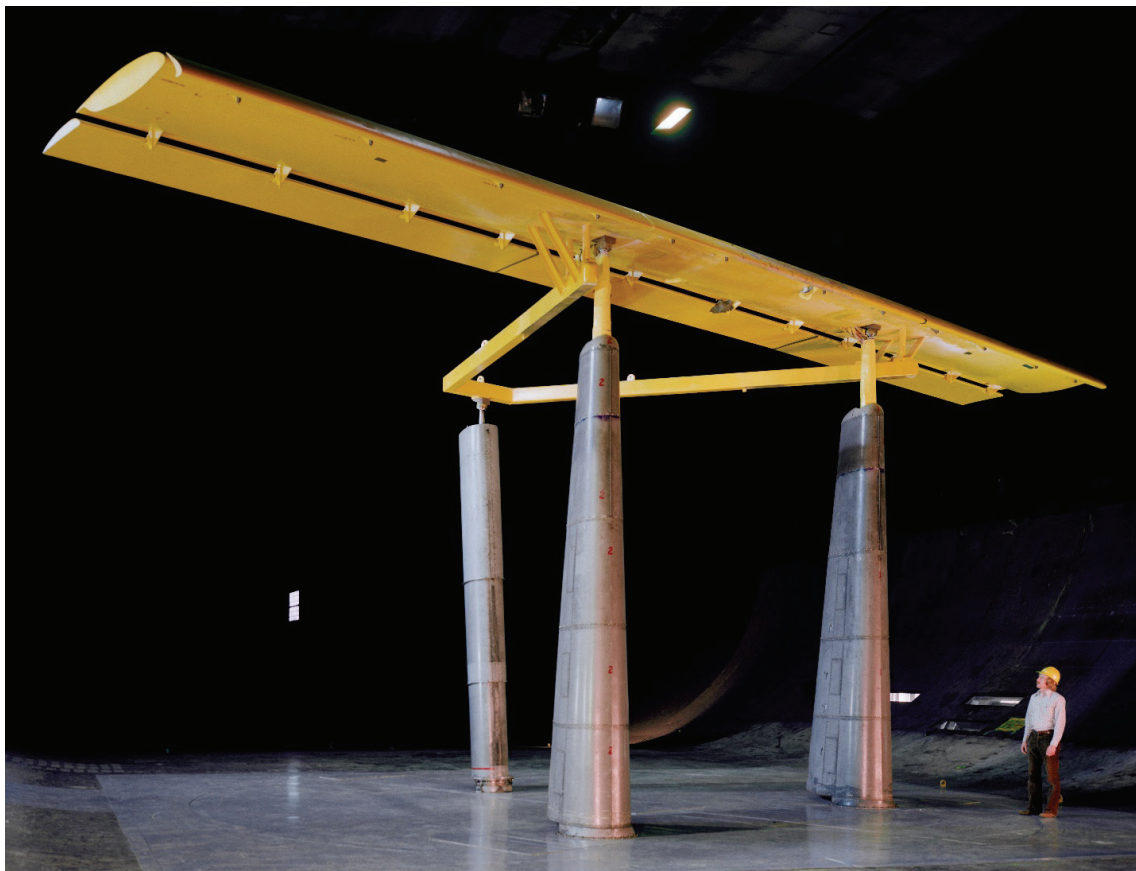
Figure 112. Two-dimensional wing model with a single-slotted flap and a leading-edge slat used for high-lift studies; Mark Betzina in photo. (NASA AC76-0011)
