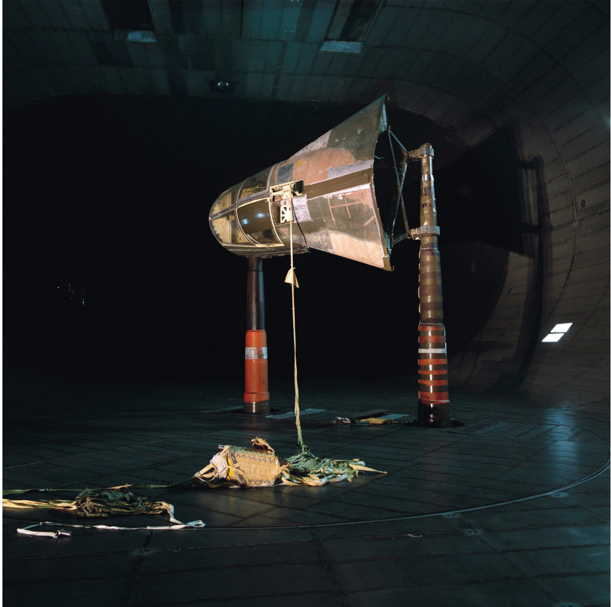
Figure 277. F-111 fighter crew capsule mounted sideways with deployed parachute laying on floor. (NASA AC89-0144-1)
