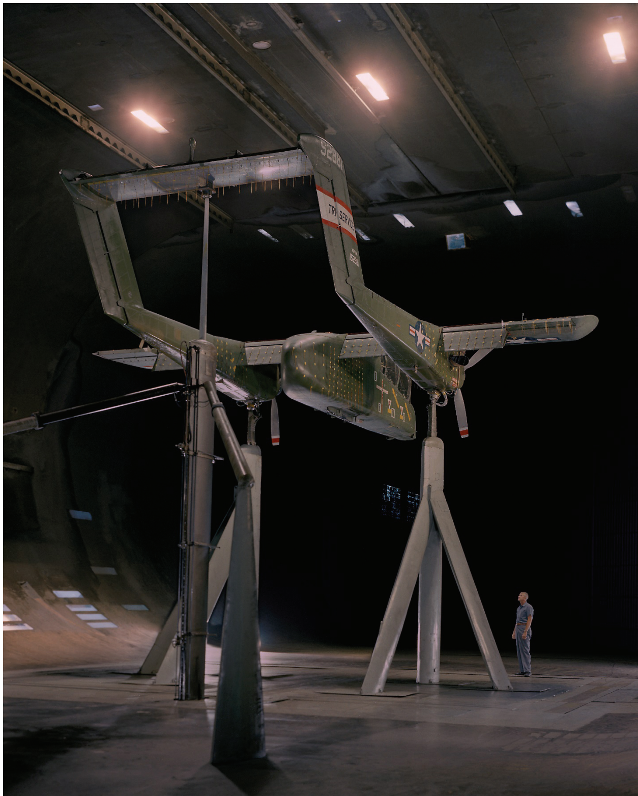
Figure 108. Three-quarter rear view of the North American OV-10 Bronco showing the unusual empennage that allowed up to six paratroopers to jump from the rear fuselage door. (NASA AC-41122)
