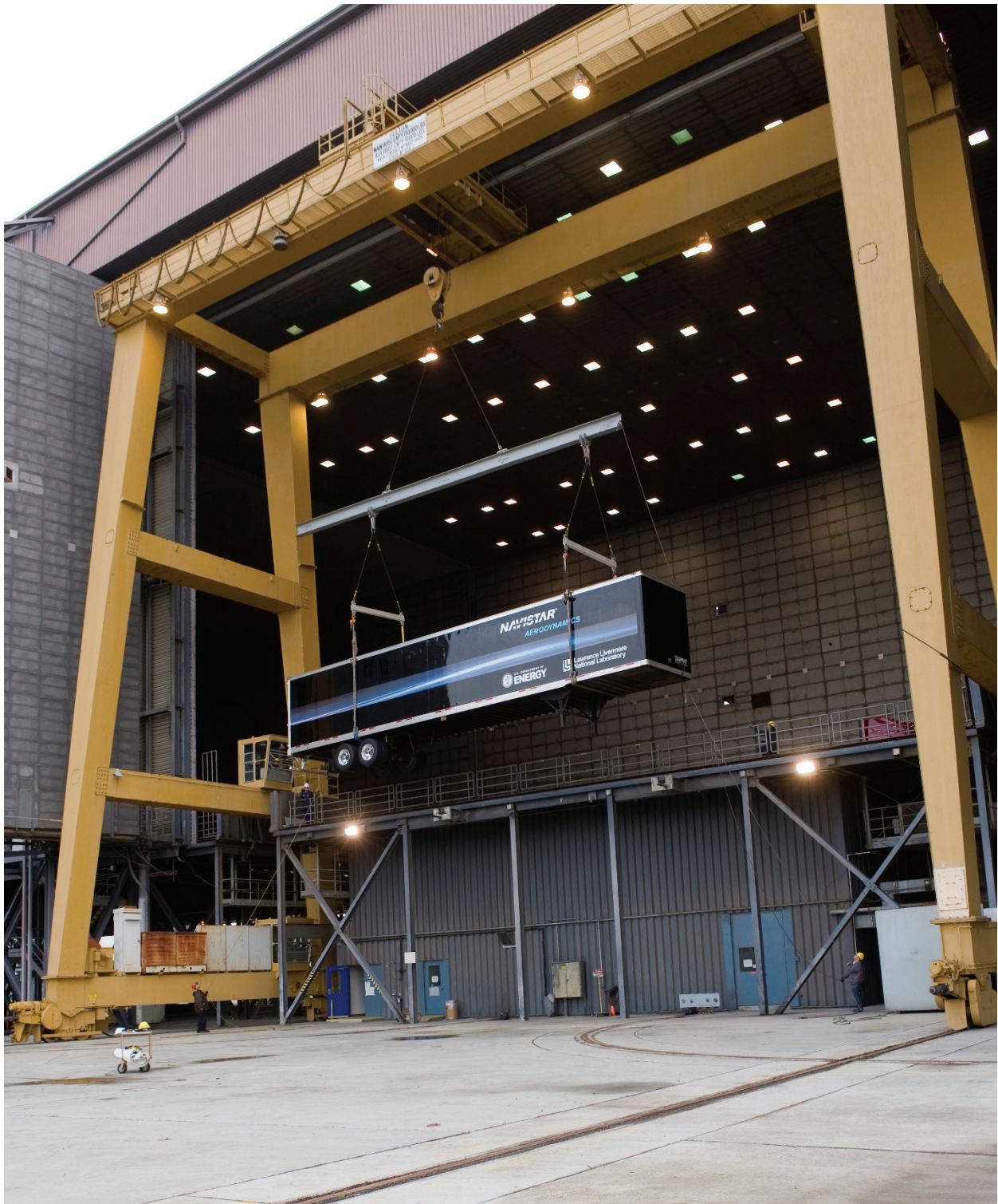
Figure 282. Truck-trailer installation in the 80- by 120-foot test section. ( NASA ACD10-0020-023 )
