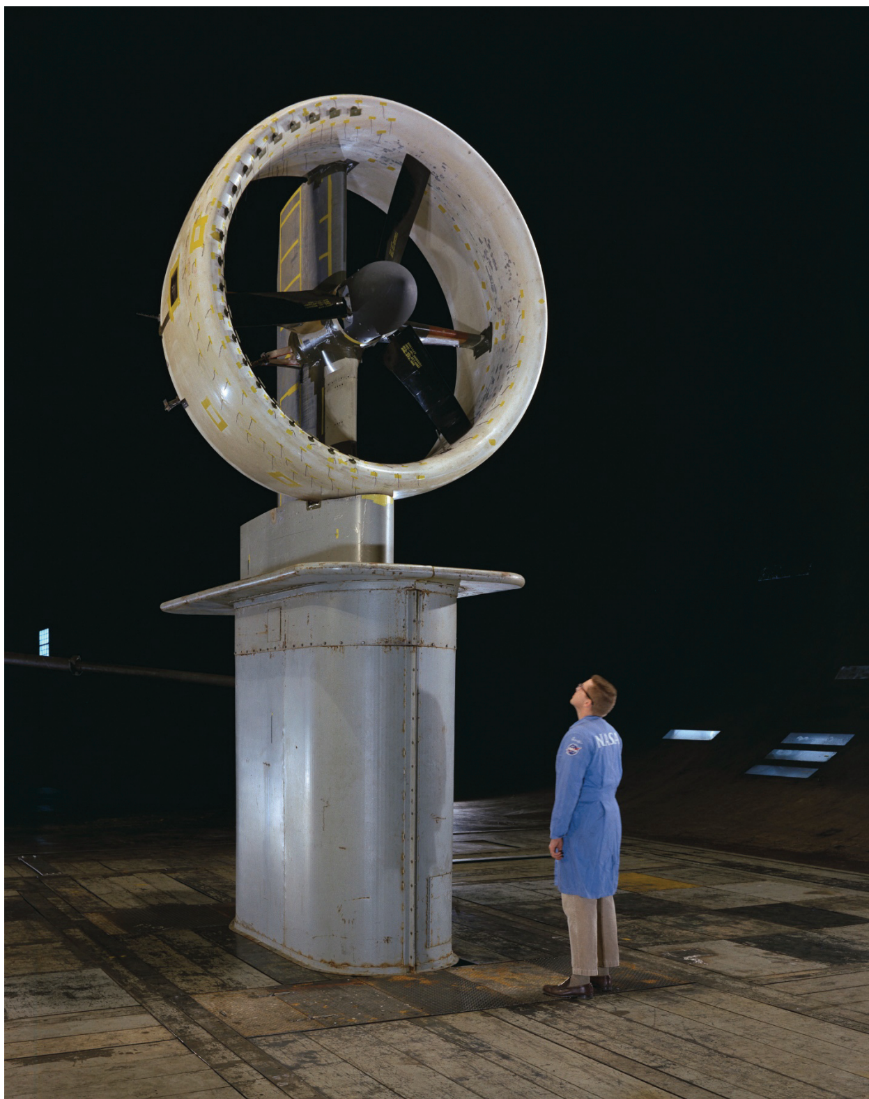
Figure 183. Bell X-22A 7-foot-diameter ducted fan with vortex generators on upstream duct lip (left side) with Mike Falarski in photo. (NASA A-38036)
