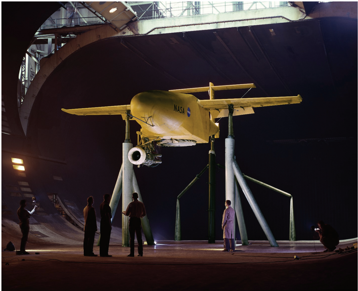
Figure 152. Lift fan mounted in the fuselage of 1/2-scale model. (NASA AC-27149-B)
