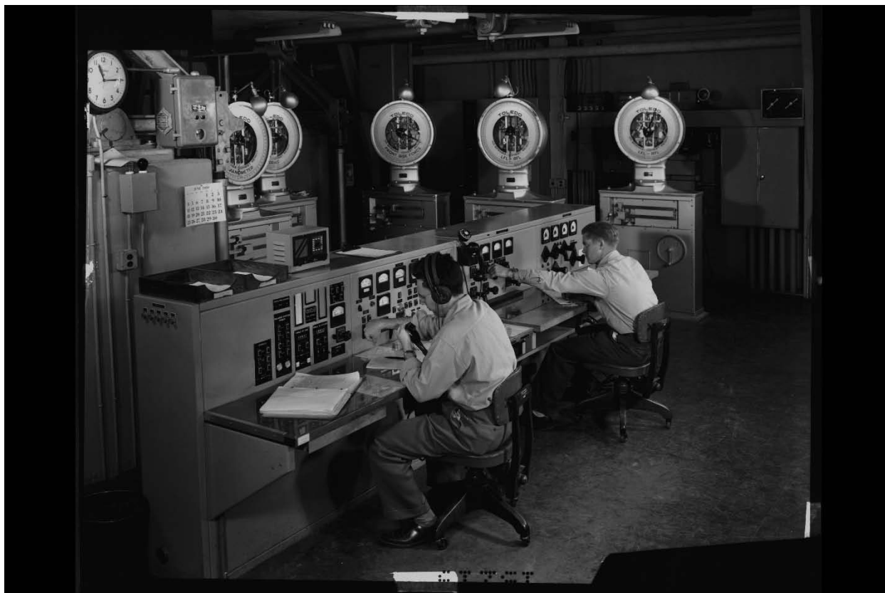
Figure 22. Control room bench board. Five of the scale heads are shown. (NACA A-15219)
