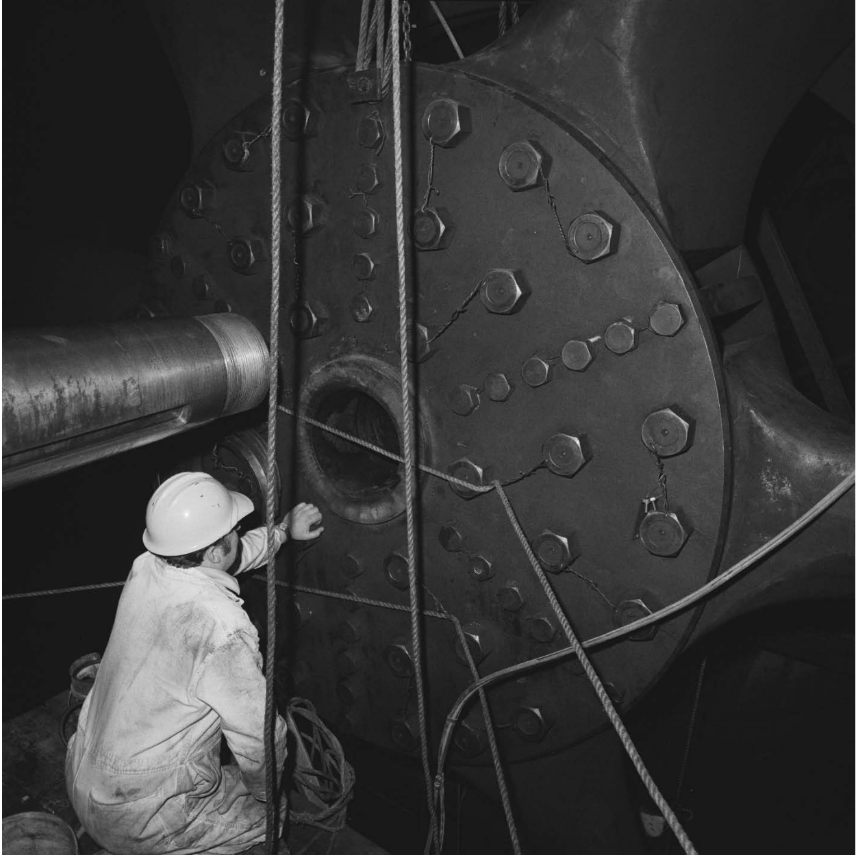
Figure 25. Fan has been removed. Fan hub plate is shown with all of the bolt heads, and tapered drive shaft with keyway end is shown on the left. (NASA A71-8832)
