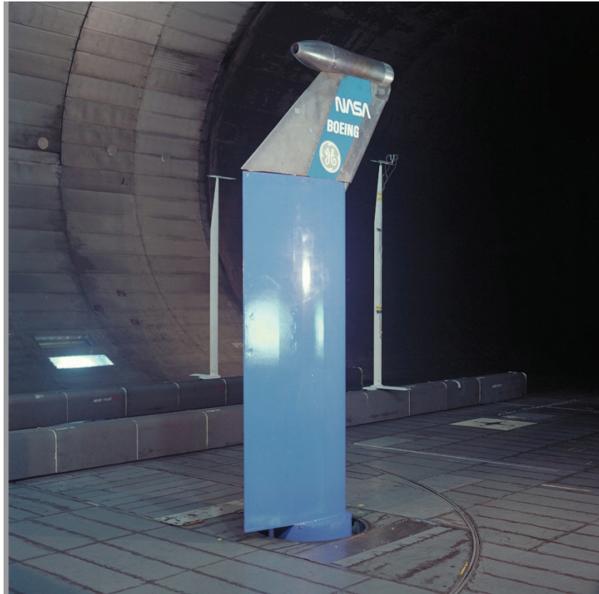
Figure 273. Heated supersonic jet acoustic experiments. (AC94-0029-3)
