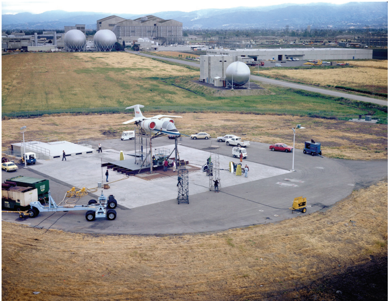
Figure 184. Grumman 698 tilt-nacelle V/STOL model during outside static testing. (NASA AC80-0455-6)
