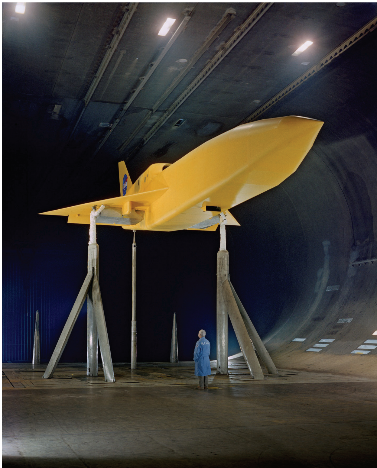
Figure 161. Three-quarter front view of lift fans in a 5-percent-thick wing of a supersonic fighter model. (NASA A-37808)
