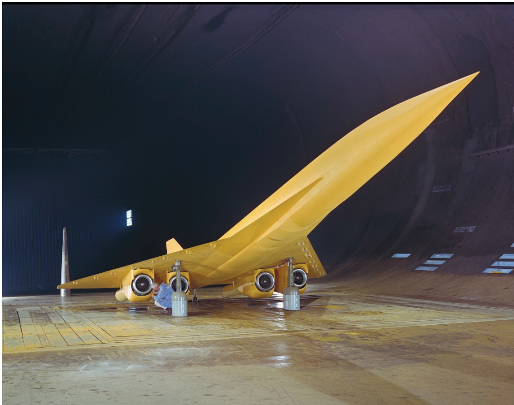
Figure 127. Ground-effect testing of a double-delta SST model. (NASA A-37700)
