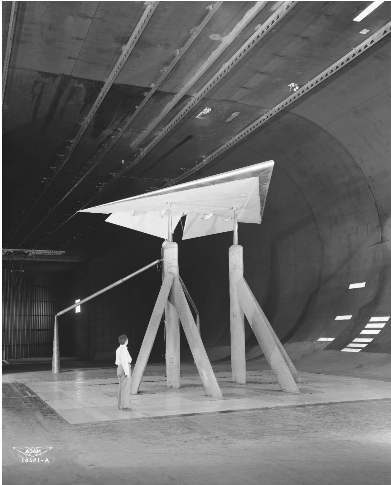
Figure 87. Triangular-wing- (delta-wing-) alone model with an aspect ratio of 2 and a wingspan of 25 feet; flaps are down. (NACA A-15261-010)
