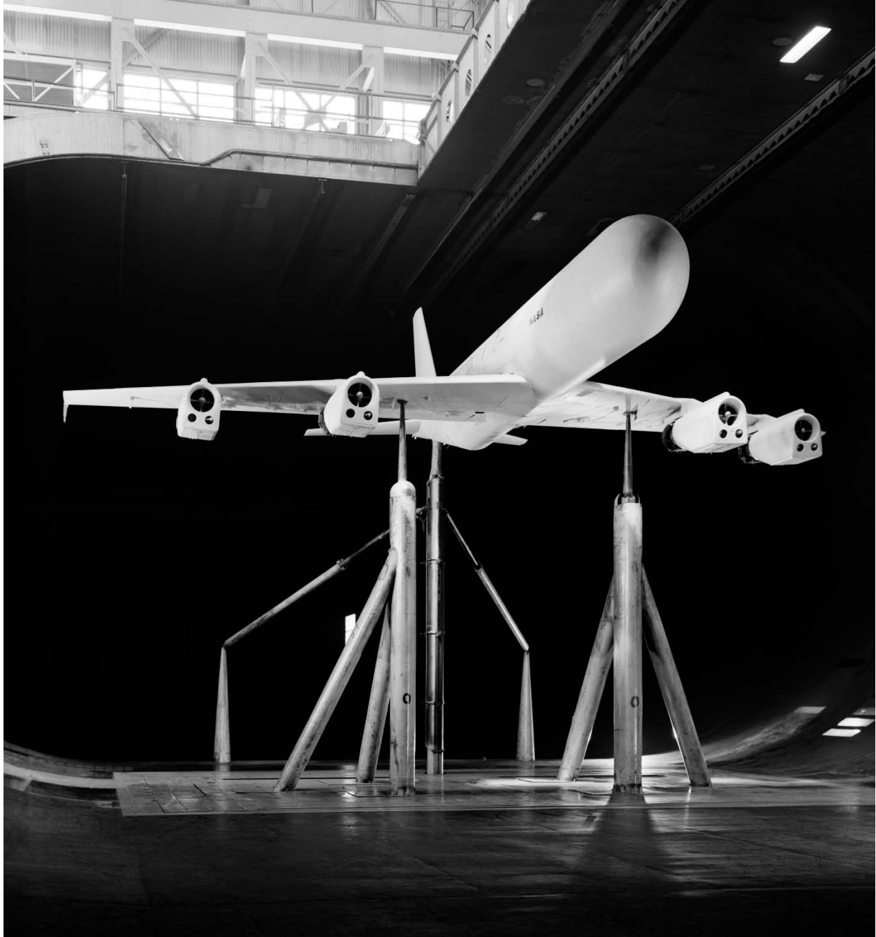
Figure 121. Four-engine jet-transport model used for thrust-reverser experiments. ( NASA A-25585 )
