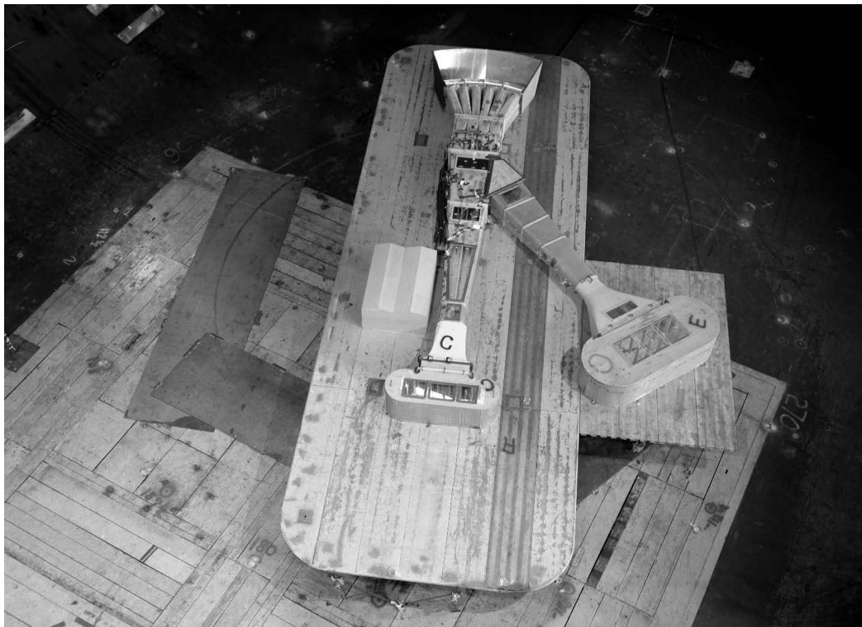
Figure 28. Super Tunnel model mounted on a ground board used for wind-effect studies in the tunnel. Y-configuration, high-speed test-section screened inlet in lower center, low-speed test-section screened inlet to the right, and vertical exhaust at top of figure. (NASA A72-2687)
