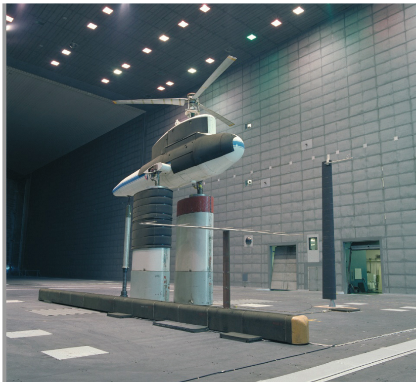
Figure 240. Isolated proprotor experiments for the XV-15 tilt-rotor aircraft in hover orientation in the 80- by 120-foot test section. (NASA AC98-0261-6)
