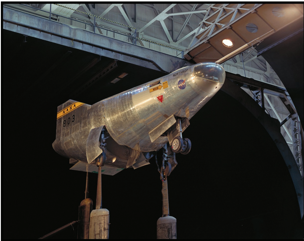
Figure 223. Three-quarter front view of M2-F2 lifting-body experimental aircraft with landing gear down. (NASA A-35069)
