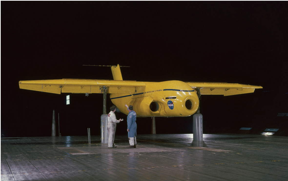
Figure 203. Three-quarter front view of de Havilland augmentor wing model during ground-effect experiments. (NASA AC-36486)
