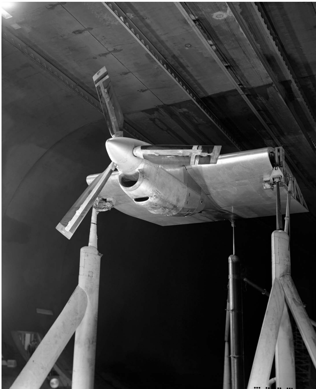
Figure 102. Nacelle with propeller decoupler and controlled-feathering device mounted on partial wing. (NACA A-18957)
