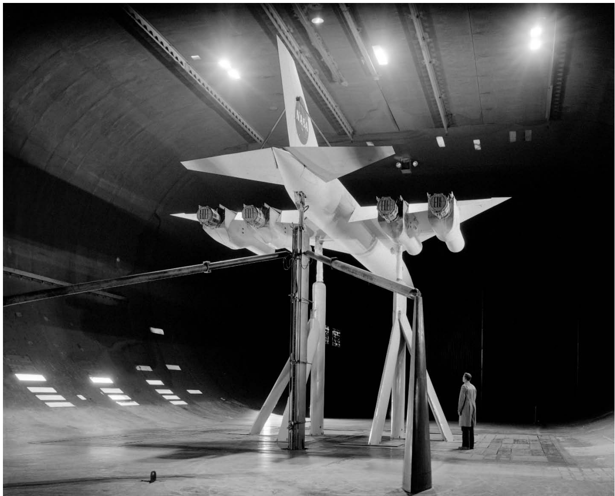
Figure 122. Delta-wing SST model used for thrust-reverser experiments; Tom Wills in photo. (NASA A-31004)
