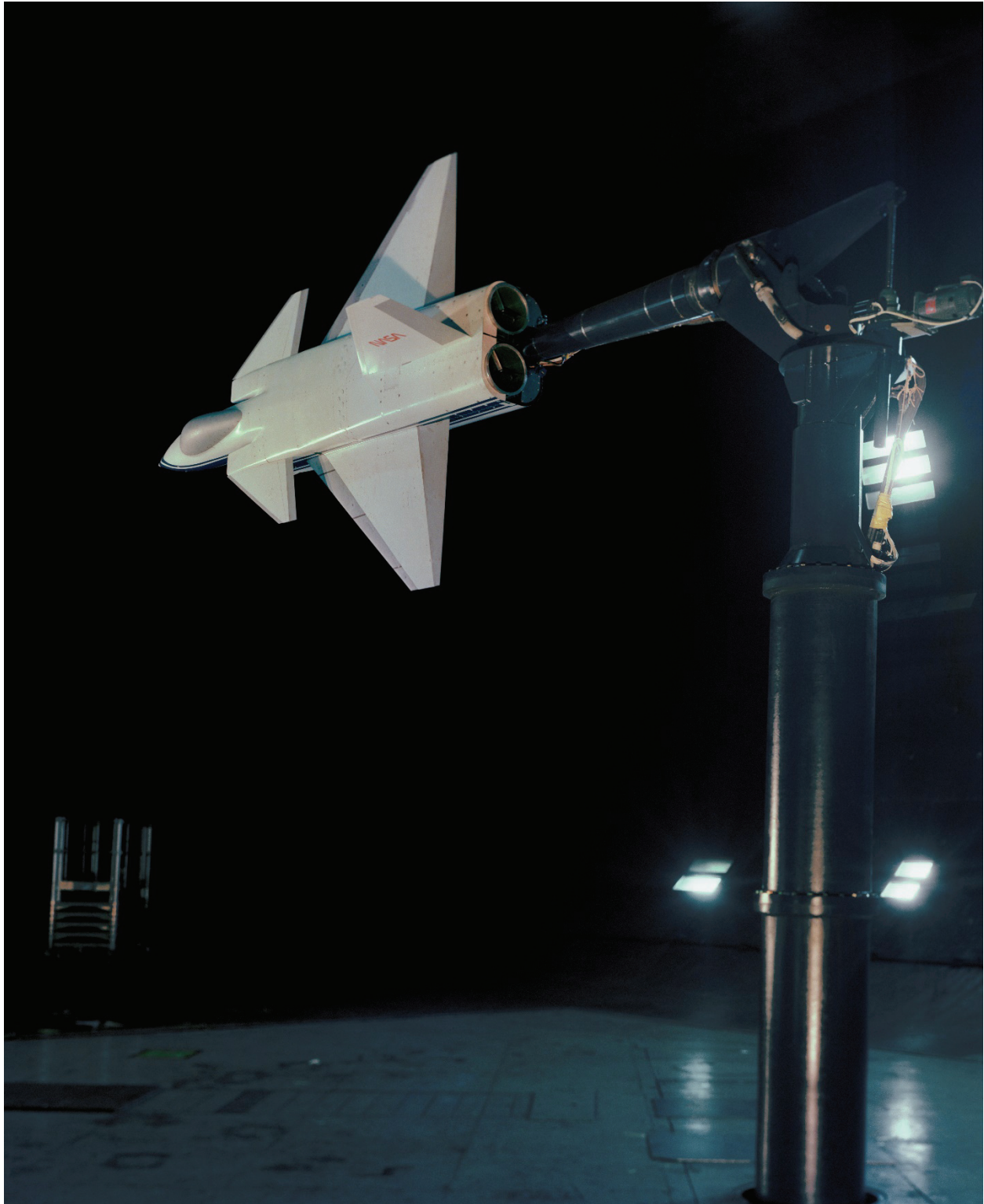
Figure 176. VATOL fighter model mounted sideways on a sting so it could be rotated in horizontal plane to increase the angle of attack to high values. ( NASA AC80-0623-1 )
