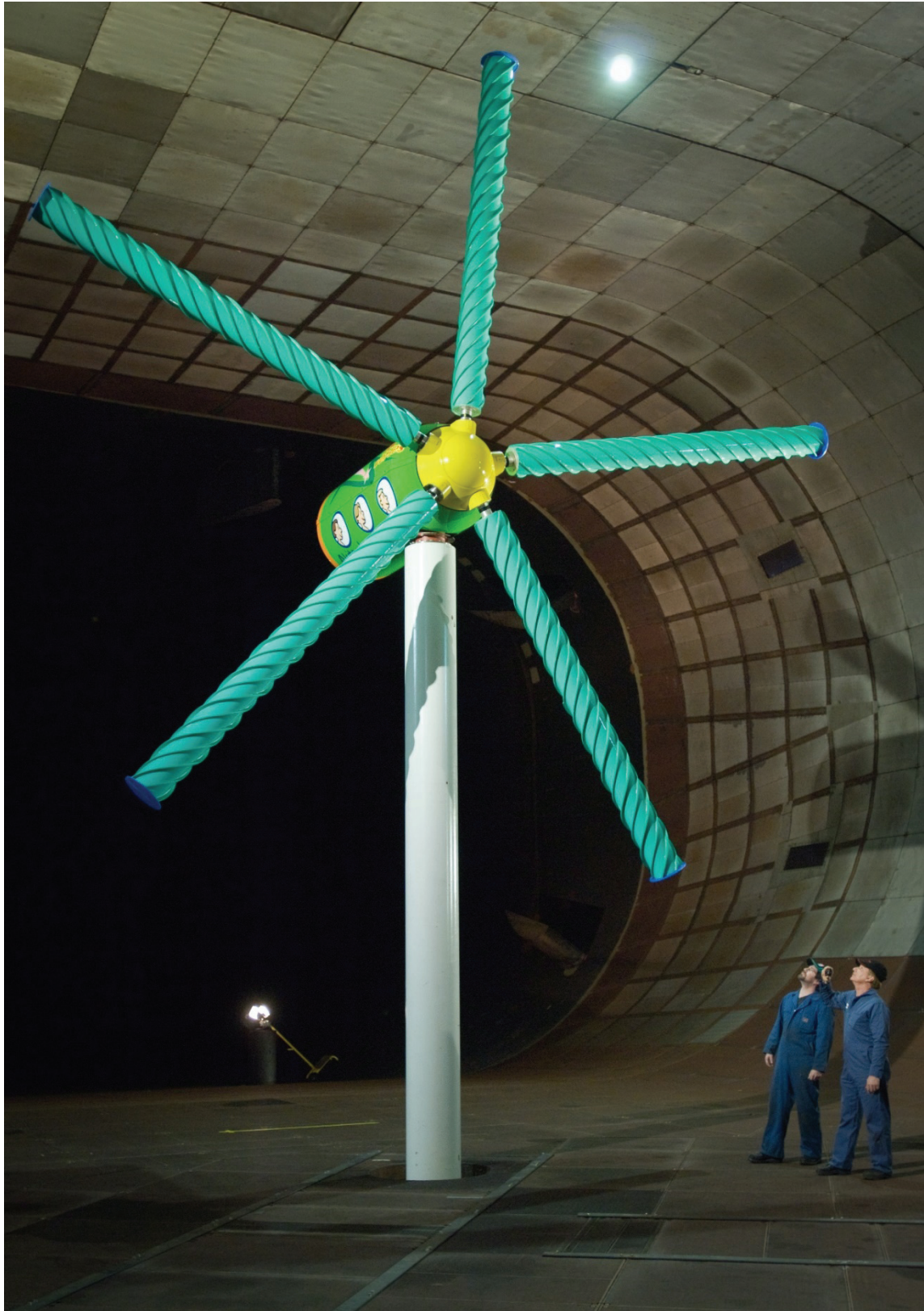
Figure 280. Mecaro Spiral Magnus wind turbine in the 40- by 80-foot test section; note the spirally wrapped fins around the five circular “blades.” (NASA ACD07-0242-002)
