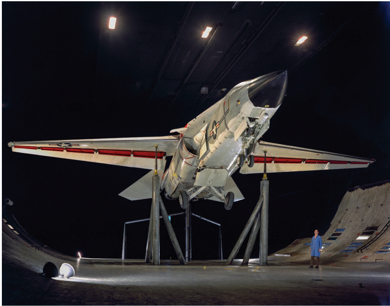
Figure 109. Three-quarter front view of the General Dynamics F-111B fighter/bomber with wings unswept and landing gear down—another very large aircraft in the tunnel. (NASA A-42117-040)
