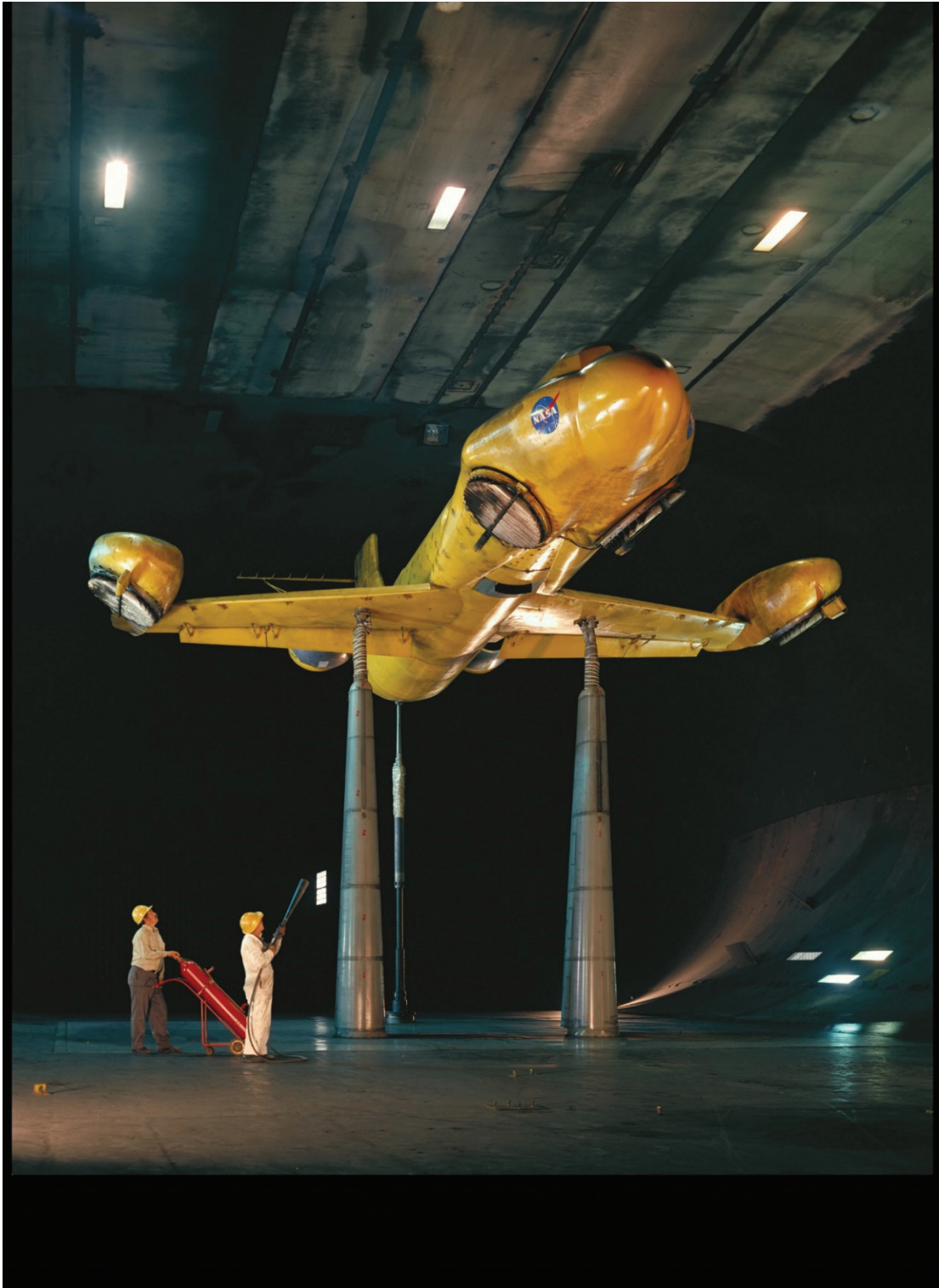
Figure 160. STOL transport model with lift fans and cruise fans. (NASA AC75-1002)
