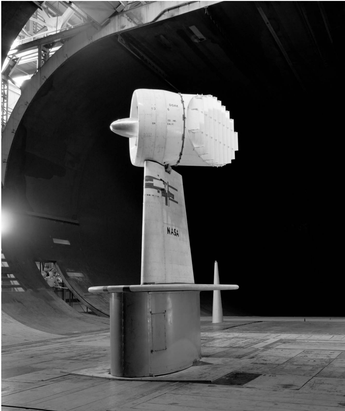
Figure 179. Four-foot-diameter ducted-fan semispan model with variable-exit-vane cascade. (NASA A-28982)
