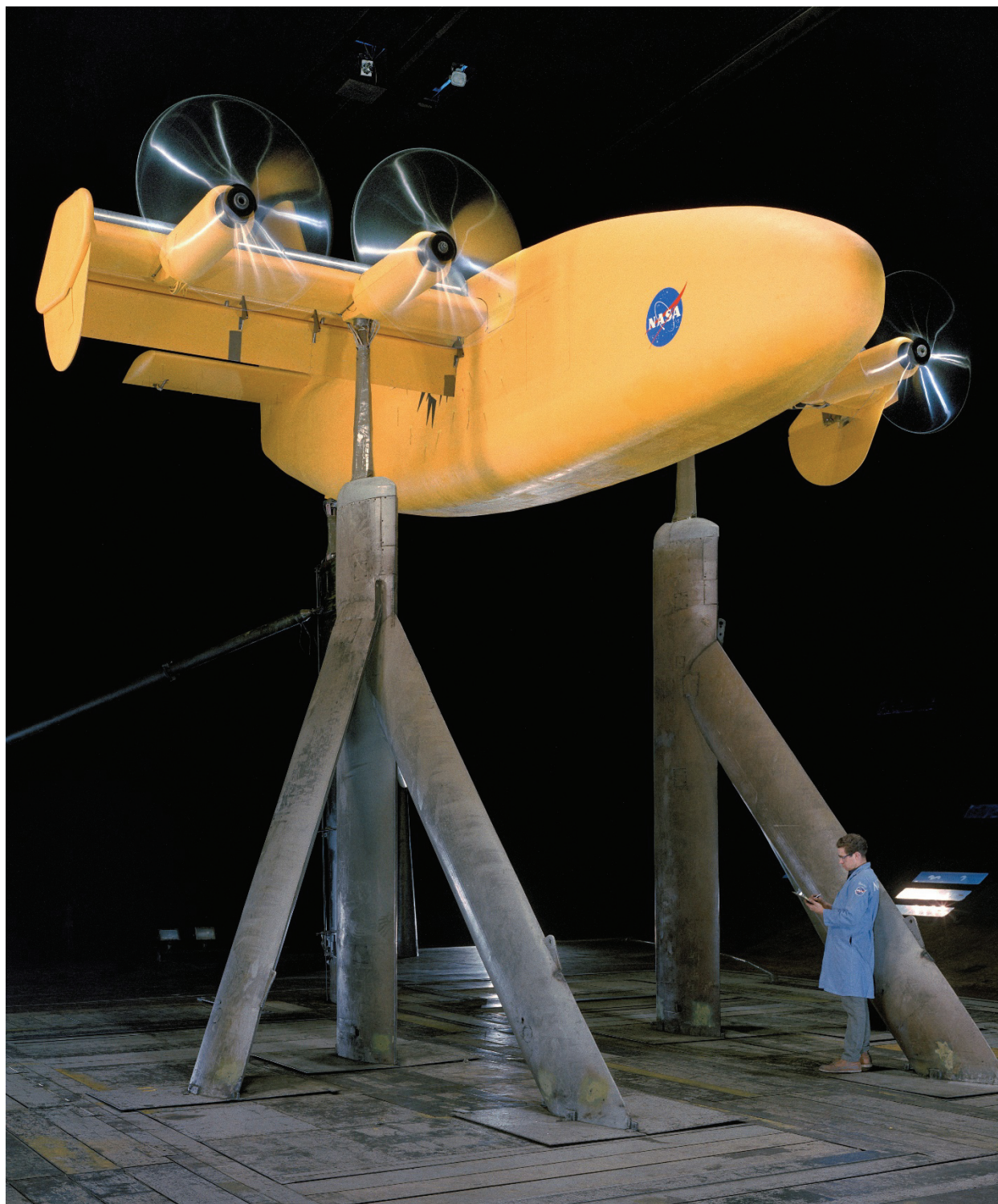
Figure 201. Three-quarter front view of four-propeller model with rotating-cylinder flaps. (NASA A-39267)
