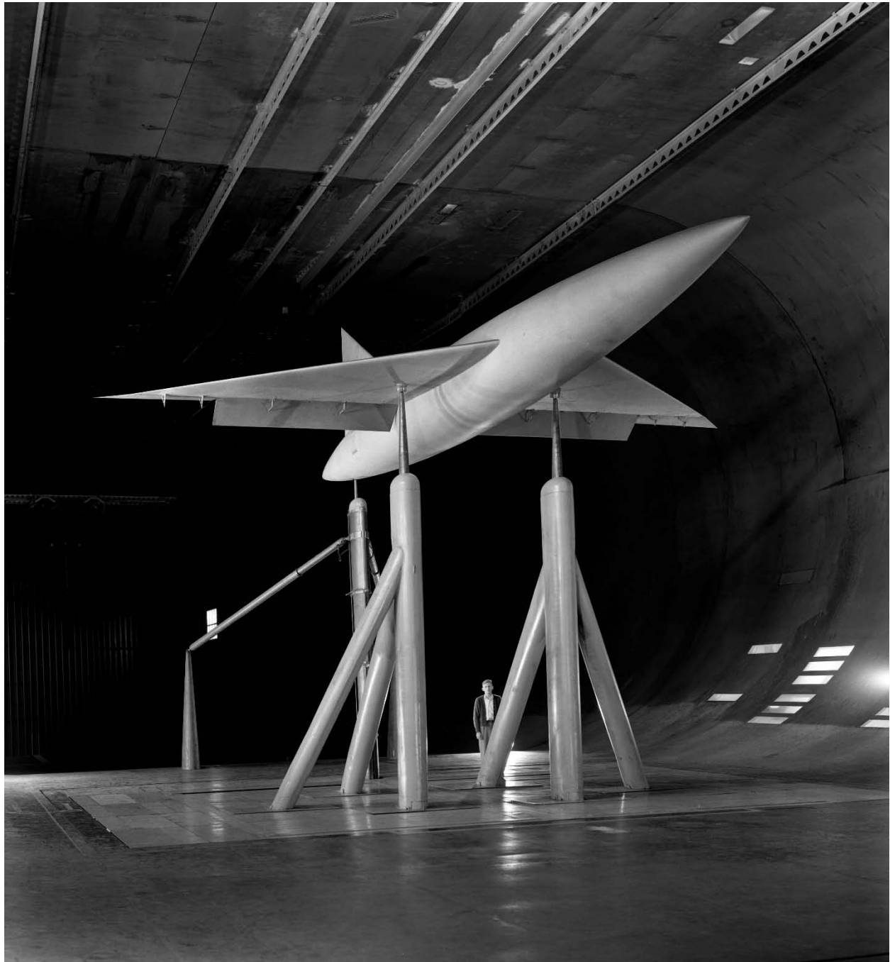
Figure 90. Three-quarter front view of triangular-wing model with an aspect-ratio-4 wing with flaps down. (NACA A-16603)
