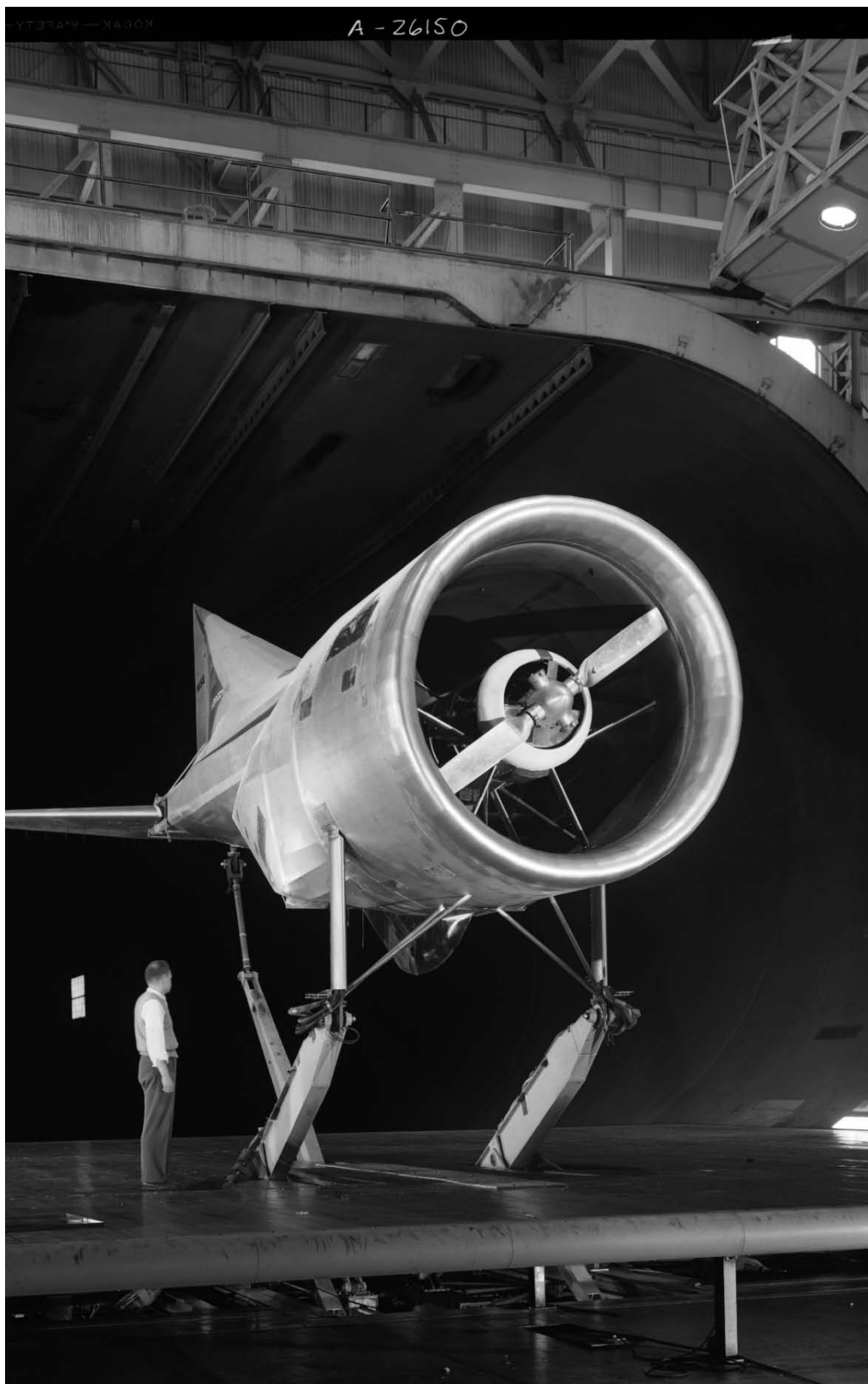
Figure 177. Collins Lippisch Aerodyne VTOL model on variable-height struts with Dave Koenig in photo. Front propeller in duct can be readily seen. (NASA A-26150)
