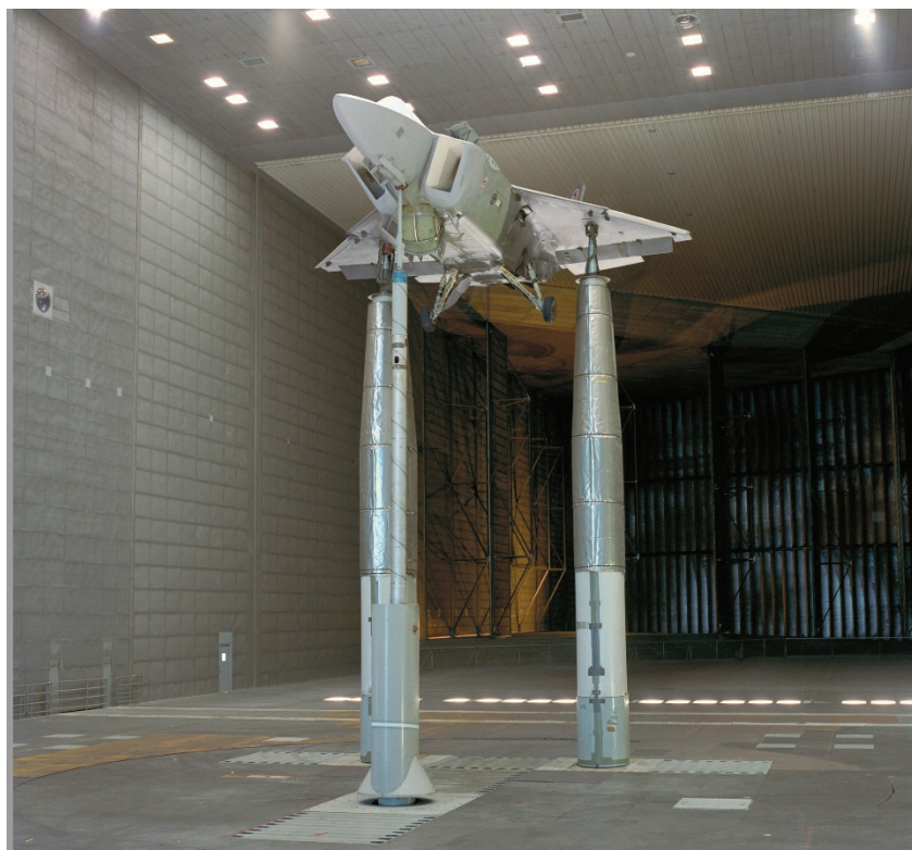
Figure 257. An 86-percent-scale model of the JSF in the 80- by 120-foot test section. ( NASA AC96-0233-1 )
