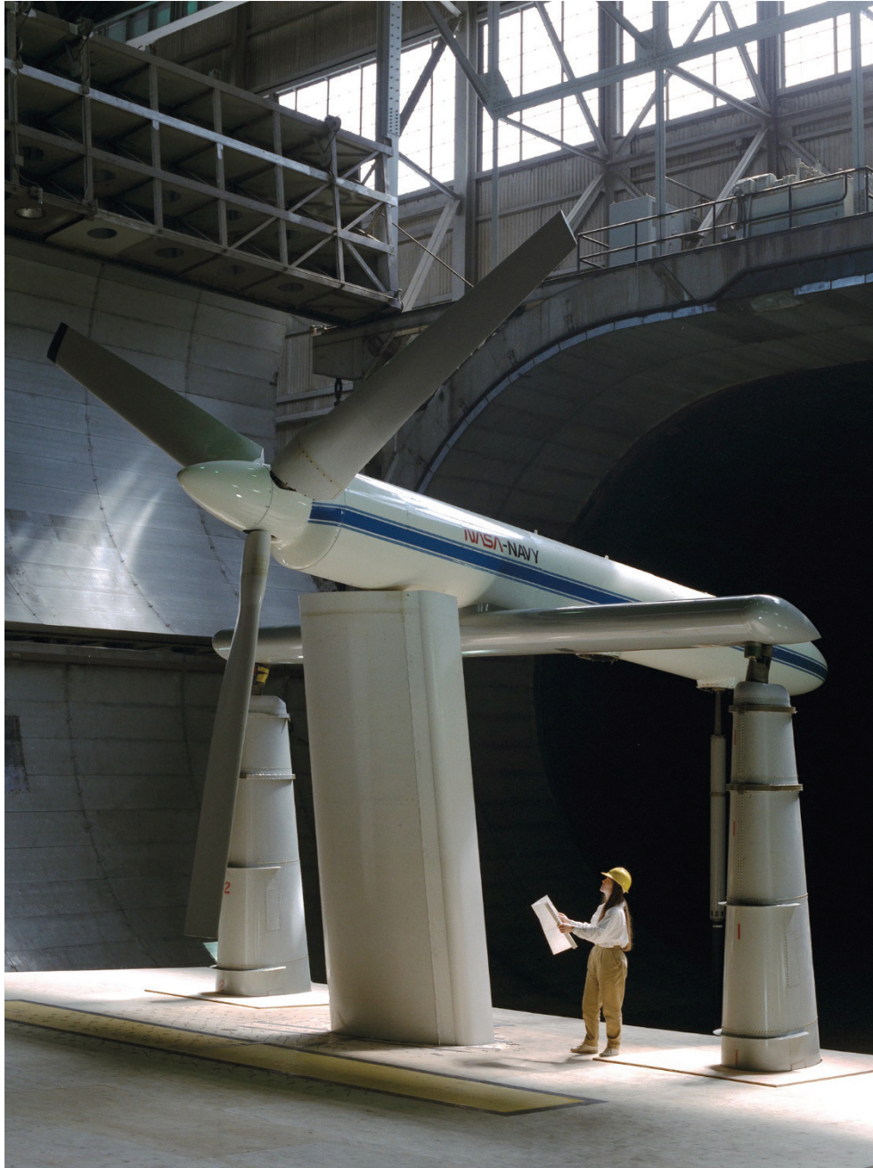
Figure 241. A 2/3-scale V-22 tilt-rotor aircraft proprotor in cruise orientation in the 40- by 80-foot test section. (NASA AC88-0182-2)
