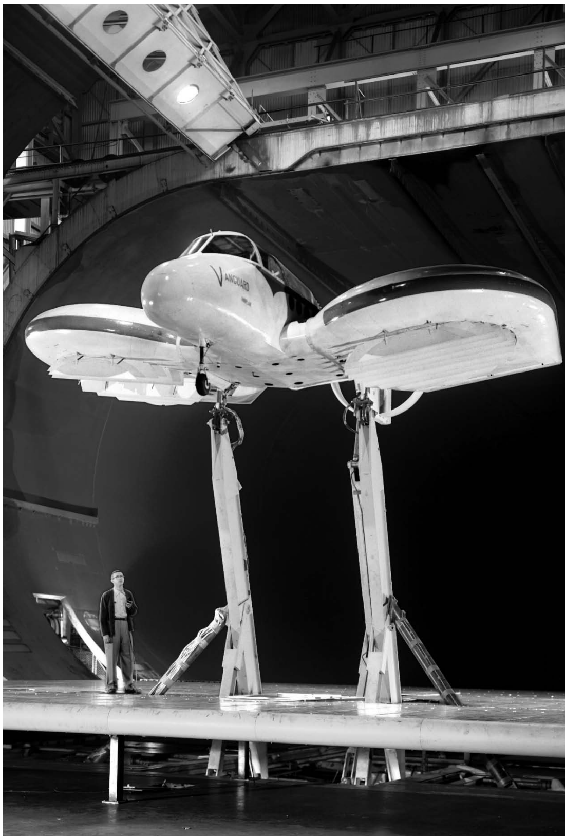
Figure 166. Three-quarter front view of the Vanguard Omniplane low-pressure-ratio fan-in-wing experimental aircraft with engineer Ralph Maki in photo. (NASA A-26189)
