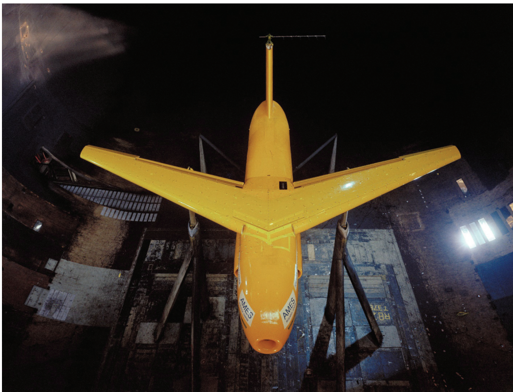
Figure 205. Overhead front view of de Havilland augmentor wing model. (NASA AC71-2502)
