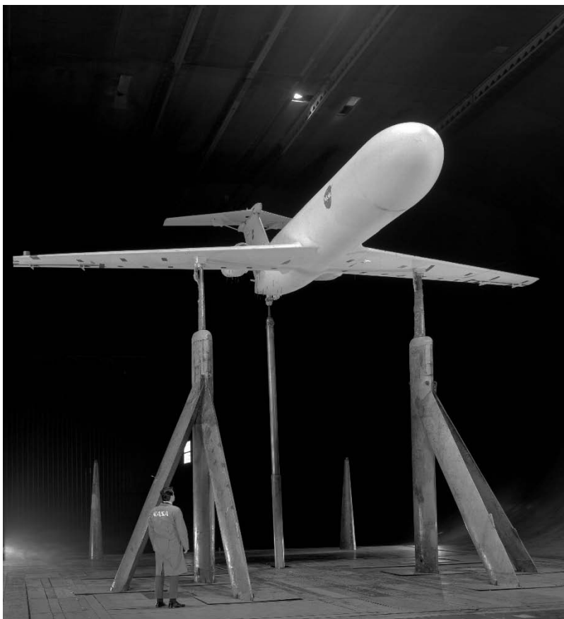
Figure 114. Subsonic jet transport model with aft fuselage-mounted engines and a T-tail, used for deep-stall studies. (NASA A-36210)
