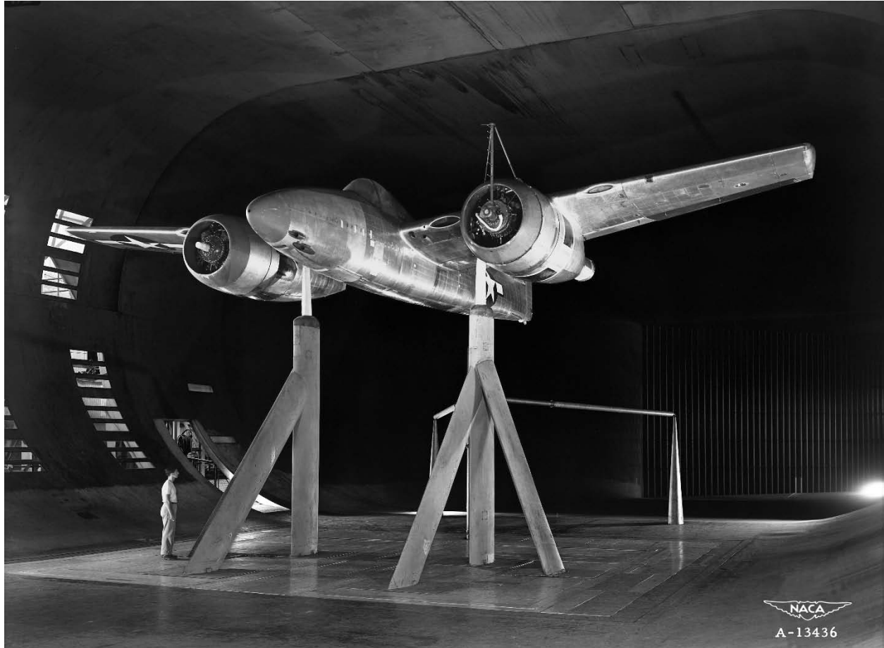
Figure 99. Flow surveys at the left propeller plane of the Grumman XF7F-1. Vertical flow-measuring rake on top of left nacelle. ( NACA A-13436 )
