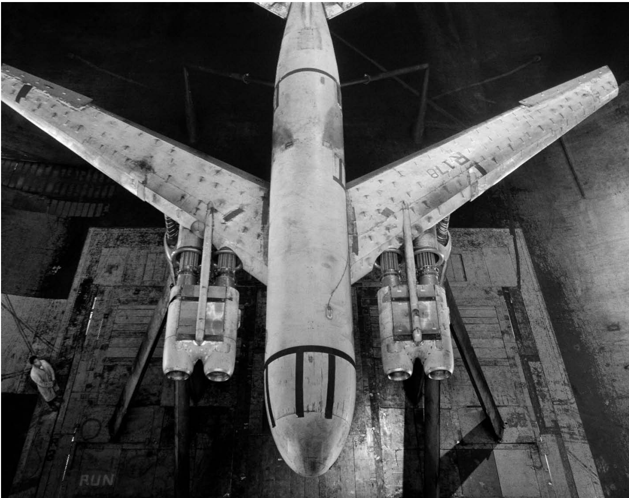
Figure 215. Overhead front view of EBF model using augmented jet engines. Bell-mouth inlets of augmentors are shown close to the leading edges of the wings. Exhaust flow is directed to flap trailing edges to increase lift. (NASA A-42494-001)
