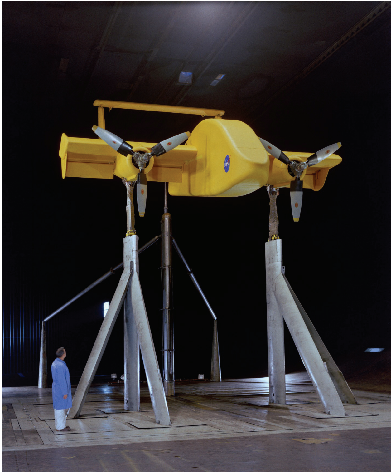
Figure 199. Three-quarter front view of two-propeller model with rotating-cylinder flap. (NASA A-41389)
