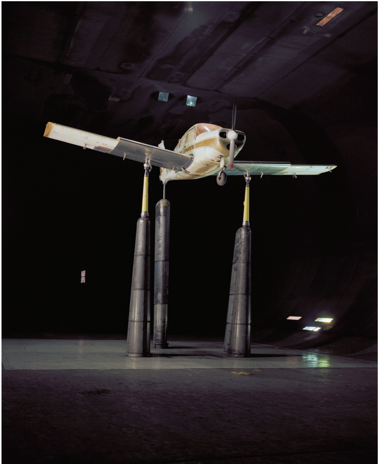
Figure 131. Stall studies using a Beechcraft Musketeer, Model 23A. Note the wing-leading-edge glove on the inboard half of the wings. (NASA AC79-0973-2)
