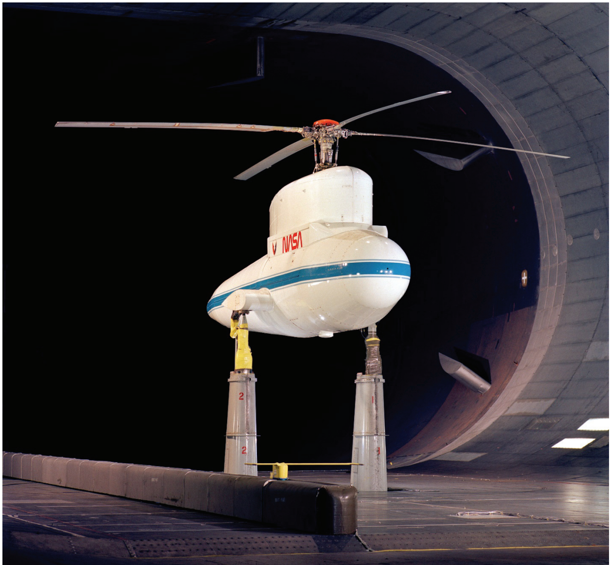
Figure 245. MBB Bo-105 hingeless main rotor mounted on the RTA. ( NASA AC93-0035-13 )
