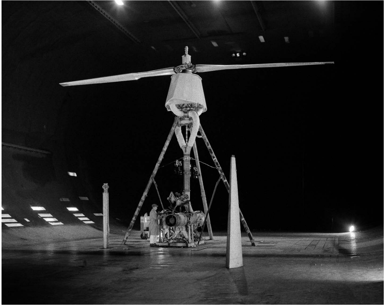
Figure 136. Giravions Dorand jet-flap helicopter rotor with Sam Yacco, aircraft mechanic, in photo. The jet engine on the floor of the test section produces compressed air for the jet flap. (NASA A-34960)
