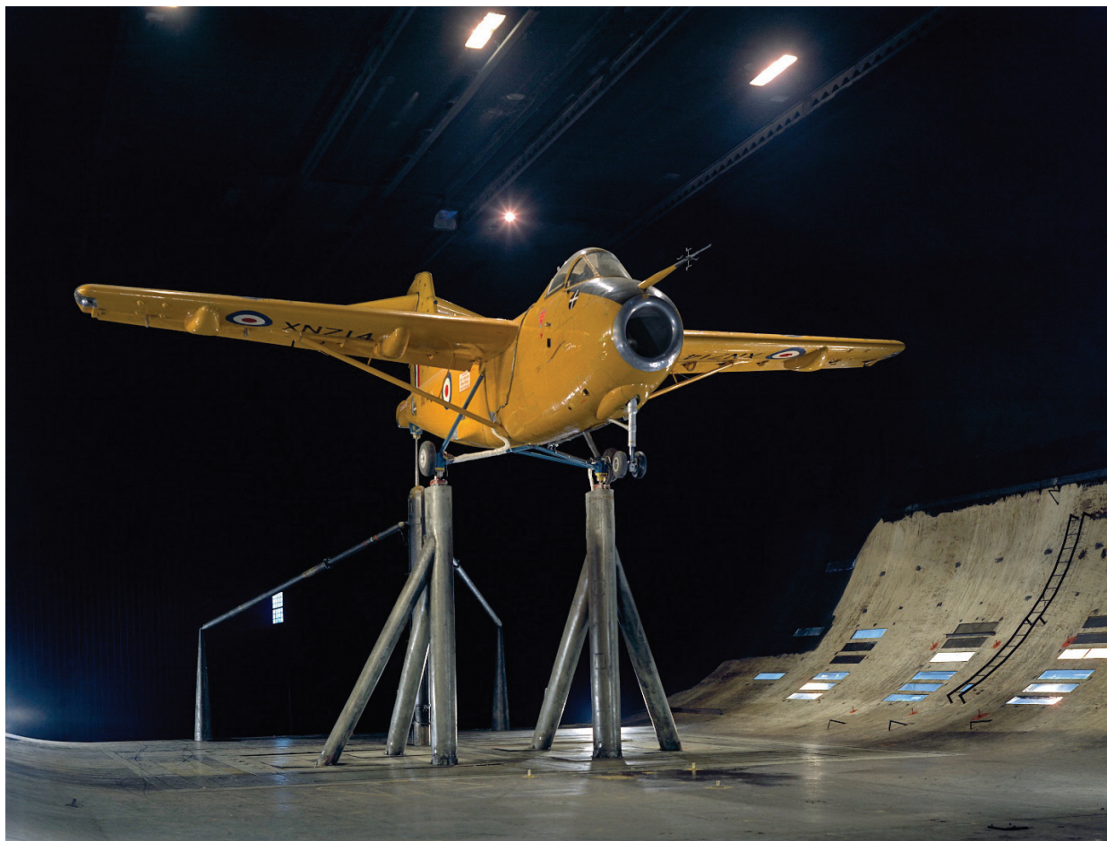
Figure 212. Three-quarter front view of the Hunting H.126 jet-flap experimental aircraft. (NASA AC-42409)
