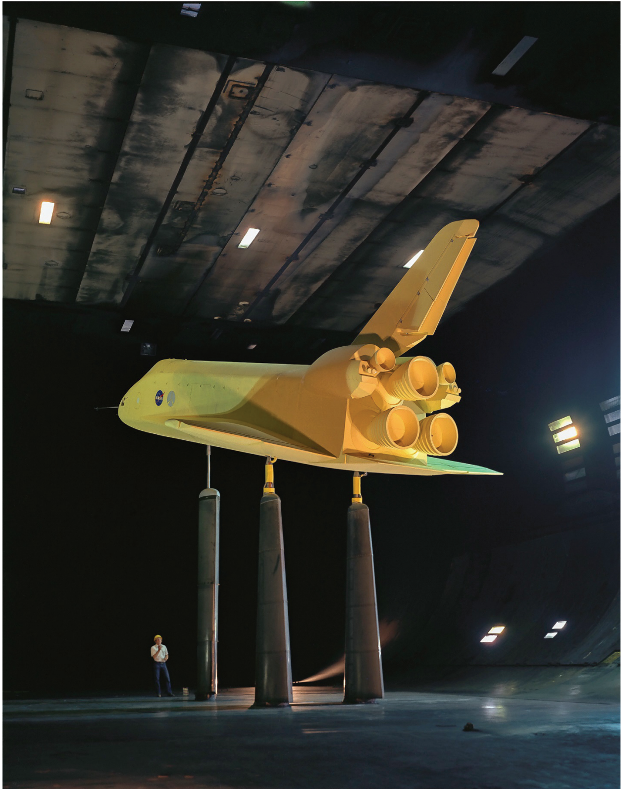
Figure 232. Three-quarter rear view of the space shuttle model in the wind tunnel showing mock-ups of engine nozzles. (NASA AC75-1161-003)
