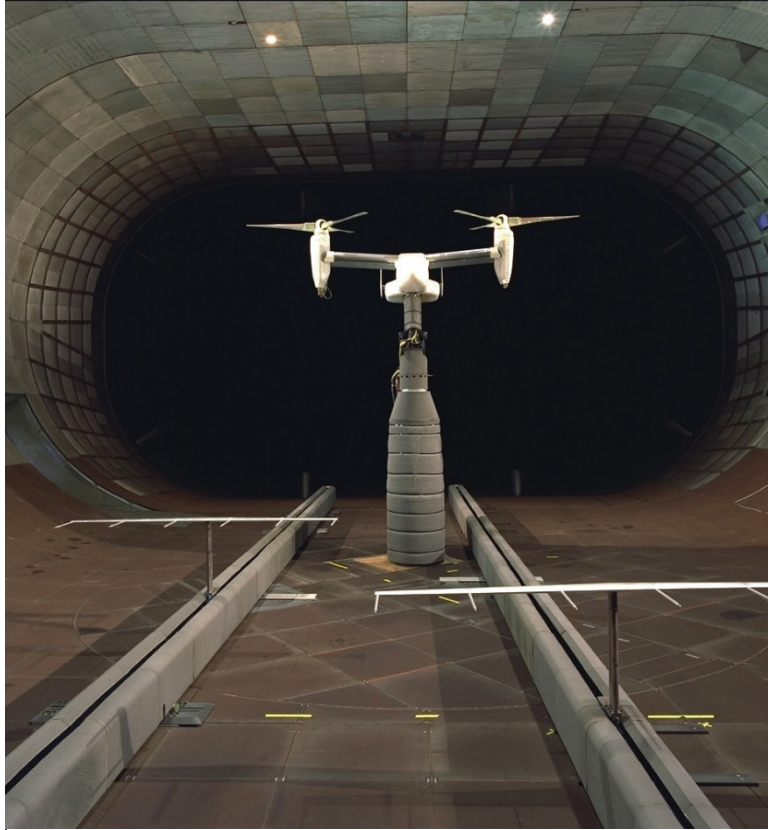
Figure 242. TRAM test stand; approximately 1/4-scale model V-22 in the 40- by 80-foot test section. ( J. Sacco collection, T40-0062 )
