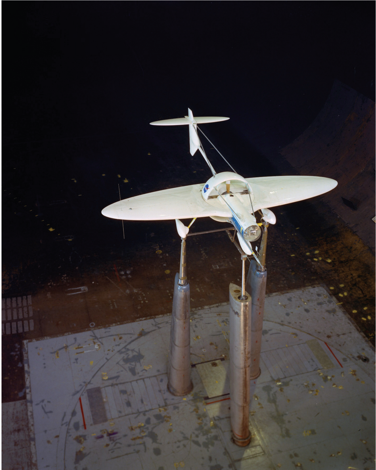
Figure 239. Oblique-wing remotely piloted research model with the wing in the straight orientation. (NASA AC75-2410)
