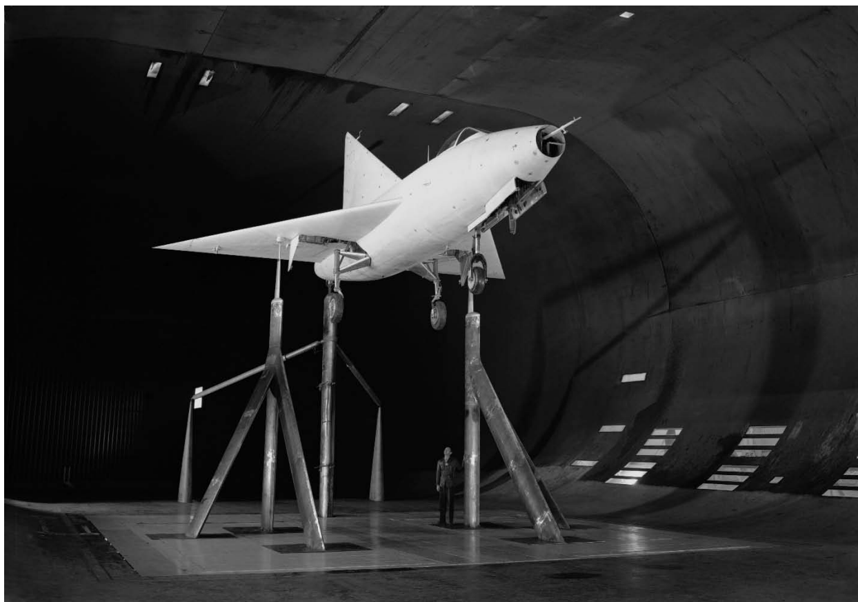
Figure 86. Flying mock-up of the Consolidated Vultee XP-92 delta-wing aircraft in the tunnel with landing gear down. The flying mock-up was going to have a turbo-jet engine, but the airplane was intended to have both ram-jet and rocket power plants. (NACA A-12352)
