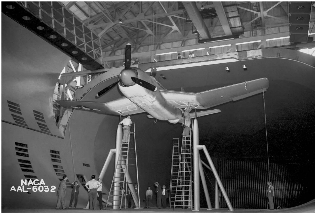
Figure 60. Douglas XSB2D-1 being mounted on the support struts. Initially, tall ladders (as shown) were used by the mechanics to access the strut tips for attachment of the aircraft. Ball joints at the strut tips served as pivots when the angle of attack was varied using the telescoping tail strut. (NACA AAL-6032)
