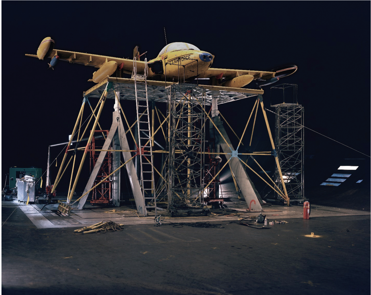
Figure 123. Cessna A-37B airplane with experimental thrust reversers with a temporary ground board being installed. (NASA AC-41258)
