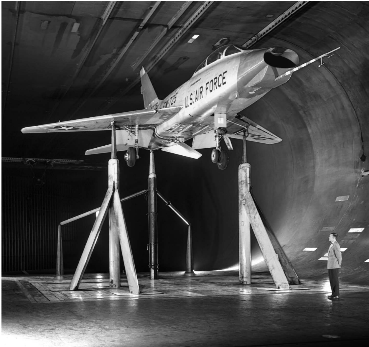
Figure 120. North American F-100F fighter used for thrust-reverser tests; landing gear down and Mark Kelly in photo. (NASA A-24788)
