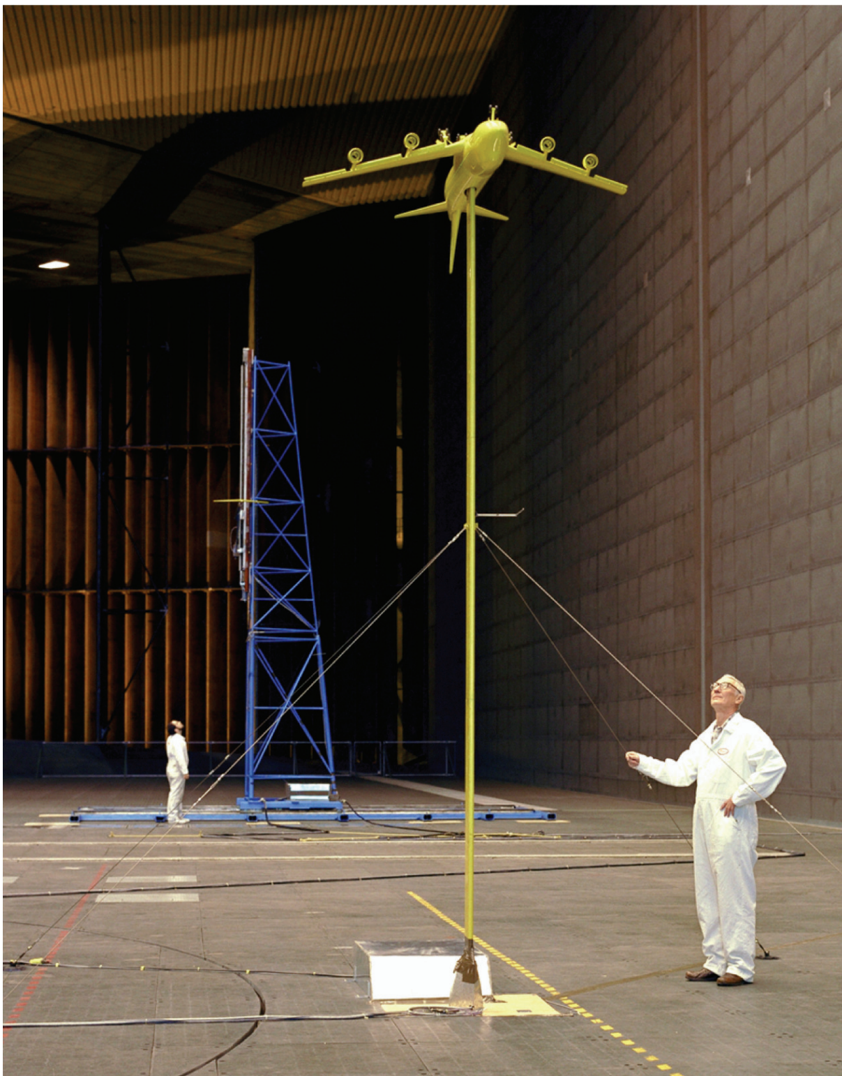
Figure 263. Lift-generated tip-vortex wakes using a 0.03-scale Boeing 747 model in the 80- by 120-foot test section with Vernon Rossow in photo. Model is upside down to minimize model-support effects on wakes. (NASA AC92-0688-3)
