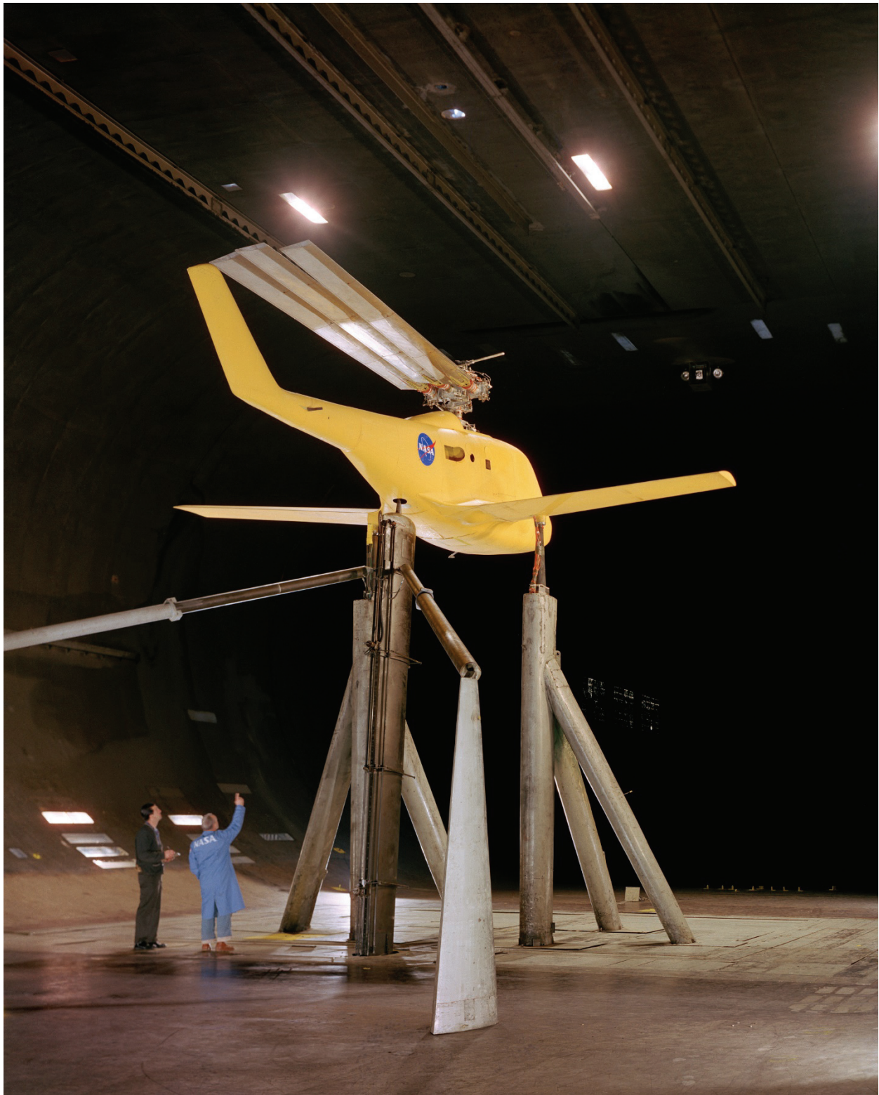
Figure 138. Lockheed stoppable rotor with blades folded back for cruise mode. (NASA A-36030)
