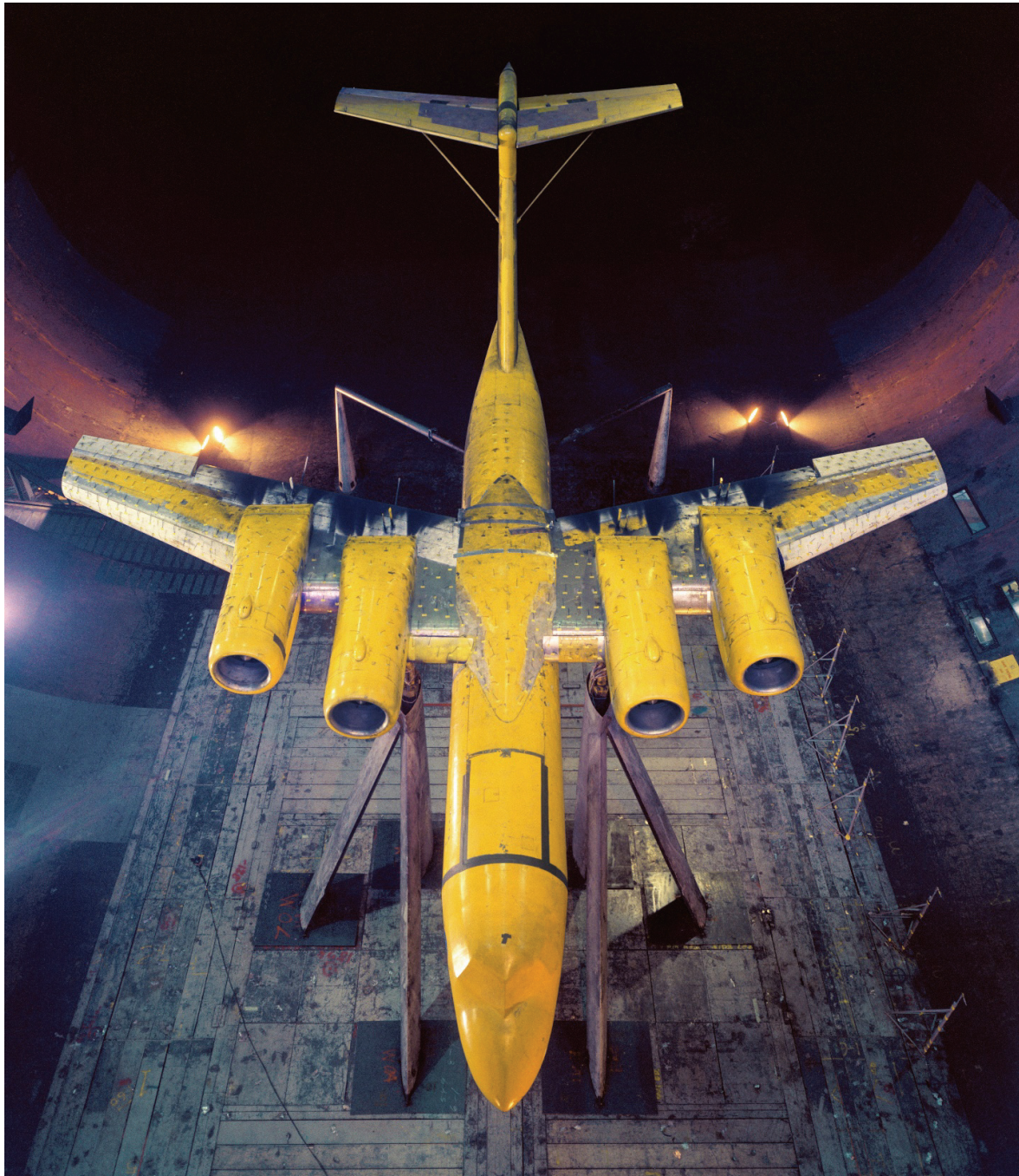
Figure 218. Overhead view of USB model with four jet engines. Jet-engine exhaust is directed over the top of the wing flaps. (NASA AC74-2756)
