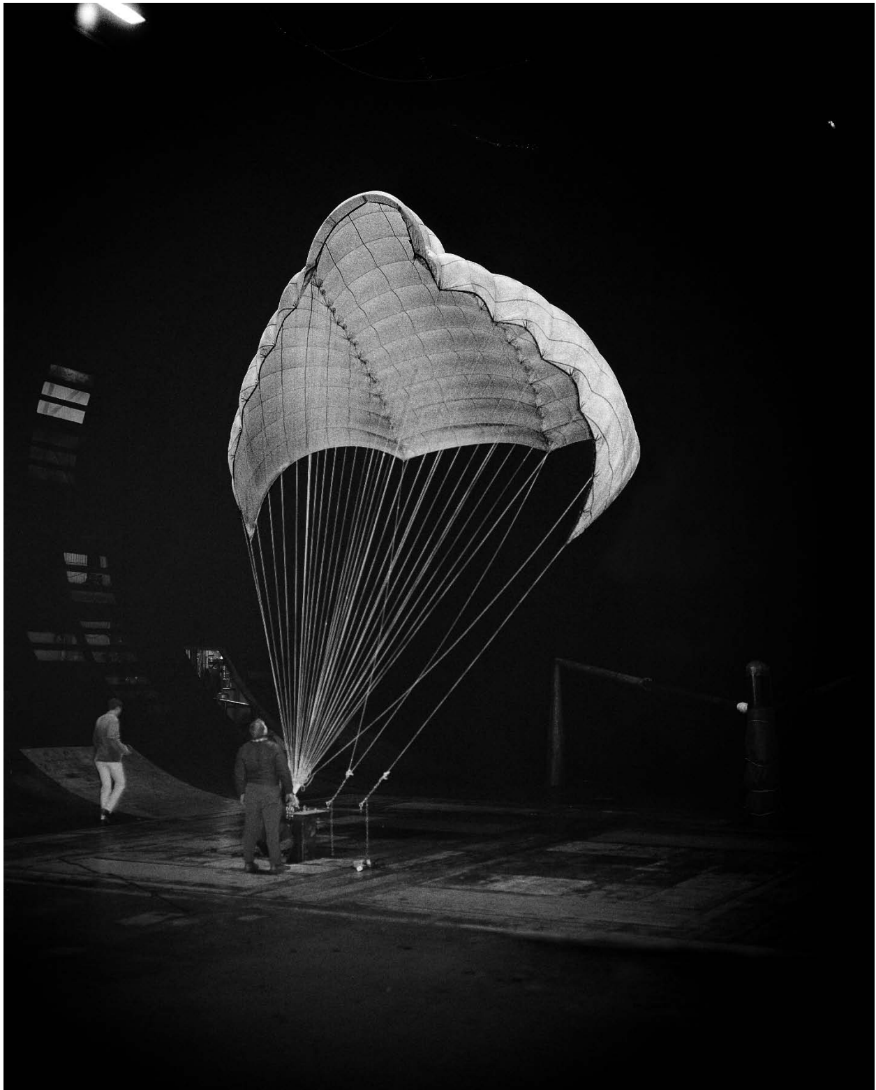
Figure 235. Dual-keel parawing in wind tunnel with vertical orientation. ( NASA A-40414 )
