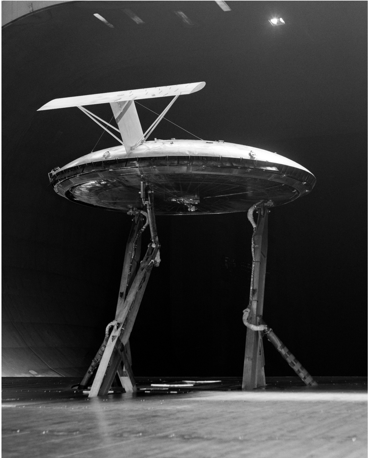
Figure 151. Three-quarter rear view of the Avrocar with a T-tail added for stability. (NASA A-27749)
