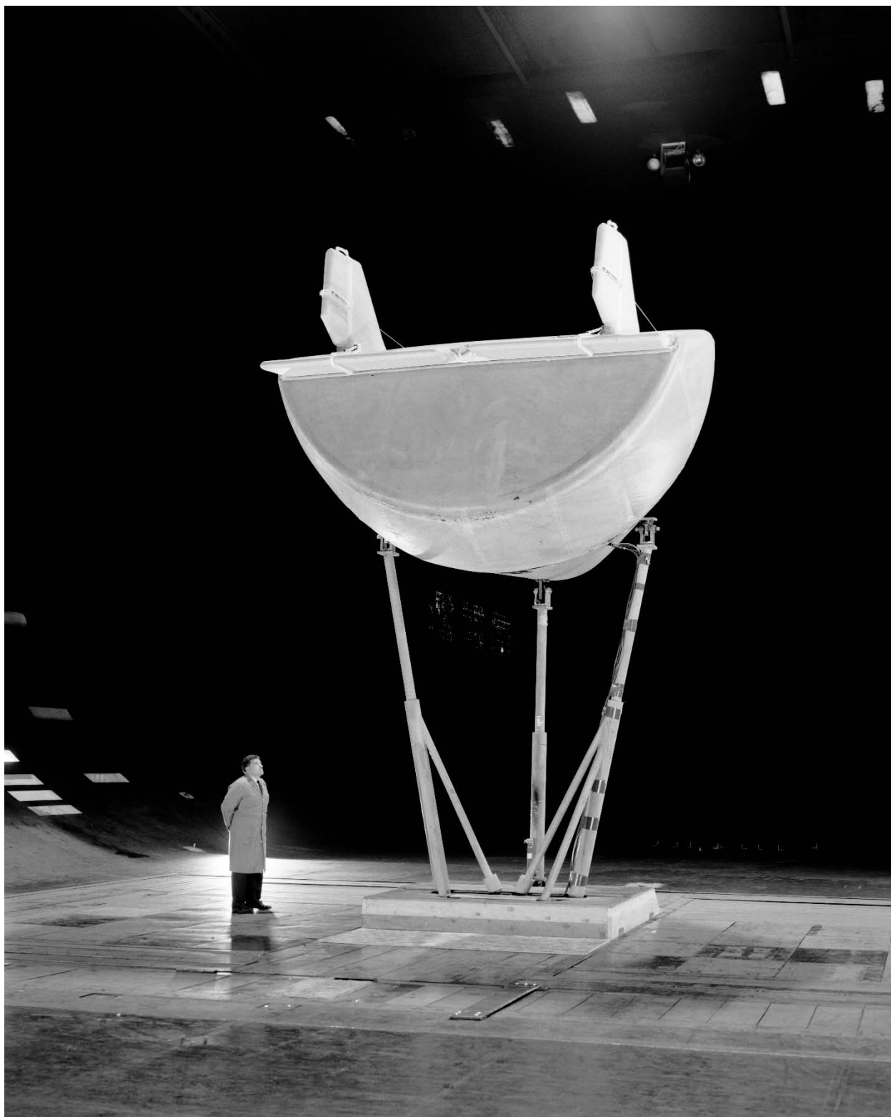
Figure 229. Three-quarter rear view of M1-L lifting-body model with inflatable afterbody and vertical fins. (NASA A-35756)
