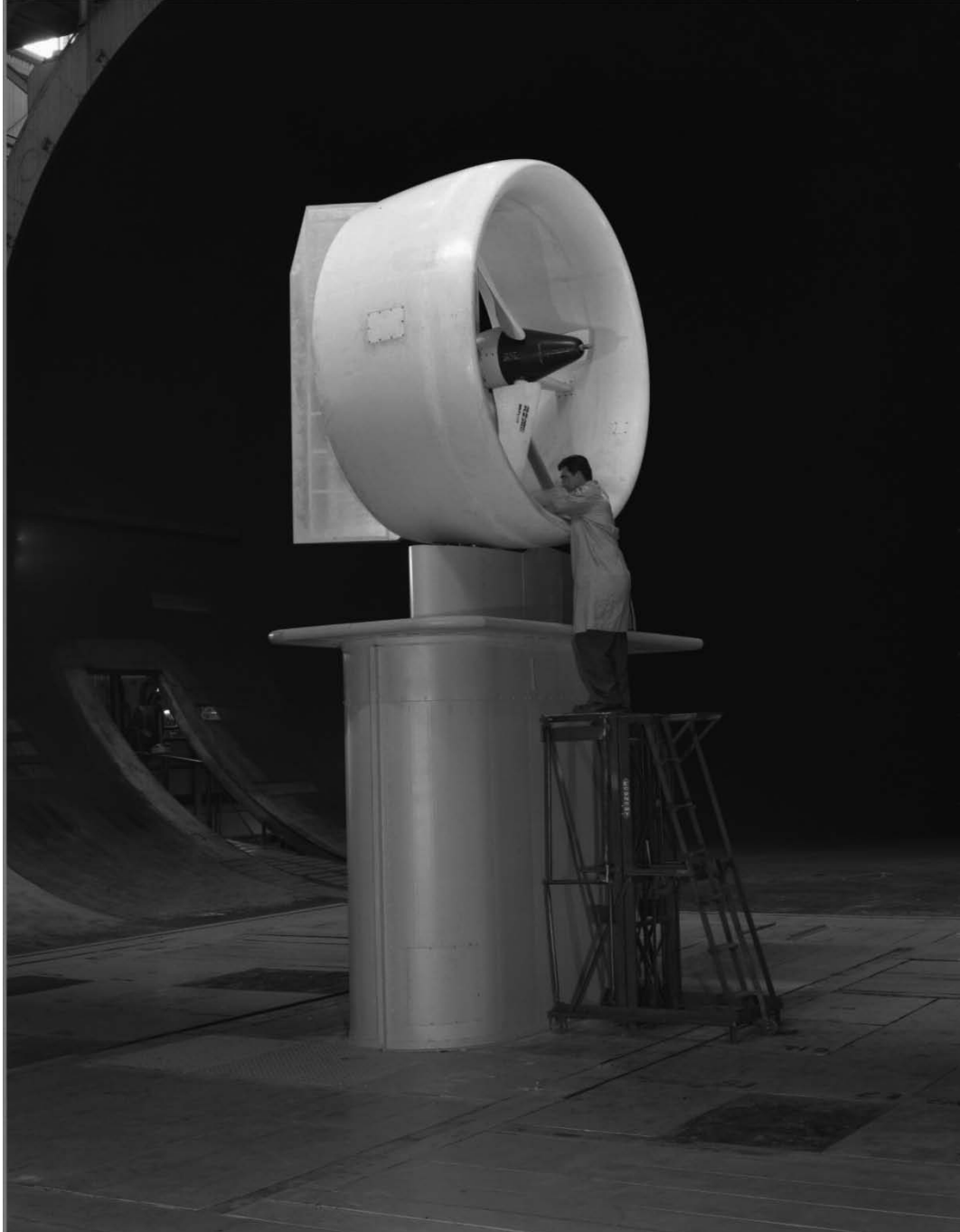
Figure 182. Bell X-22A 7-foot-diameter ducted-fan semispan model with Chuck Greco in photo checking the blade angle. (NASA A-32844)
