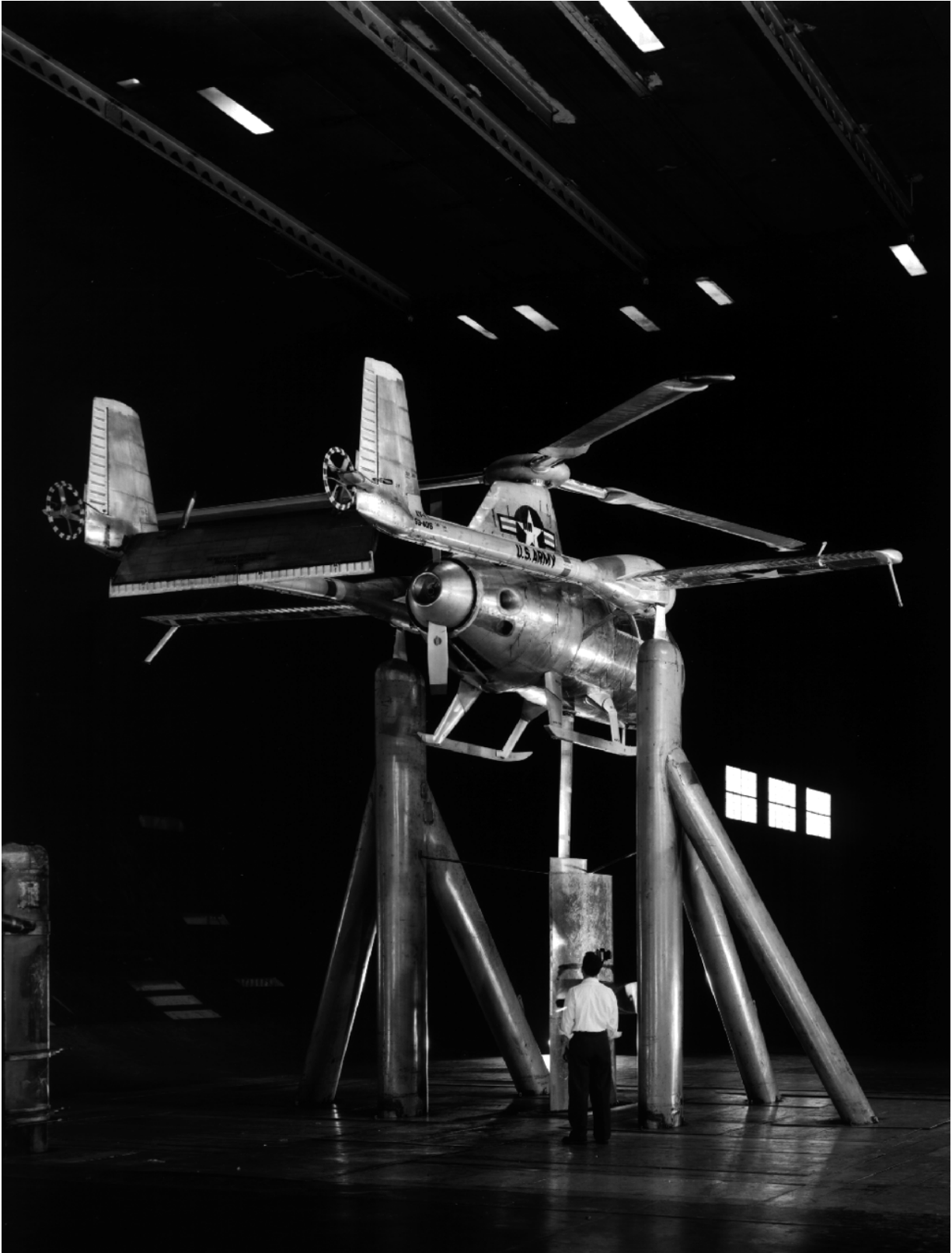
Figure 104. Three-quarter rear view of the XV-1 convertiplane. The small rotors used for yaw control at low forward speeds are shown behind the vertical tails. ( NACA A-19237 )
