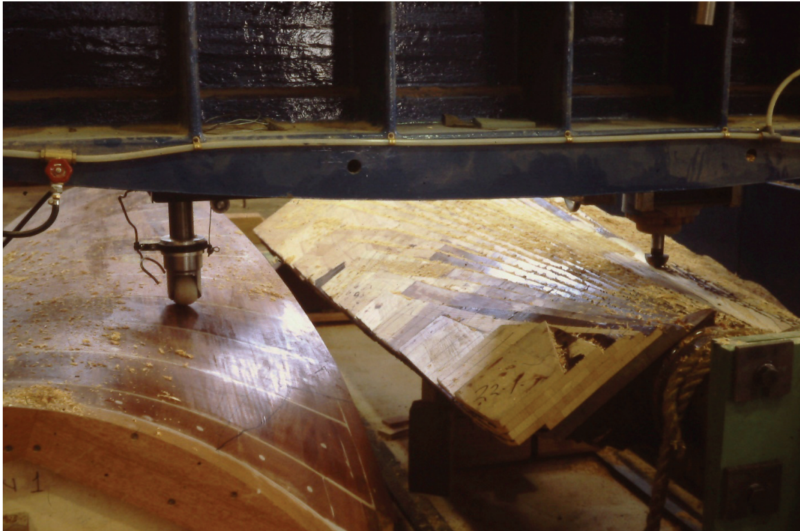
Figure 46. Fan blade shaping process showing the pattern on the left with follower and cutting router on the right. ( Author's collection, KM8 )
