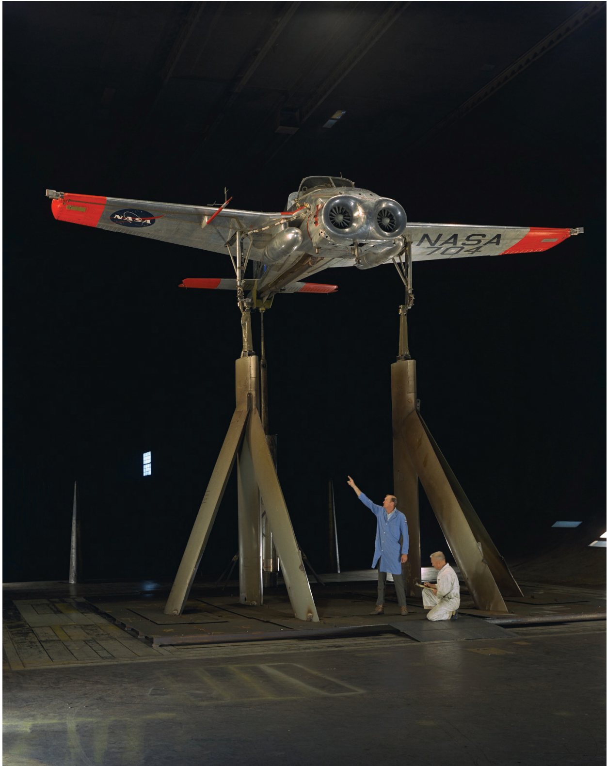
Figure 170. Bell lift-jet X-14 aircraft at zero sideslip in tunnel. (NASA A-38814)
