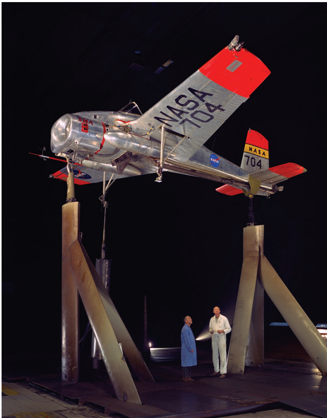
Figure 171. Bell X-14 at 90 degrees sideslip in tunnel. (NASA A-38761)
