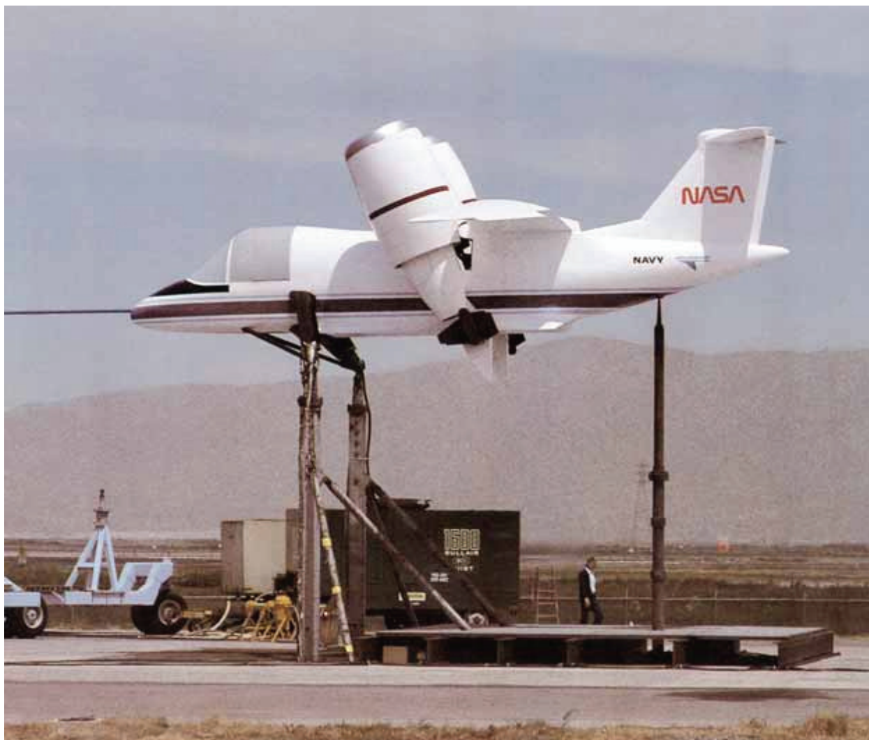
Figure 185. Grumman 698 tilt-nacelle V/STOL model with nacelles tilted upward about 60 degrees during outside static testing. ( J. Sacco collection, tilt_nacelle )
