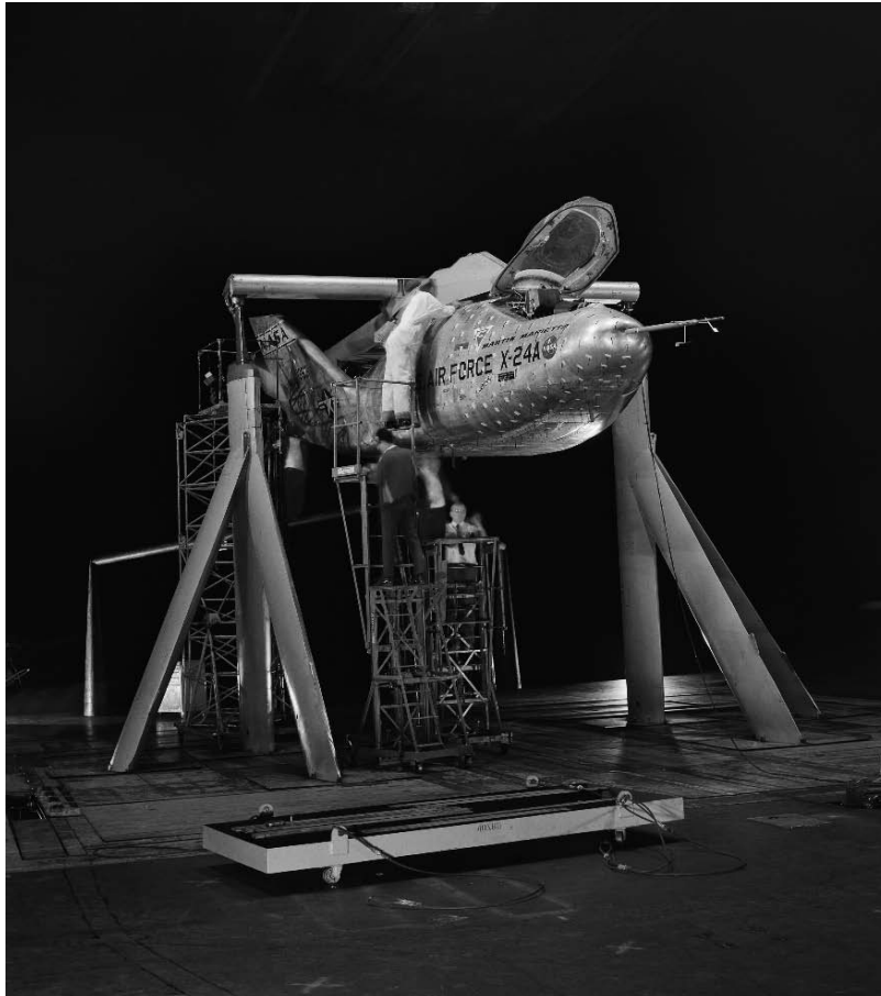
Figure 227. Martin Marietta X-24A mounted as it would be on the B-52 airplane for launching flight-tests. (NASA A-40423-009)
