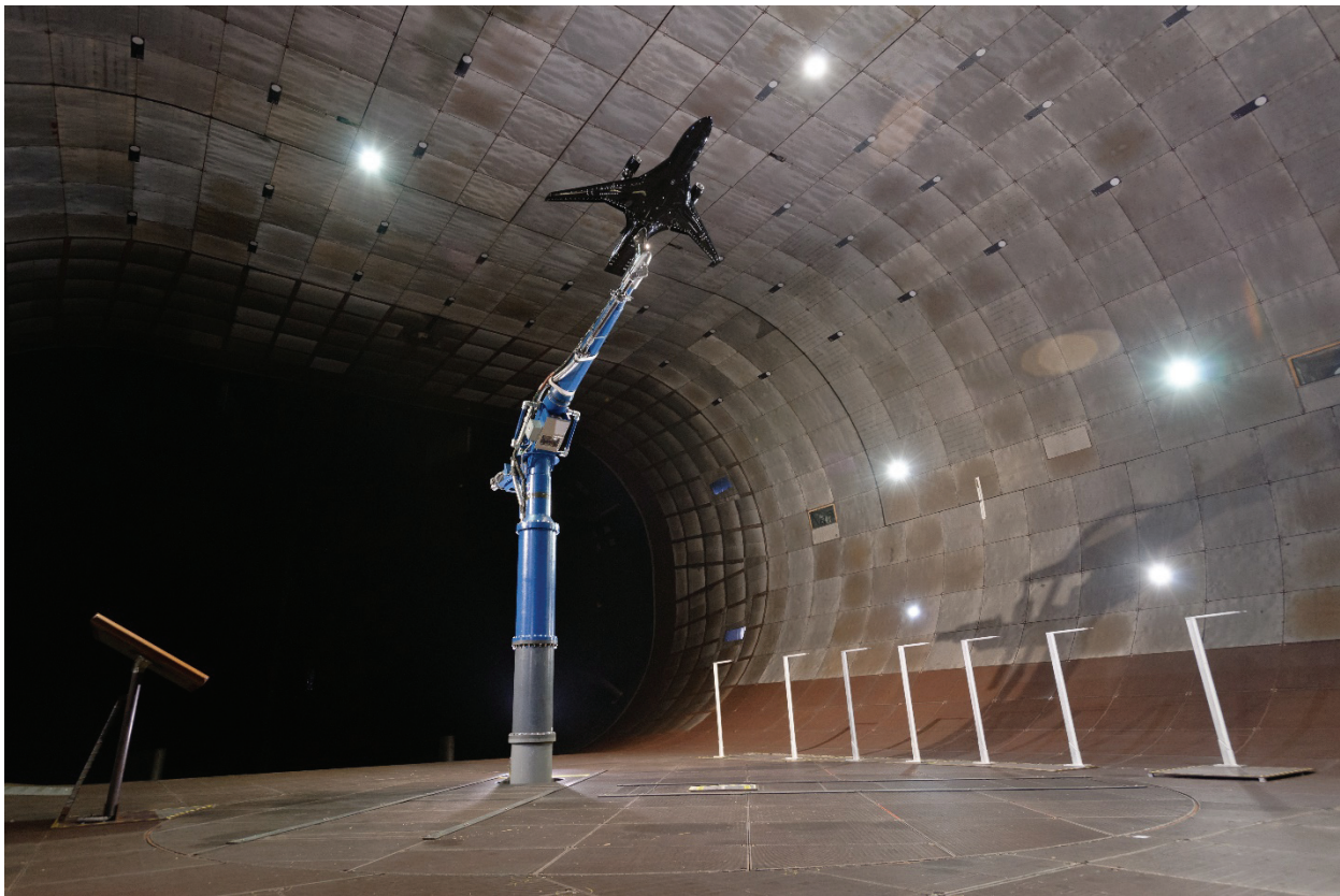
Figure 251. A 1/11-scale model of AMELIA (part of the CESTOL program) sting-mounted in the 40- by 80-foot test section. (NASA ACD12-0003-012)
