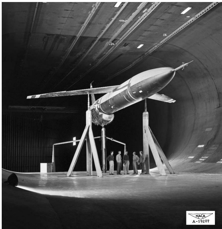
Figure 82. Northrop XB-62 cruise missile; jet-engine inlet shown at the bottom of the fuselage near the rear. (NACA A-19207)
