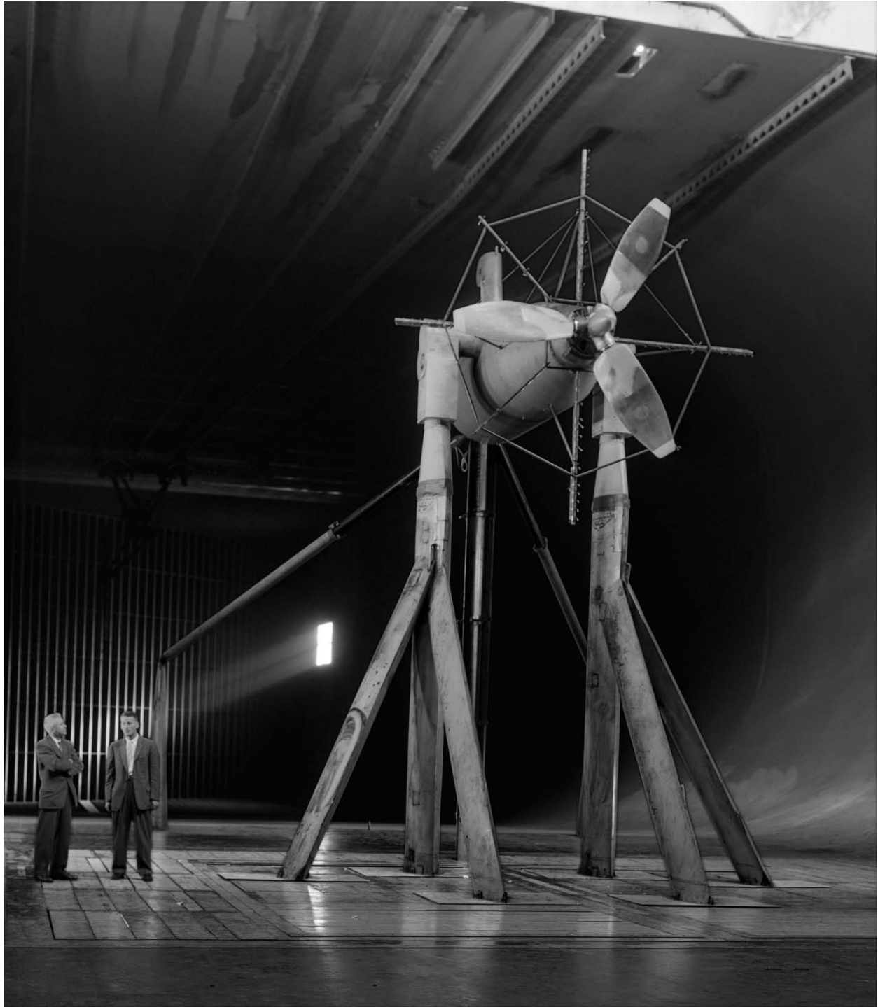
Figure 197. Downstream flow surveys of Curtiss-Wright VTOL propeller on propeller test rig at zero degree angle of attack. Note the wide-chord blades. ( NASA A-24304 )
