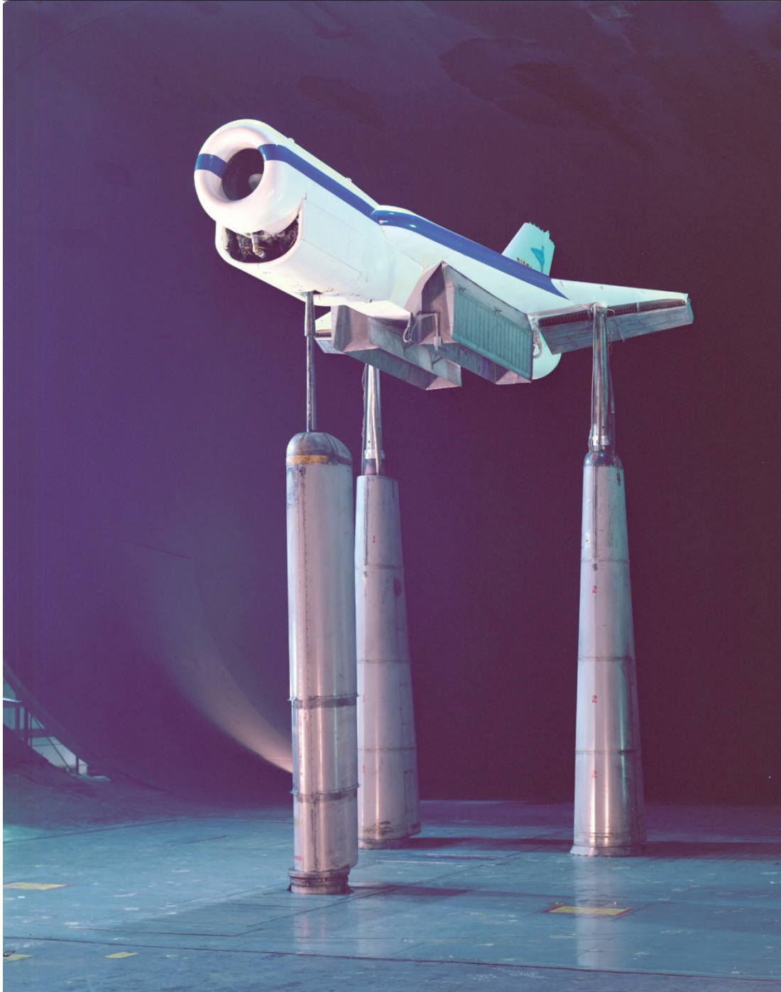
Figure 210. Three-quarter front view of augmentor model with ejectors at the wing root. (NASA AC79-0197-1)
