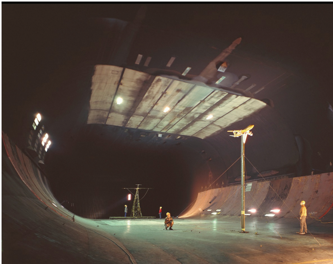
Figure 118. Vortex-wake testing with a 747 model as a wake generator. ( NASA AC74-2201 )
