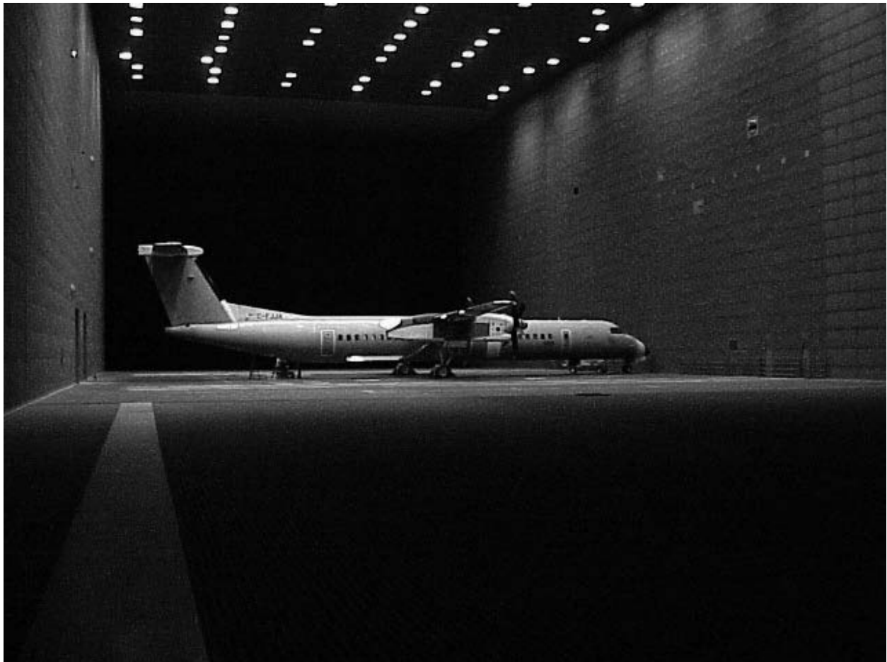
Figure 267. Bombardier Dash 8 Q400 aircraft in the 80- by 120-foot test section; this was the largest airplane ever tested in a wind tunnel. ( J. Sacco collection, airliner_80x120 )
