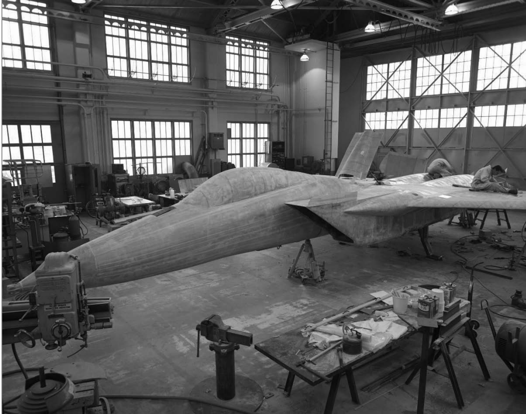
Figure 111. A 3/4-scale model of the McDonnell Douglas F-15 Eagle fighter undergoing construction in the Ames model shop. (NASA AC71-5717)
