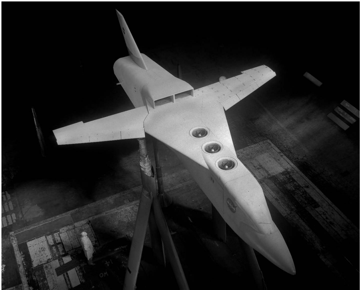
Figure 168. Overhead view of lift-engine model with three engines in fuselage. (NASA A-38524)
