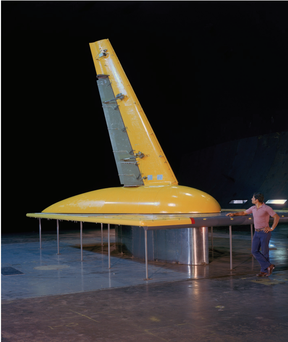
Figure 207. Three-quarter front view of semispan augmentor wing and fuselage model with John Bouldt in photo. (NASA AC75-2276)
