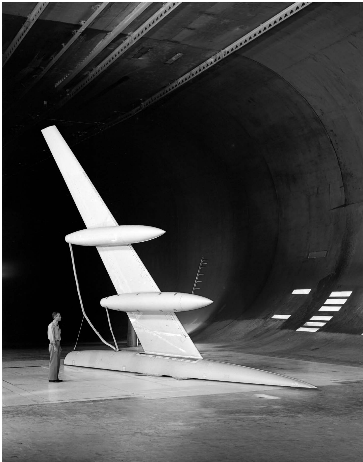
Figure 101. Semispan swept-wing model used for flow surveys at propeller locations. Engineer Vern Rogallo in photo. ( NACA A-16397.1 )
