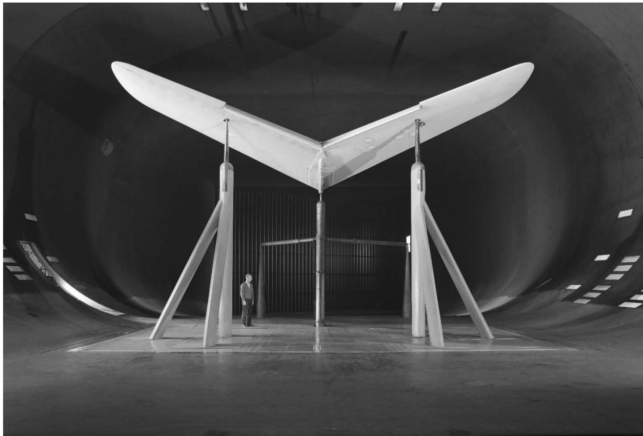
Figure 83. Wing model used for swept-wing studies; wings are swept forward. ( NACA A-12509 )
