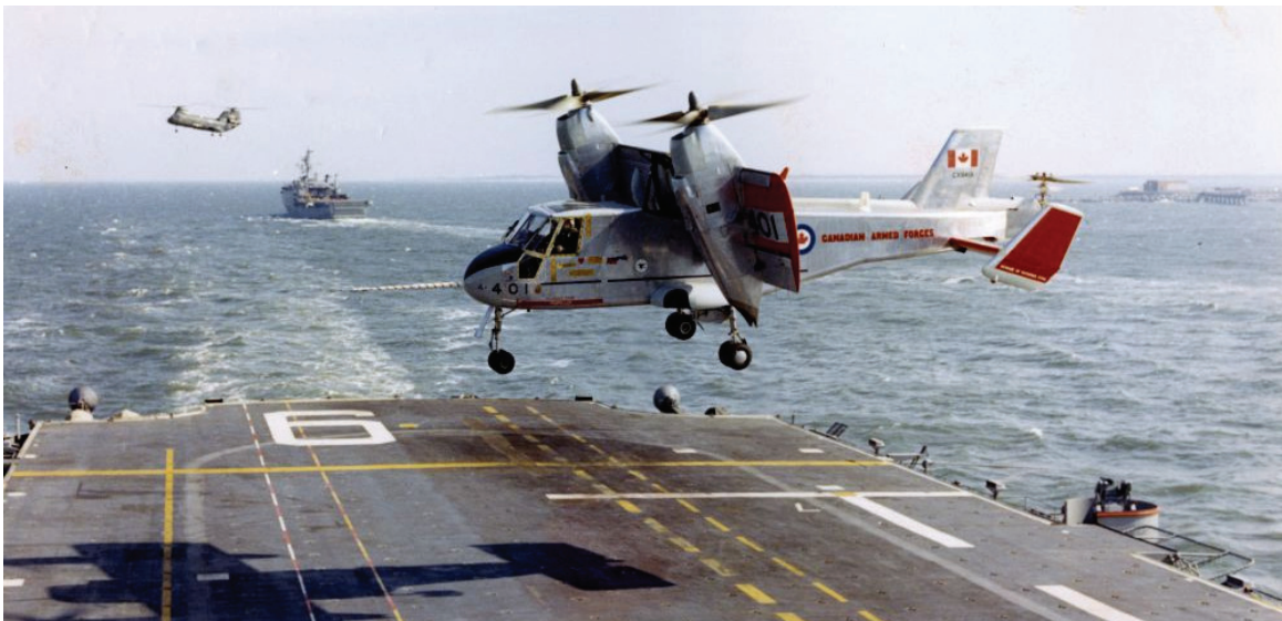
Fig. 2-86. The Canadair CL-84. This 10,600-pound VTOL technology demonstrator made its first hovering flight on May 7, 1965. The first full conversion back and forth from hover was made on January 17, 1968. The CL-84's success far exceeded either Vertol's VZ-2 or Hiller's X-18.
