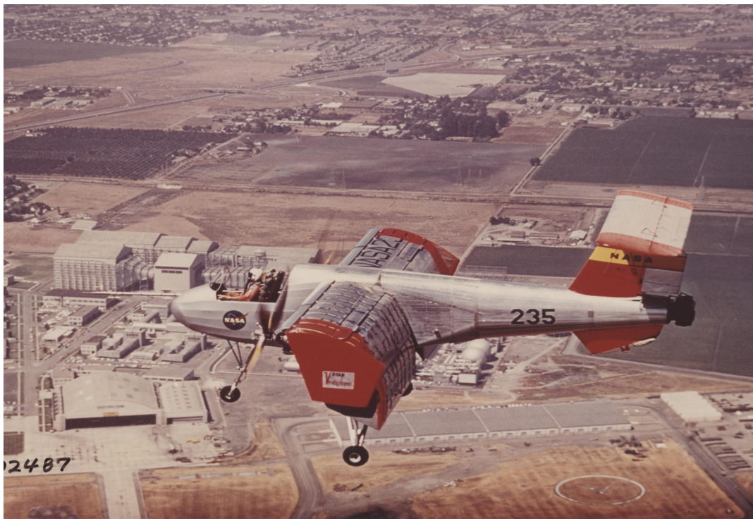
Fig. 3-95. The Ryan VZ-3, along with several NASA wind tunnel experiments, established what potential the deflected slipstream concept had for VTOL. The wingspan was 23 feet and the gross weight was about 2,600 pounds. The general conclusion was that the approach was not too promising, and now the aircraft is on display at the U.S. Army Aviation Museum in Ft. Rucker, Alabama.
