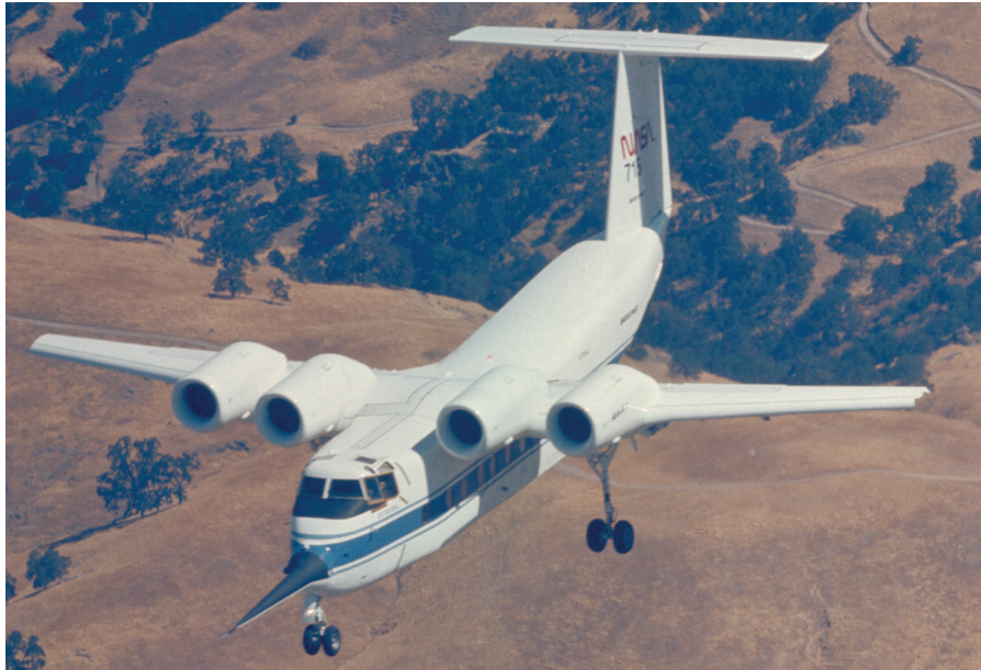
Fig. 3-196. NASA's QSR, a Boeing conversion of a de Havilland Buffalo, first flew July 6, 1978. Operational weight empty was 36,800 pounds; normal takeoff weight was 50,000 pounds. Wingspan was 73.5 feet with an area of 600 square feet. Each Avco YF102 turbofan engine was rated at 7,500 pounds thrust [641-646].
