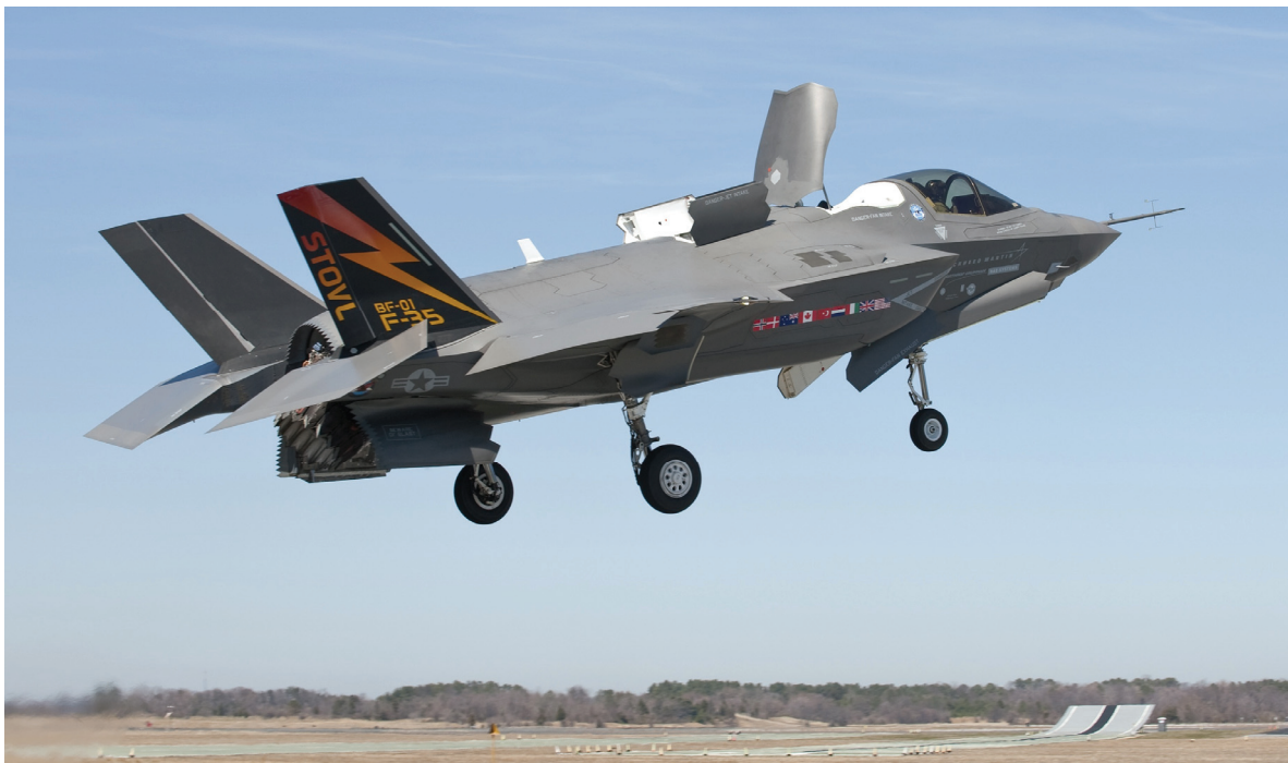
Fig. 1-30. The Joint Strike Fighter, the F-35, is a slightly compromised V/STOL called a STOVL, which stands for Short Takeoff and Vertical Landing. The approach defines the mission takeoff gross weight based on a STOL takeoff rather than a vertical takeoff. After fuel is burned off, a vertical landing and takeoff is easily accomplished.
