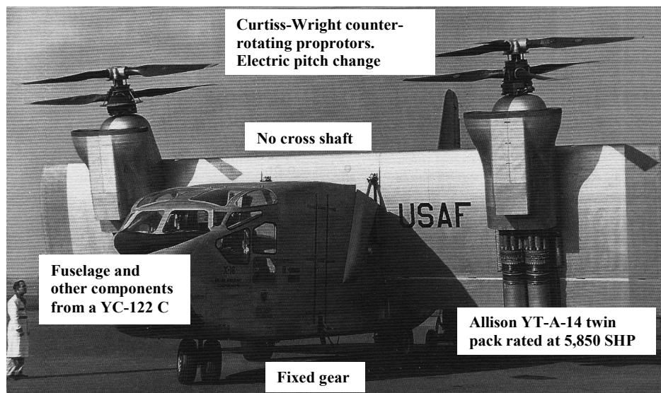
Fig. 2-81. The Hiller X-18 tiltwing 33,000-pound experimental aircraft first flew on November 24, 1959. It had so many prop rotor, engine, and other design problems that the U.S. Air Force cancelled the program on January 18, 1964.
