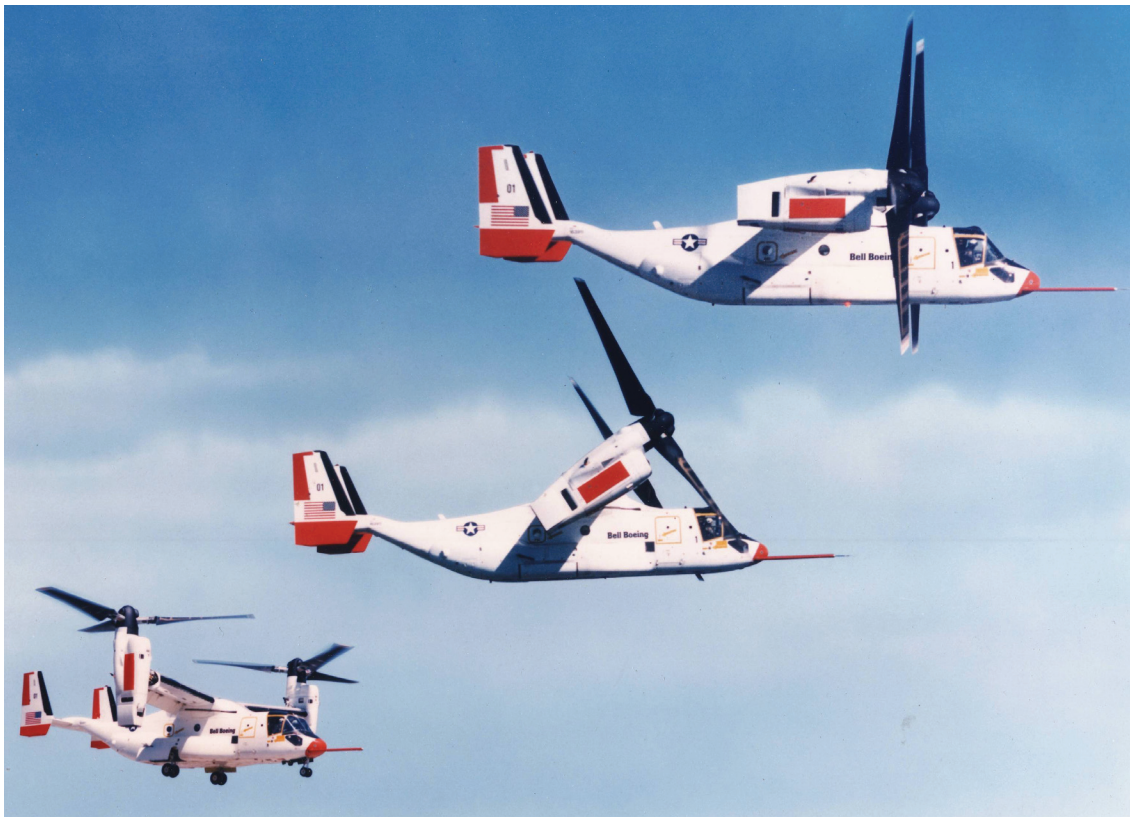
Fig. 2-63. The Bell/Boeing V-22 Osprey: a collage showing the aircraft in hover, then in transition with the rotors partially tilted, and finally in cruise flight.
