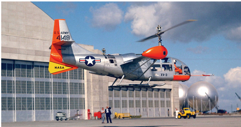
Fig. 2-126. The XV-3 (s/n 54-4148), the second aircraft, used Bell's "standard" two-bladed, teetering propeller, which, along with several other fixes, suppressed whirl flutter enough that military flight test evaluation could be completed [256].
