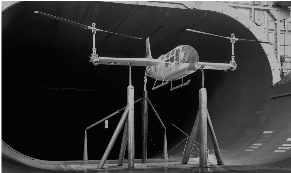
Fig. 2-133. Before flight testing at Edwards Air Force Base, the XV-3 was tested in NASA's large-scale wind tunnel (photo courtesy of Bill Warmbrodt).
