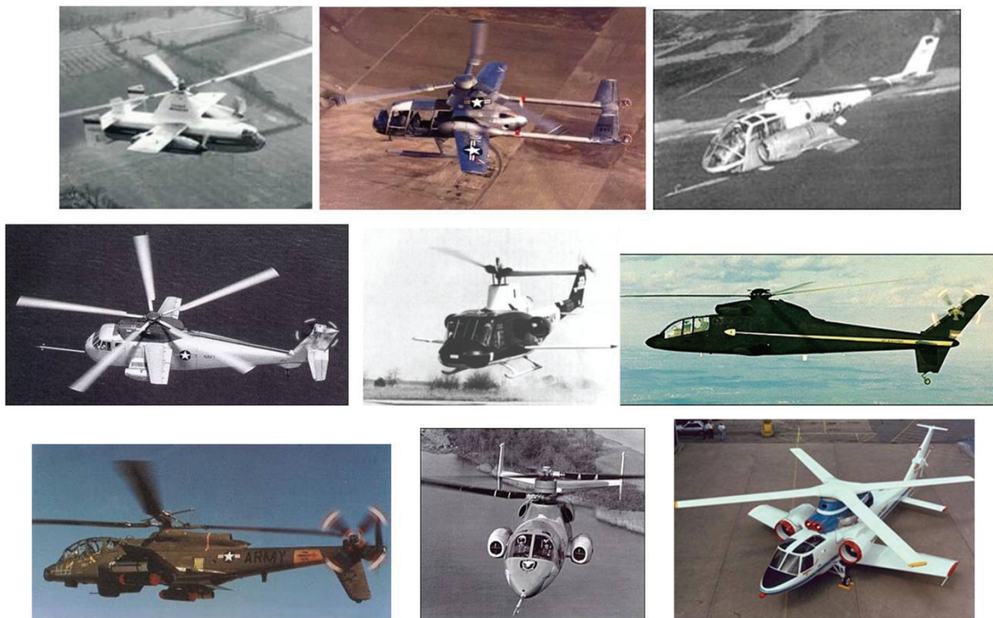
Fig. 2-44. Some past high-speed rotary wing aircraft (1950s through 1970s). Top row—Fairey Rotodyne, McDonnell XV-1, and Lockheed XH-51; center row—Sikorsky NH-3, Bell 533, and Sikorsky S-67; bottom row—Lockheed AH-56, Sikorsky S-69 Advancing Blade Concept, and Sikorsky/NASA/DARPA Rotor Systems Research Aircraft (RSRA) with a prototype x-wing installed (photos courtesy of Todd Quackenbush).
