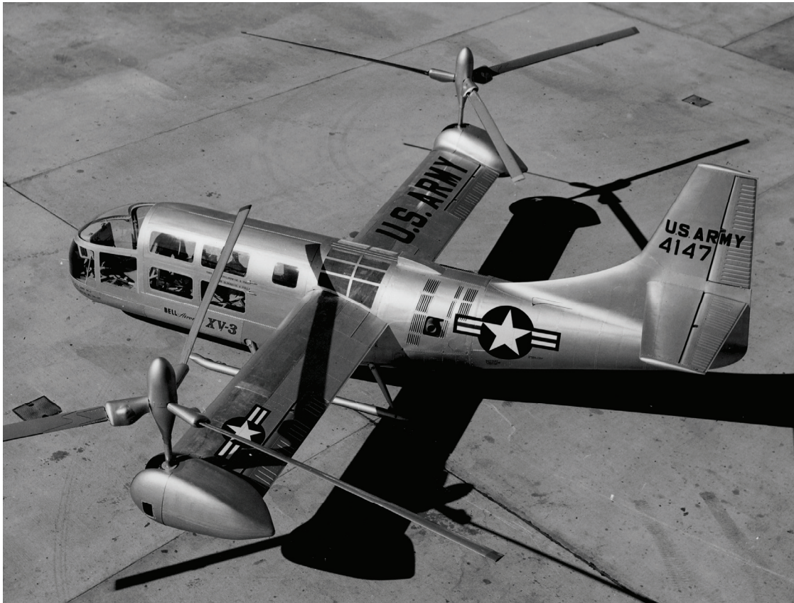
Fig. 2-125. The Bell XV-3 (s/n 54-4147) started out with three-bladed, articulated hinged propellers. A dynamic instability referred to as rotor-pylon instability, and later as whirl flutter, finally caused a catastrophic crash on October 25, 1956 (photo courtesy of Tommy Thomason).
