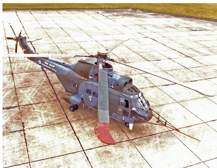
Figure 44. Research Puma with swept-tip blades at RAE Bedford.
